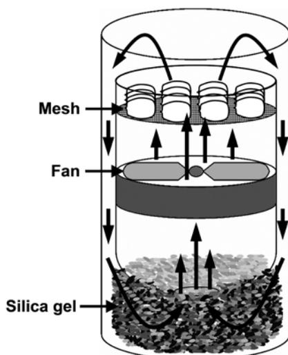
**Fig. 3** Schematic diagram of the apparatus used in this study to achieve rapid desiccation. Arrows show the movement of air when seeds placed on the mesh ( $n = 9-16$ ) were desiccated. Silica gel was packed under the main component and was recharged in an oven before each use.
