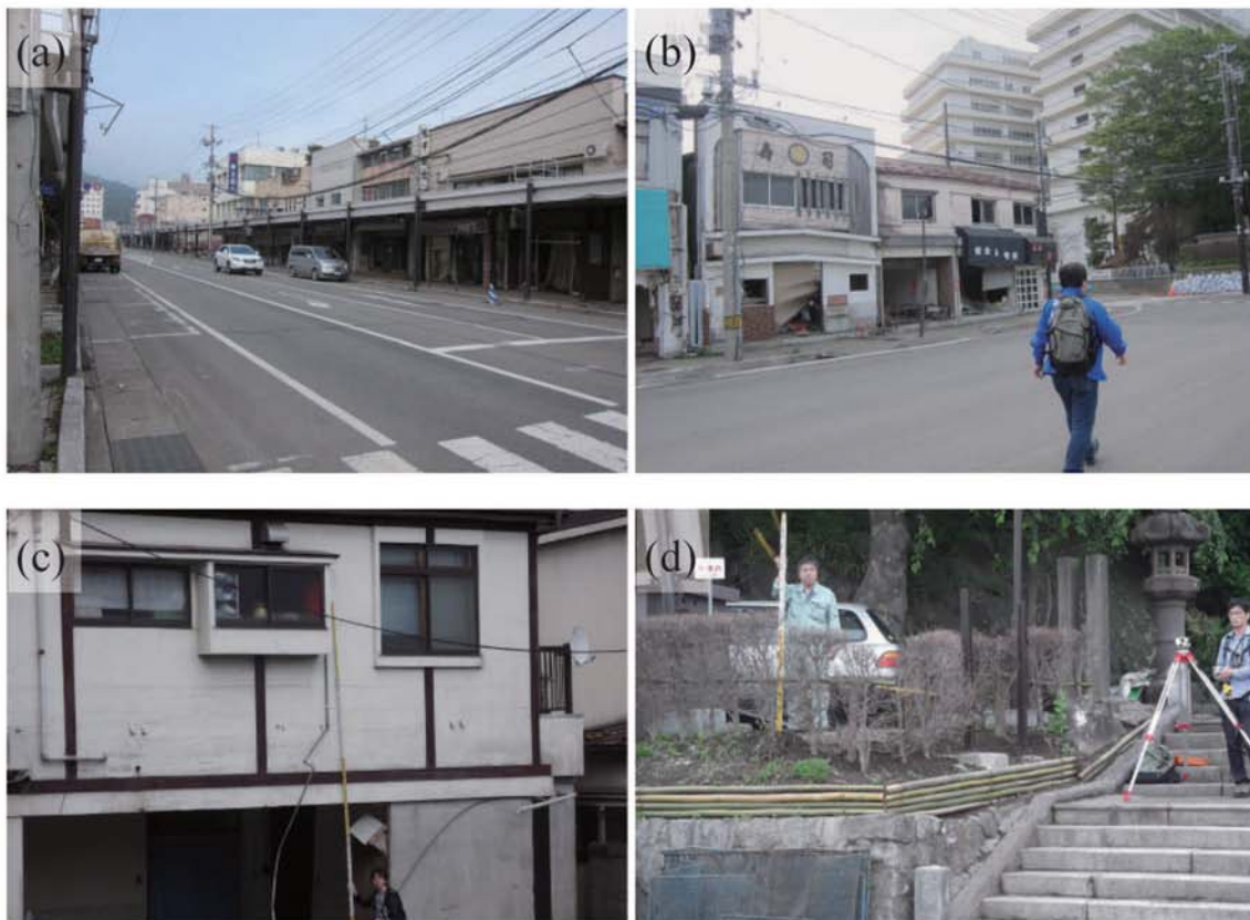
Fig. A120. (a)-(b) Damage at Omachi. (c) Watermark on the wall of the Japanese green tea shop Sachu (3.95 m above ground level, I123). (d) Benchmark (TP 4.0m), which is under the rod used to measure tsunami height.
