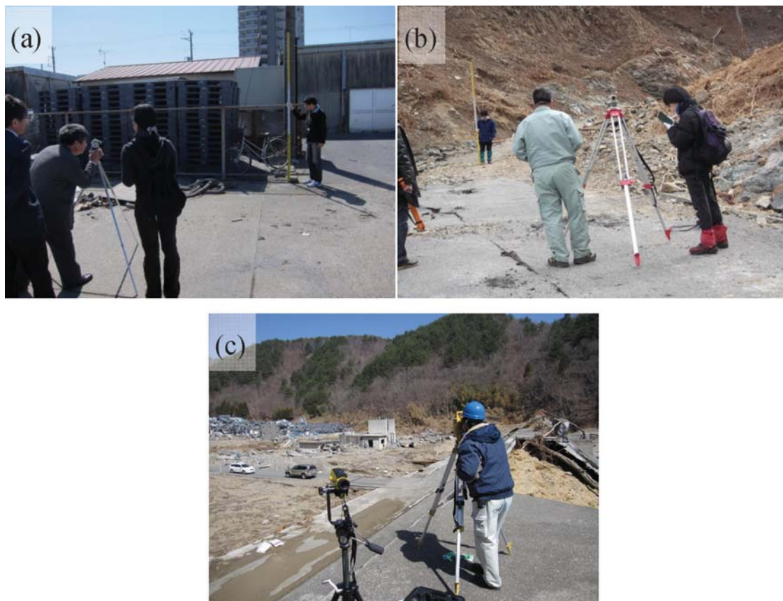
Fig. 2. Instruments used in the survey: (a) level tracon (b) auto-level (c) total-station (right) and laser range finder “Tru Pulse 360” (left).
