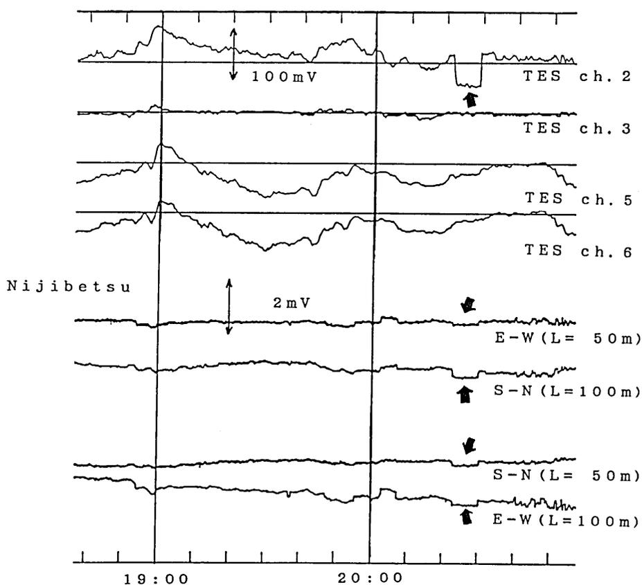
Fig. 17. Example of anomalous disturbances detected simultaneously both on ch. 2 of Teshikaga and on all the short-span dipoles set up at Nijibetsu Junior High School (indicated by arrows). L is the span of each short dipole. E-W means that we measure the potential difference of the eastern electrode minus the western one.
