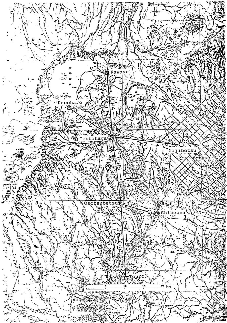
Fig. 5. Distribution of NTT electrodes at telephone stations and measuring channels at Teshikaga (TES).
