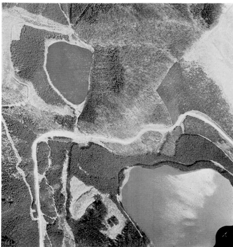
Fig. 36. Large-scale slide on embankment and damage to slope protection at Point B in the Fig. 5.
