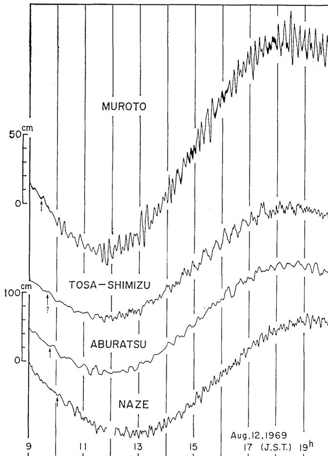
Fig. 13. Tide gauge records of tsunami.
