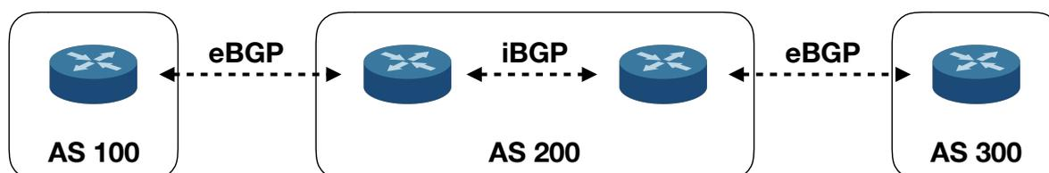
Fig. 2.1. Routers in different ASs communicate using eBGP or iBGP.
