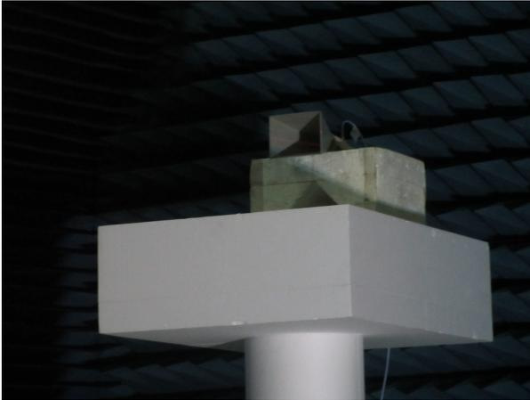
(b) Standard X-band horn antenna for calibration
