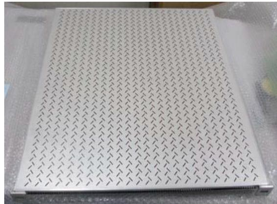
(d) Fabricated antenna panel. The radiating slot-pair can be seen cut on the front aluminum skin.
