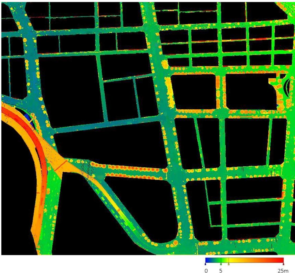
**Figure 4-2.** Generated high-resolution ground elevation profile from ALS.
