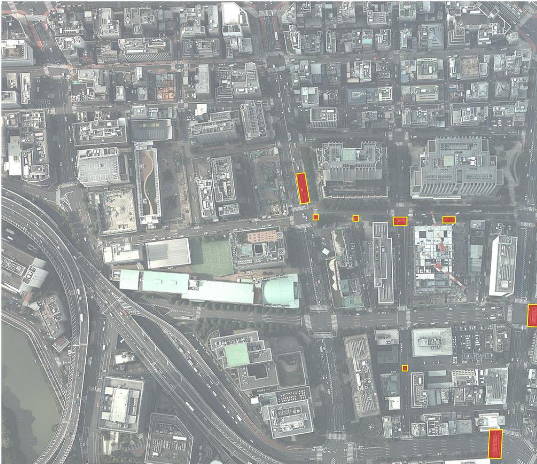
**Figure 3-32.** Areas where the road markings were repainted after June 12, 2014 (the date of the aerial image acquisition).
