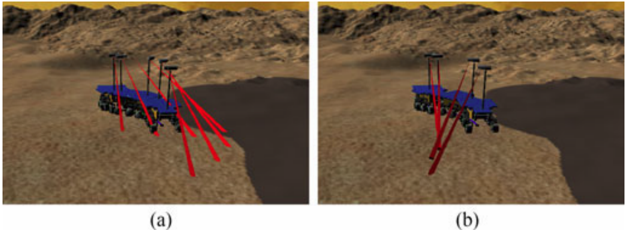
図 1.4: The red lines represent the viewing directions of mast cameras. In (a), the mast angles and timing are predefined. In (b), the optimal viewing angles and timing are computed based on the VOSAP(proposed) algorithm[14].
