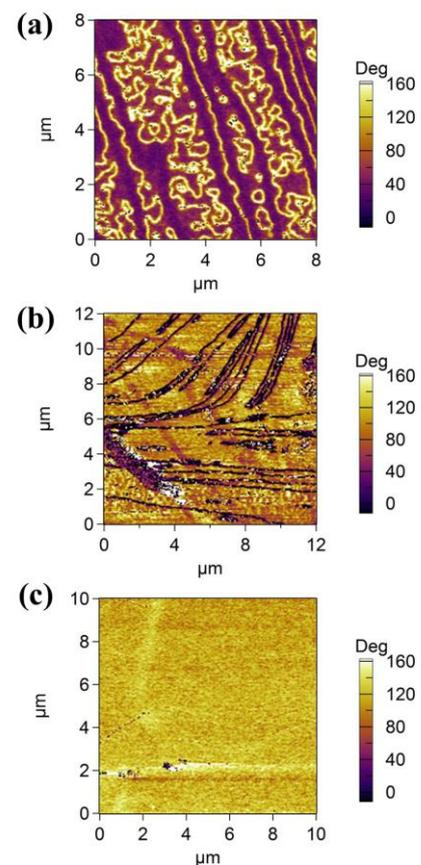
**Fig.3:** Phase of piezoresponse signal of LSFO. Color contrast corresponds to ferroelectric domain. (a)LSFO grown at  $1250^\circ\text{C}$  (b) LSFO grown below  $1250^\circ\text{C}$  (c) LSFO grown at  $1200^\circ\text{C}$
