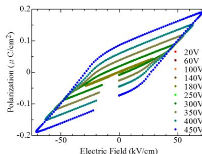
**Fig. 4** : Hysteresis loop of polarization of LSFO at 2 K.
