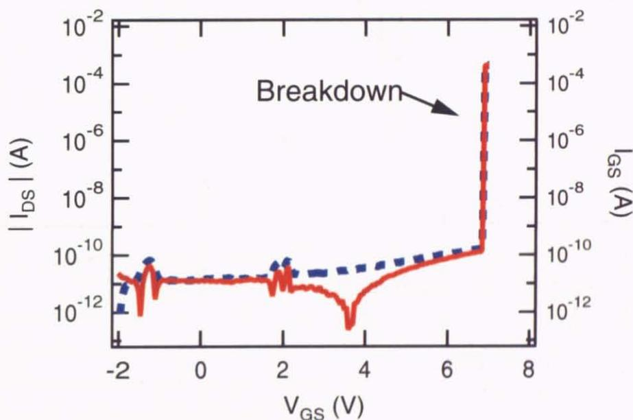
Figure 57:  $I_{DS}$  vs.  $V_{GS}$  at 100 K. This FET did not show channel current change before gate insulator breakdown at  $V_{GS} \approx 7$  V at 100 K.
