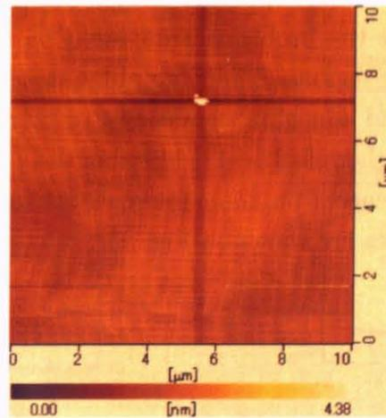
Figure 63: AFM image of the surface of an epitaxial DSO/STO/LTO/STO structure. The size of the image is  $10\ \mu\text{m} \times 10\ \mu\text{m}$ .
