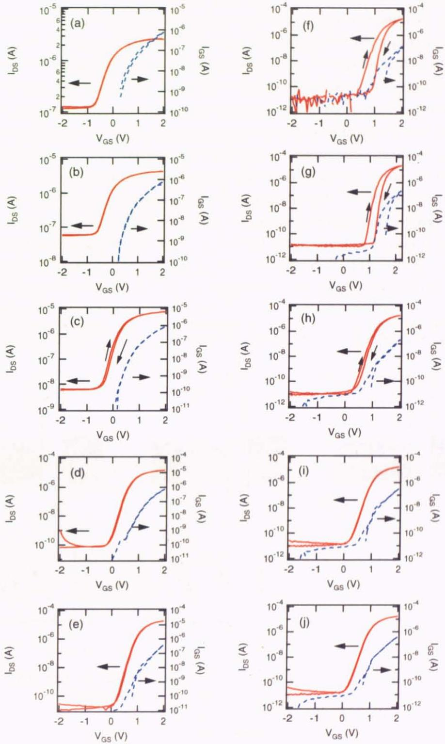
Figure 65:  $I_{DS}$  and  $I_{GS}$  as a function of  $V_{GS}$ , measured at (a) 250, (b) 200, (c) 150, (d) 100, (e) 75, (f) 60, (g) 50, (h) 40, (i) 30, and (j) 17 K.
