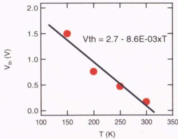
Figure 56: Linear fit of  $V_{\text{th}}$  vs. temperature.
