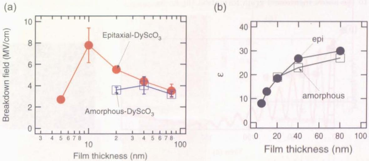
Figure 43: (a) Average breakdown fields of epitaxial and amorphous DSO films. (b) Thickness dependence of dielectric constant of epitaxial and amorphous DSO films.
