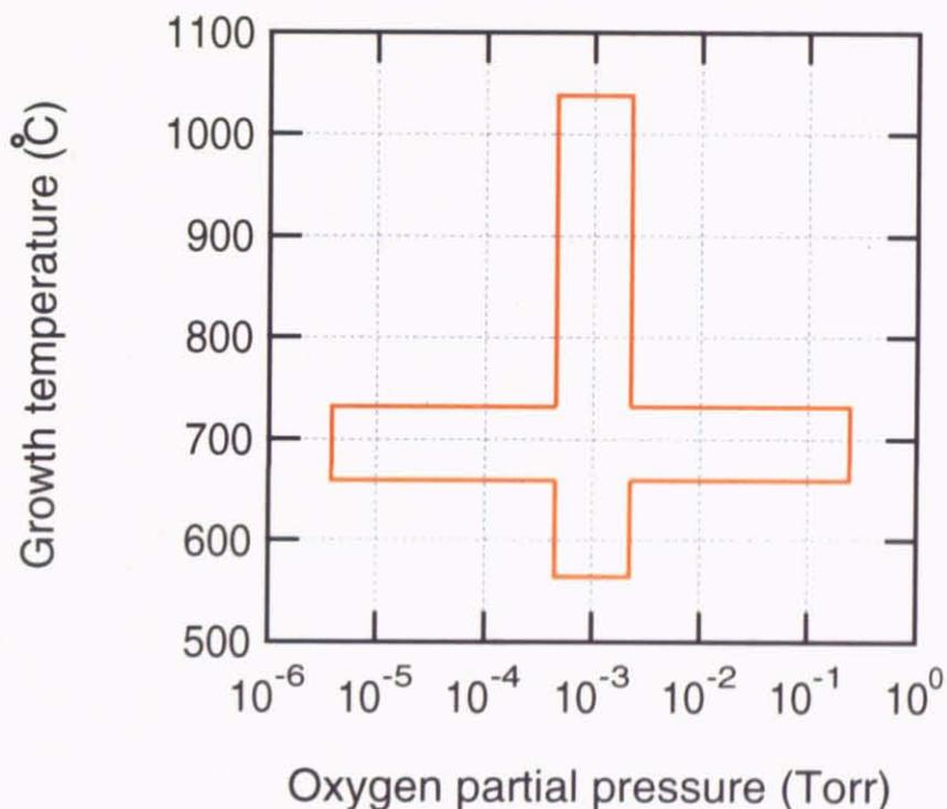
Figure 27: DSO films were fabricated at from 600 to 1000 °C, 1 mTorr, and from 10<sup>-5</sup> to 10<sup>-1</sup> Torr, 700°C.
