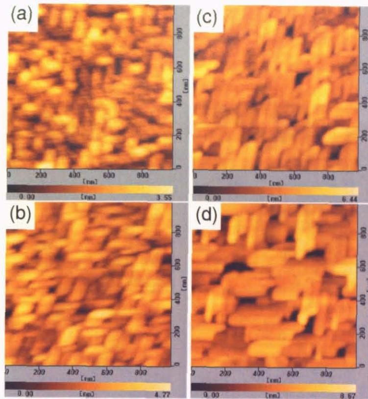
Figure 21: AFM image of NGO film surface grown at (a)700 °C, (b)800 °C, (c)900 °C, (d)1000 °C. These AFM images size are 1  $\mu\text{m}$   $\times$  1  $\mu\text{m}$ .
