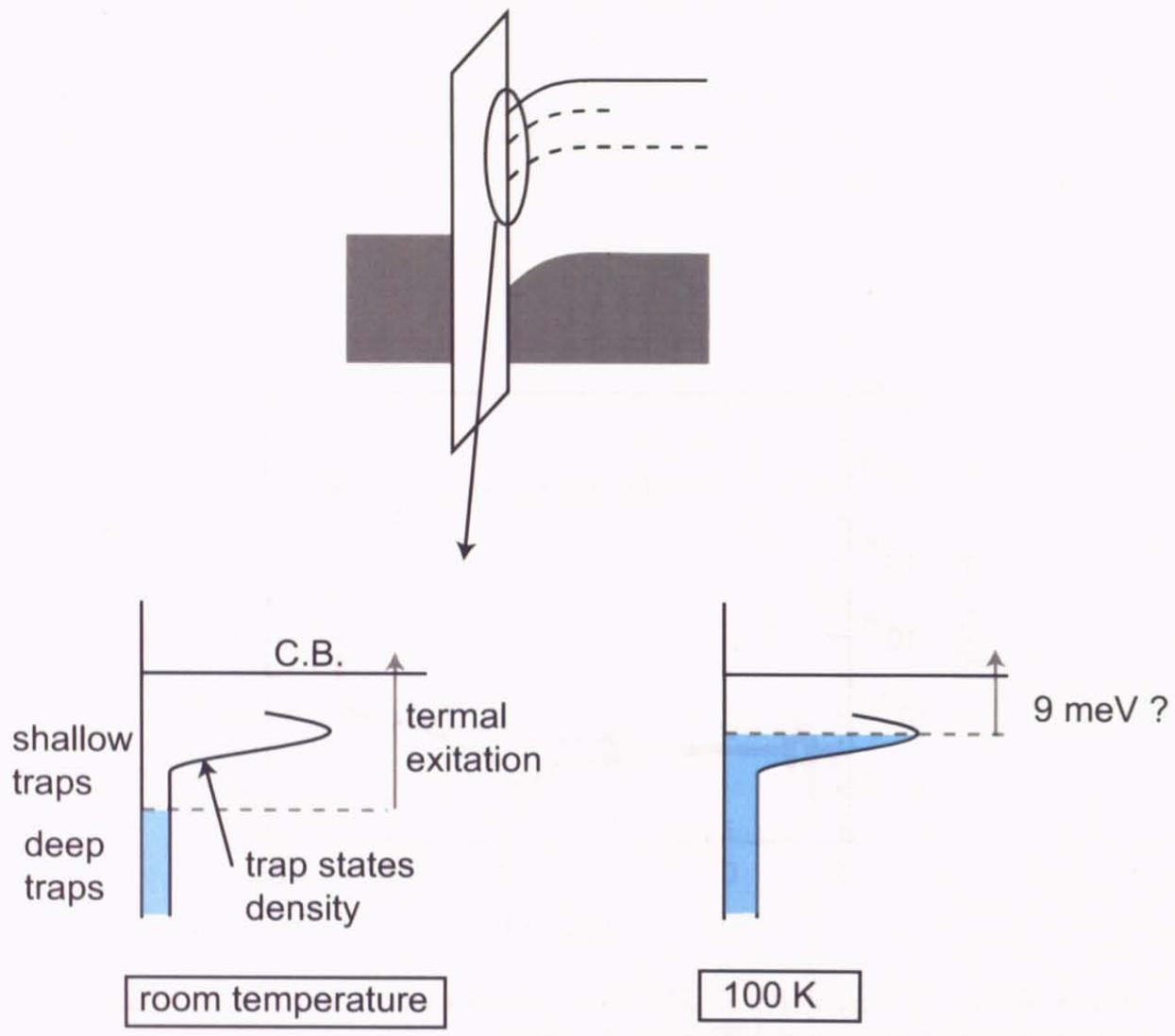
Figure 58: Schematic drawing of electronic states close to the conduction band bottom in the interface region of the amorphous CHO/STO heterostructure.
