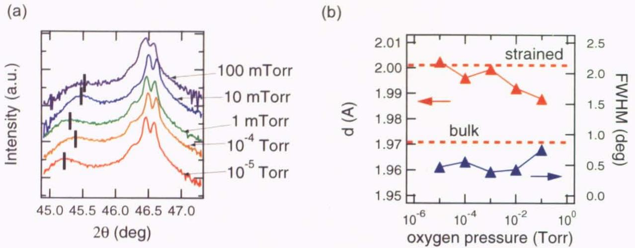
Figure 33: (a) XRD  $2\theta$ - $\theta$  scan around STO(200) peak is shown. (b) The out-of-plane axis length change and FWHM at each oxygen pressure.
