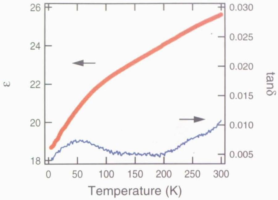
Figure 38: Temperature dependence of dielectric constant of 80 nm DSO film on Nb:STO.
