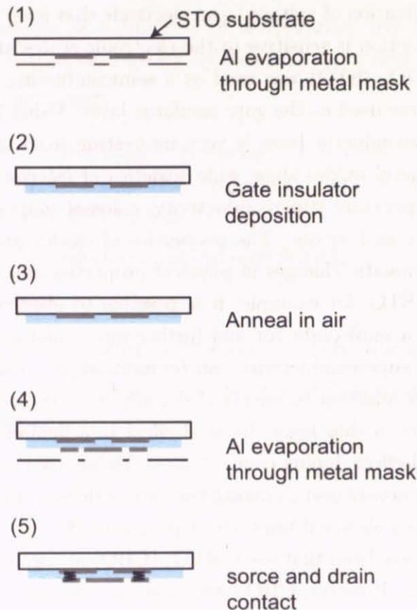
Figure 49: Fabrication process of amorphous DSO/STO FETs
