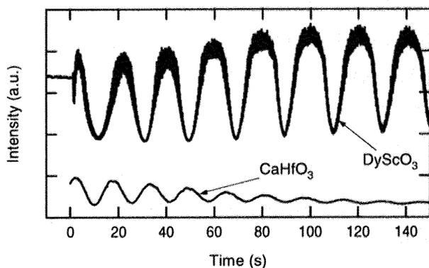
Figure 47: Typical RHEED oscillation of epitaxial DSO and CHO film on Nb:STO substrate.
