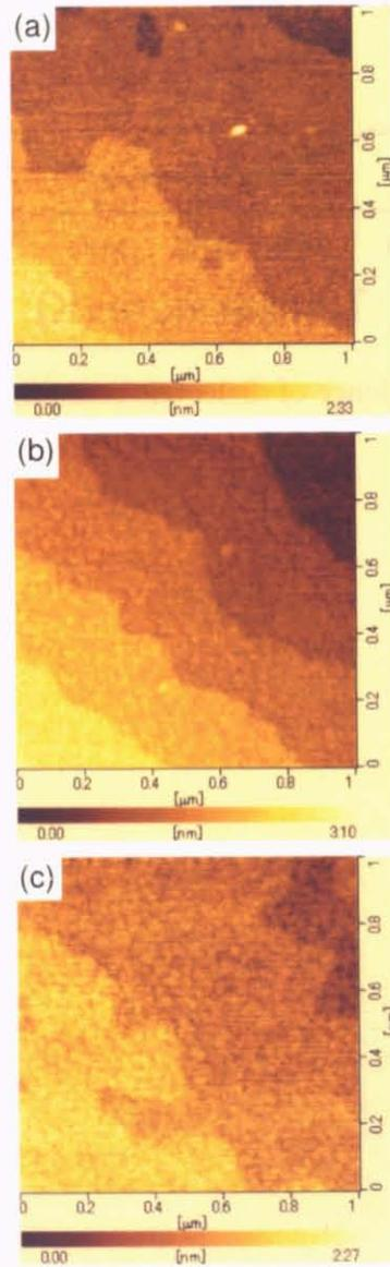
Figure 39: AFM images of amorphous DSO films with thickness,(a) 20, (b) 40, (c) 80 nm. The size of these AFM images were  $1\mu\text{m} \times \mu\text{m}$ .
