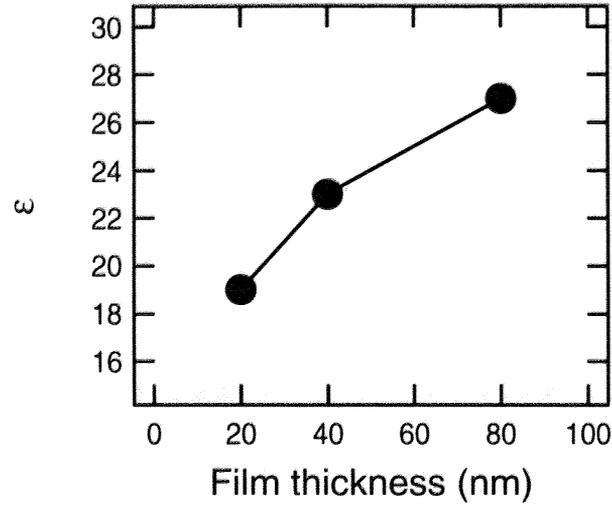
Figure 41: Dielectric constant of various thickness amorphous DSO films on Nb:STO.
