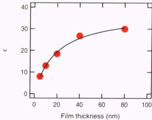
Figure 37: Thickness dependence of dielectric constant of epitaxial DSO film of Nb:STO. Solid line is fitting curve of thickness dependent dielectric constant.
