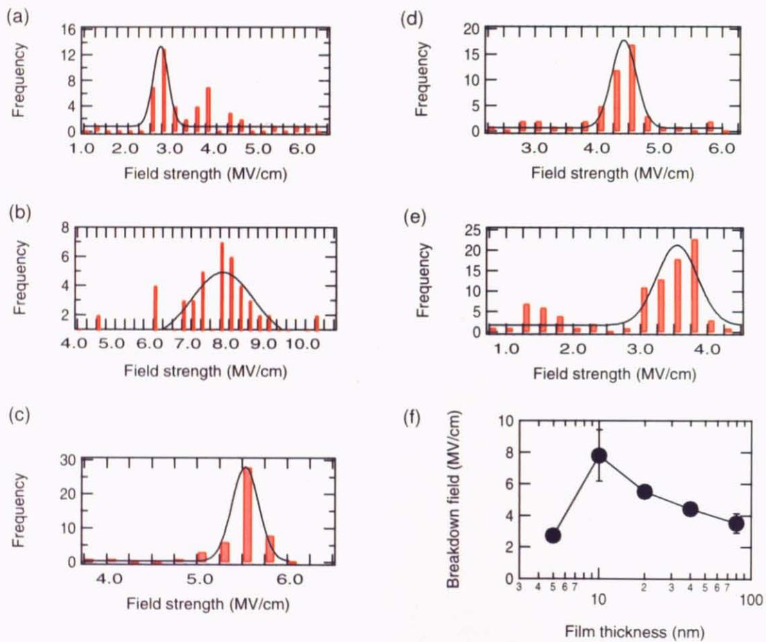
Figure 35: The histogram of breakdown field of epitaxial DSO film with the thickness, (a) 5, (b) 10, (c) 20, (d) 40, and (e) 80 nm. (f) Thickness dependence of average breakdown field at each thickness. These AFM images size are  $1 \mu\text{m} \times 1 \mu\text{m}$ , and the values of RMS of surface morphology were calculated using  $1 \mu\text{m} \times 1 \mu\text{m}$  images.
