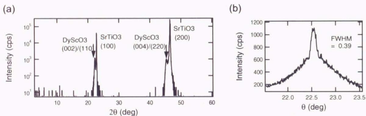
Figure 29: (a) XRD  $2\theta$ - $\theta$  scan and, (b) rocking curve of DSO film grown at 700 °C, 1 mTorr.
