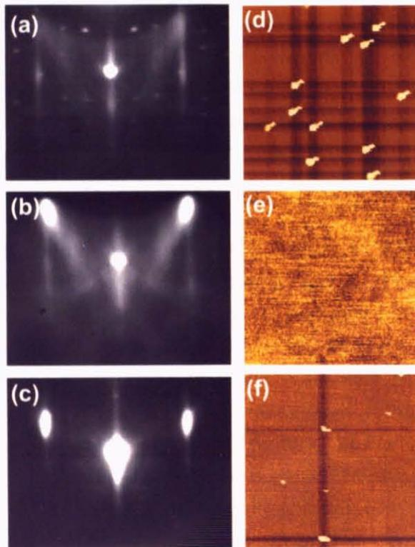
Figure 62: RHEED patterns and AFM images of annealed amorphous LTO film surfaces: (a), (d) 4 unit cells, (b), (e) 3 unit cells, and (c), (f) amorphous STO (4 u.c.) / LTO (5 u.c.) multi-layer surface. The AFM image sizes are  $10 \mu\text{m} \times 10 \mu\text{m}$ .
