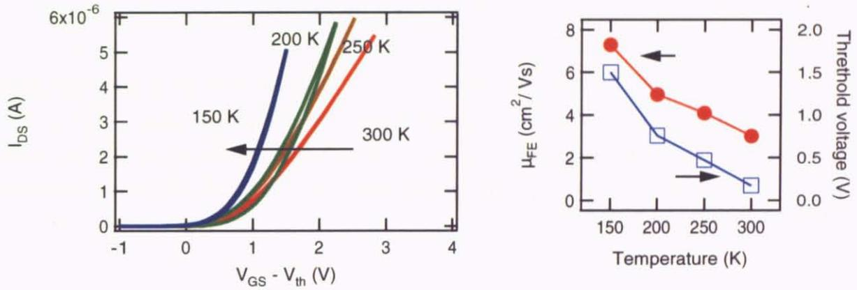
Figure 55: (a)  $I_{DS}$  vs.  $I_{th}$  at 300, 250, 200, and 150 K. (b) Field-effect mobility (open squares) and threshold voltage (filled circles) shift as a function of temperature.
