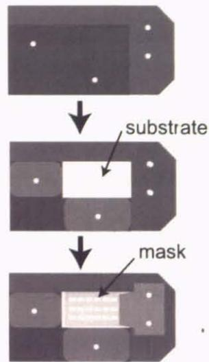
Figure 50: Schematic view of the sample holder that was used to fix the metal mask and STO substrate. First, the STO substrate was fixed in place with two metal brackets. After that, a metal mask was placed on the substrate and fixed with a clamp. The corner of the sample holder was used as a position reference.
