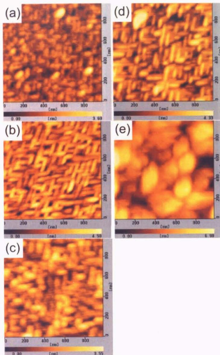
Figure 22: AFM image of NGO film surface grown at (a) $10^{-5}$ , (b) $10^{-4}$ , (c) $10^{-3}$ , (d) $10^{-2}$ , (e) $10^{-1}$  Torr oxygen partial pressure. These AFM images size are  $1 \mu\text{m} \times 1 \mu\text{m}$ .
