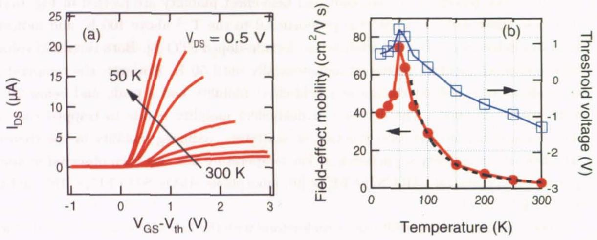
Figure 67: Temperature dependence of (a)  $I_{DS}-(V_{GS} - V_{th})$  curve and (b) field-effect mobility (filled circle) and threshold voltage (open square) as a function of temperature. The dashed line shows a  $T^{-2}$  fit of the field-effect mobility.
