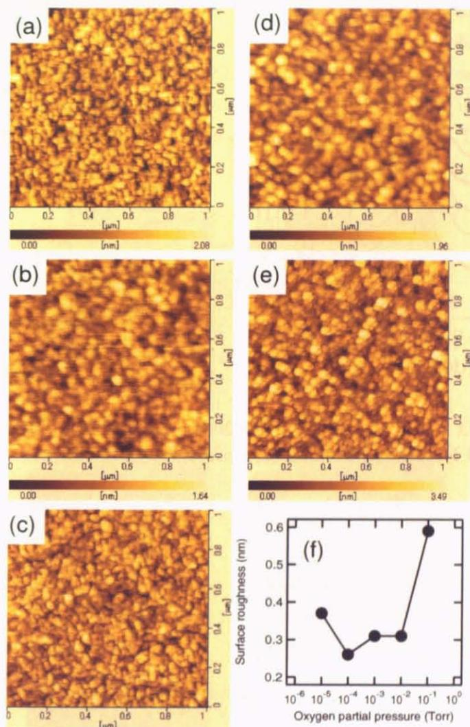
Figure 32: AFM image of growth oxygen pressure, (a)  $10^{-5}$ , (b)  $10^{-4}$ , (c)  $10^{-3}$ , (d)  $10^{-2}$ , and (e)  $10^{-1}$  Torr. (f) RMS of surface roughness at each oxygen pressure. These AFM images size are  $1\ \mu\text{m} \times 1\ \mu\text{m}$ , and the values of RMS of surface morphology were calculated using  $1\ \mu\text{m} \times 1\ \mu\text{m}$  images.
