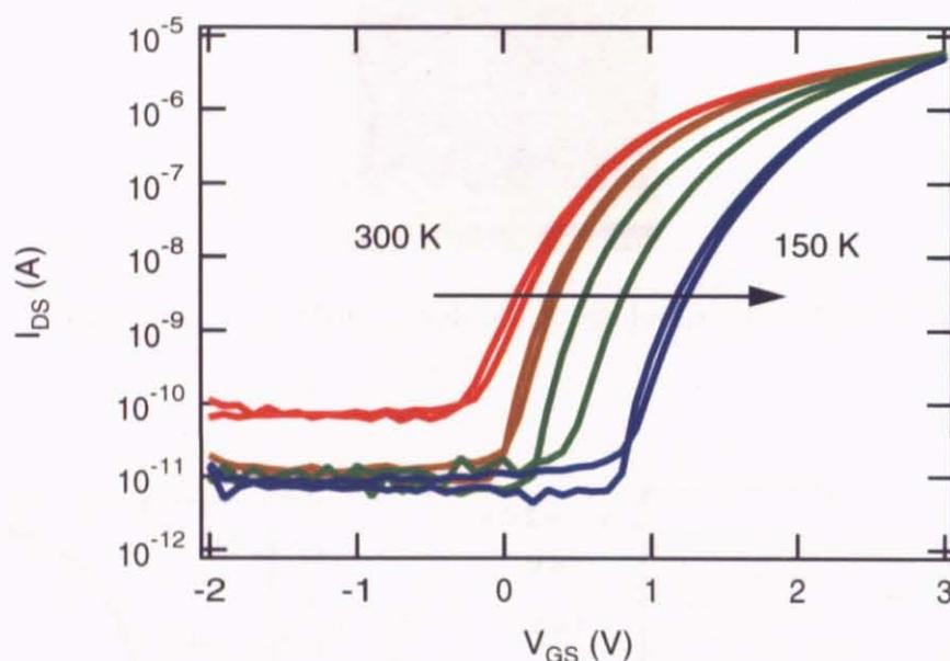
Figure 54:  $I_{DS}$  vs.  $V_{GS}$  at 300, 250, 200, and 150 K.
