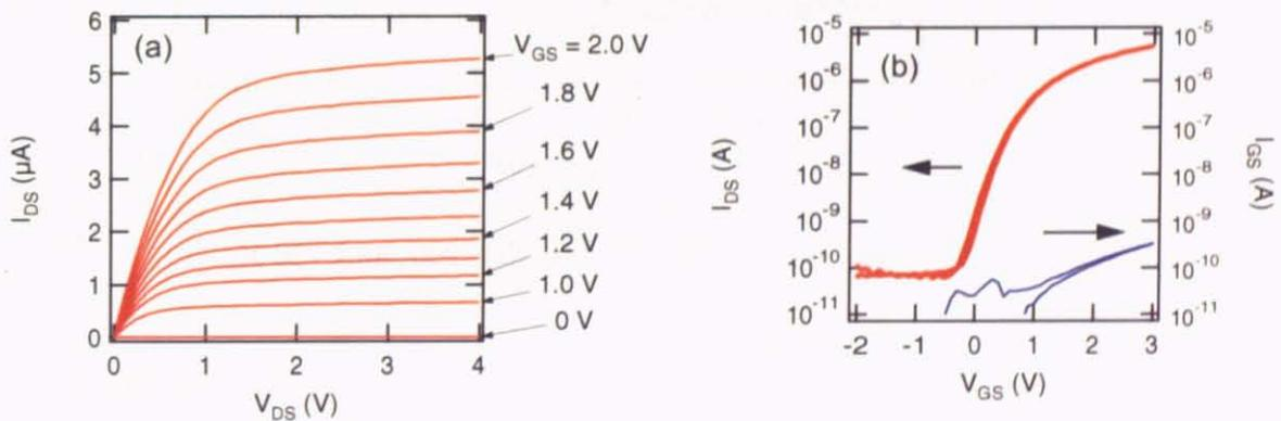
Figure 53: (a) Drain-source current,  $I_{DS}$ , plotted as a function of the drain-source bias,  $V_{DS}$ , (b) Drain-source current and the gate leak current,  $I_{GS}$ , plotted as a function of the gate bias at a fixed drain-source bias  $V_{DS}$  of  $+0.5 \text{ V}$ . The field-effect mobility was  $3.0 \text{ cm}^2/\text{V s}$  and the on-off ratio was higher than  $10^4$ .
