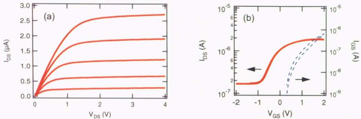
Figure 64: (a)  $I_{DS}$  vs.  $V_{DS}$  at  $V_{GS}$  of 0, 0.25, 0.5, 0.75, and 1 V. (b)  $I_{DS}$  and  $I_{GS}$  as a function of  $V_{GS}$ .  $V_{DS} = 0.5$  V. Both measurements were done at room temperature.
