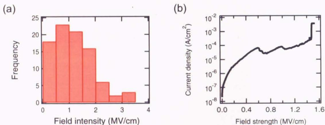
Figure 24: (a)The histogram of breakdown field of 5 nm thick NGO film grown at 700 °C, 1 mTorr. The average breakdown field was 1.6 MV/cm. (b)A typical example of breakdown characteristic of NGO film.
