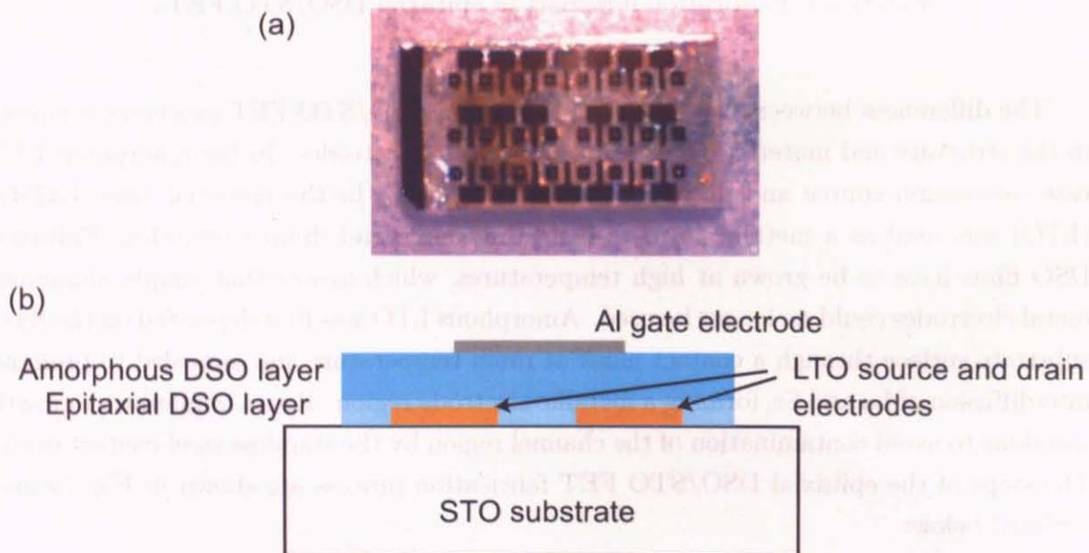
Figure 60: (a) Photograph and (b) schematic view of the epitaxial DSO/STO FET.
