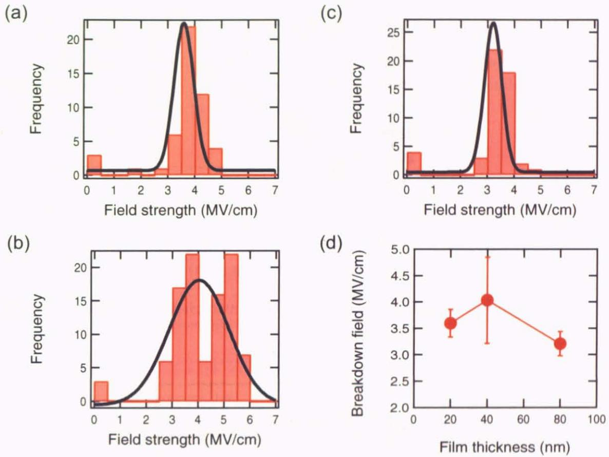
Figure 40: Histograms of breakdown fields of (a) 20, (b) 40, and (c) 80 nm thick amorphous DSO film on Nb:STO.
