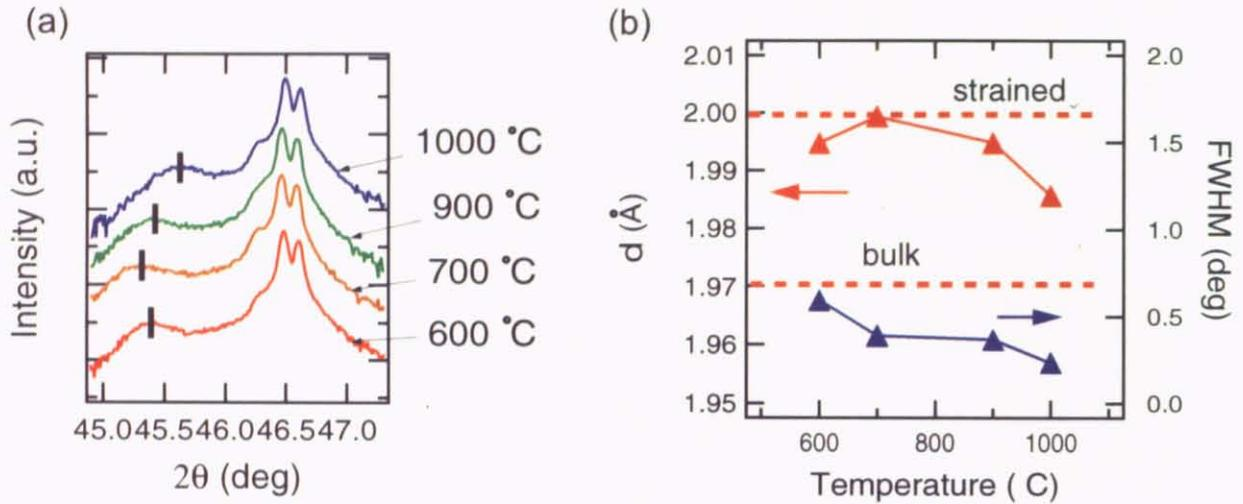
Figure 31: (a) Growth temperature dependence of XRD  $2\theta$ - $\theta$  scan of DSO/STO at around STO (200) peak and (b) out-of-plane axis length of, and FWHM of rocking curve DSO film (220)/(004) peak of 1 mTorr oxygen partial pressure during film growth.
