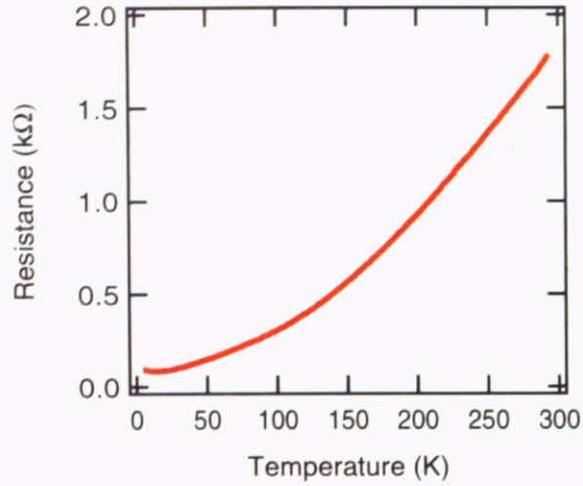
Figure 61: The temperature dependence of resistance of an annealed STO(4 u.c.) / LTO(5 u.c.) / STO heterostructure.
