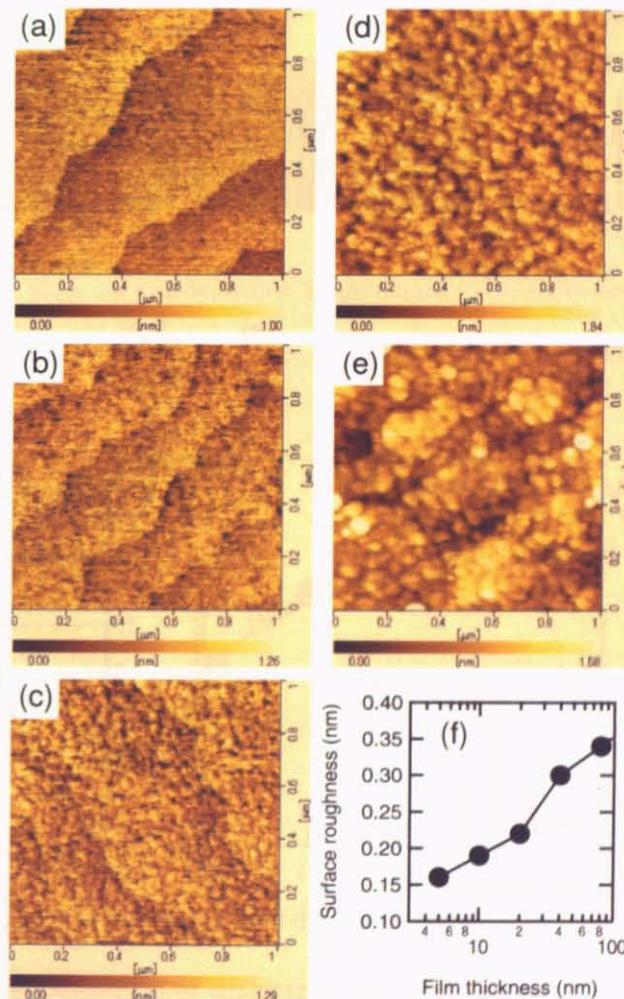
Figure 34: AFM image of DSO film on Nb:STO with various thickness, (a) 5, (b) 10, (c) 20, (d) 40, and (e) 80nm . (f) thickness dependence of RMS of DSO film surface roughness.
