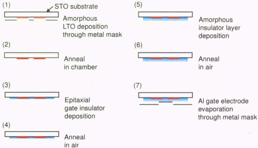
Figure 59: Fabrication flowchart of epitaxial DSO/STO FETs.
