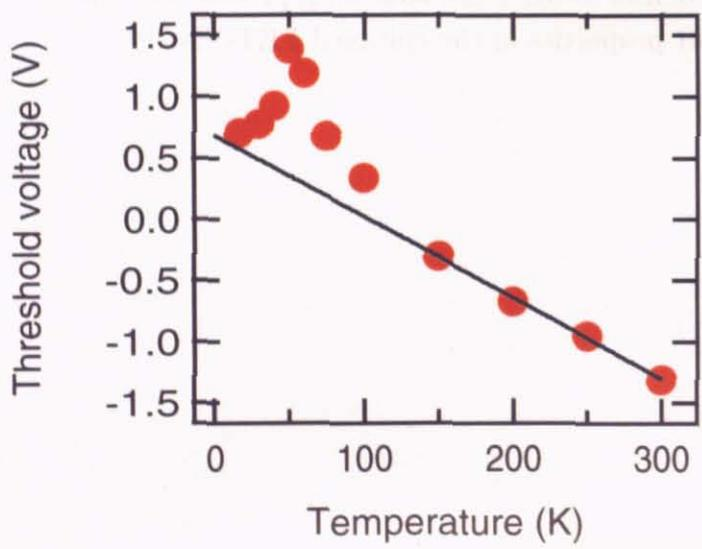
Figure 68: Linear fit (above 150 K) of  $V_{th}$  vs. temperature.
