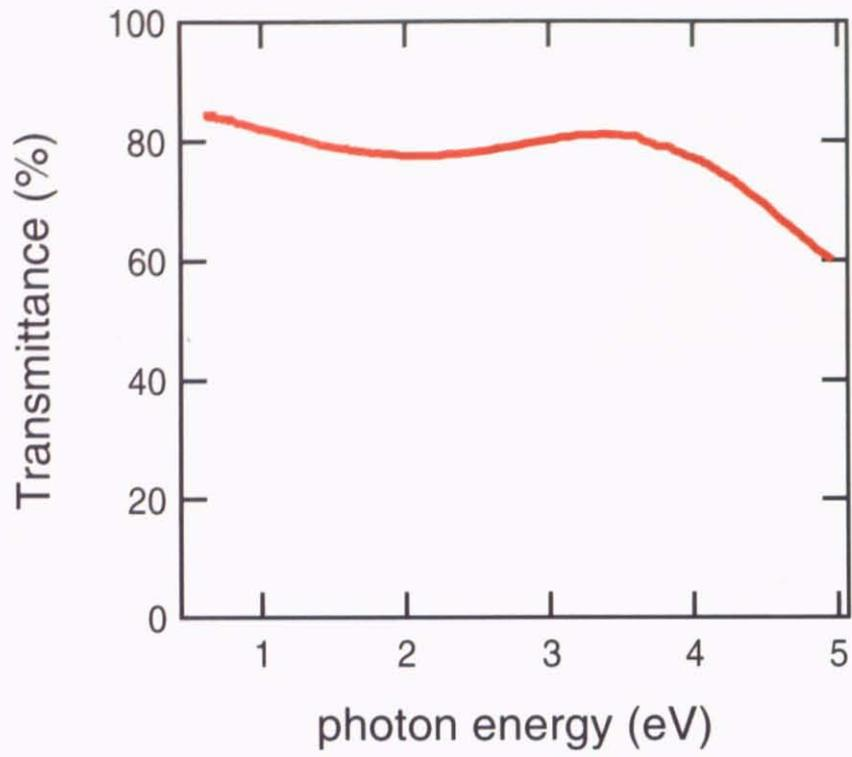
Figure 26: Transmittance of amorphous NGO film on  $\text{Al}_2\text{O}_3$  substrate.
