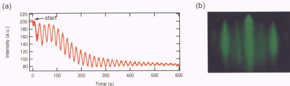
Figure 28: Typical RHEED (a) oscillation , (b) pattern of DSO film grown at 700 °C, 1 mTorr.
