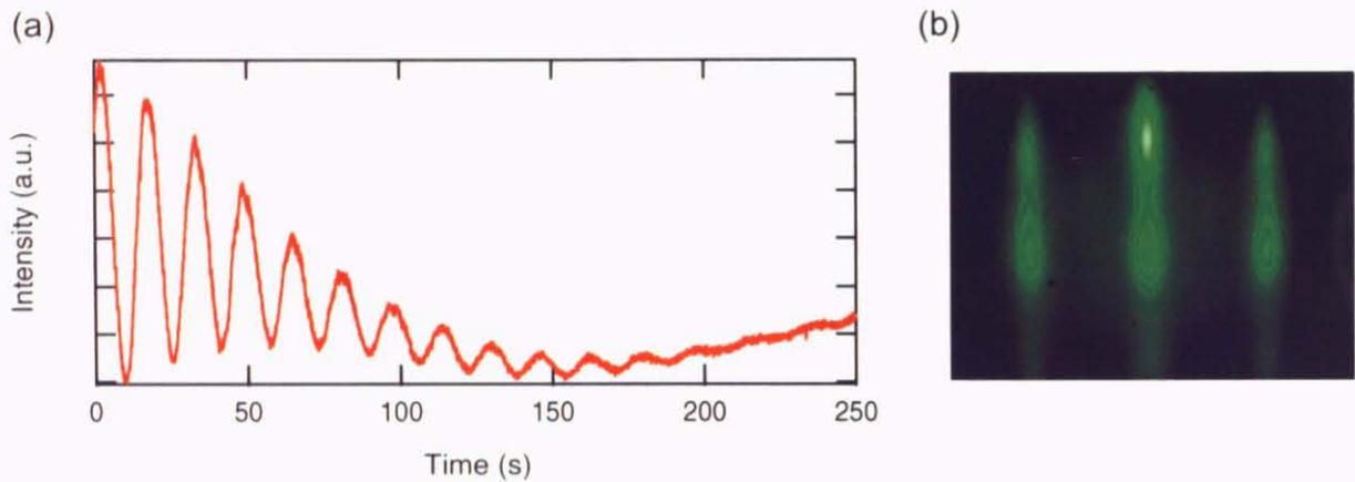
Figure 44: Typical RHEED (a) oscillation, and (b) pattern of epitaxial CHO film grown on Nb:STO substrate at 700 °C, 1 mTorr.
