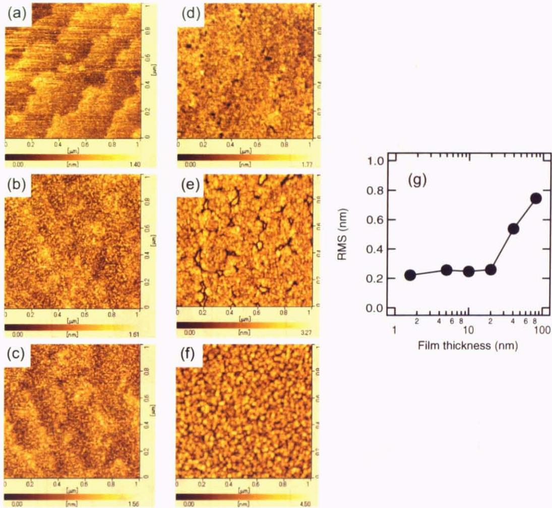
Figure 45: AFM image of epitaxial CHO films with thickness (a) 1.6, (b) 5, (c) 10, (d) 20, (e)40, and (f) 80 nm. These AFM images size are  $1\mu\text{m}\times 1\mu\text{m}$ . (g) RMS of surface morphology of epitaxial CHO films at each film thickness. RMS was calculated using  $1\mu\text{m}\times 1\mu\text{m}$  image.
