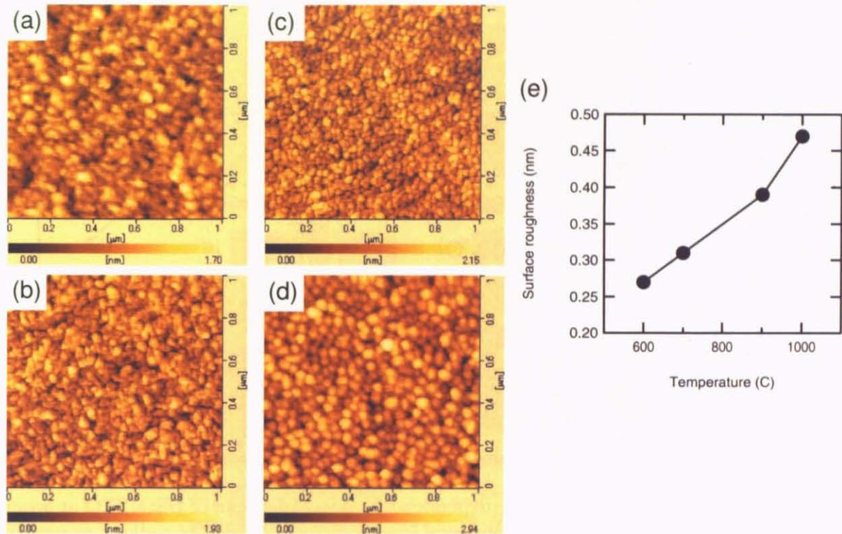
Figure 30: AFM images of surface roughness of DSO film grown at (a) 600, (b) 700, (c) 900, (d) 1000 °C, 1 mTorr. (e) The RMS of surface roughness under these conditions. These AFM images size are 1 μm × 1 μm, and the values of RMS of surface morphology were calculated using 1 μm × 1 μm images.
