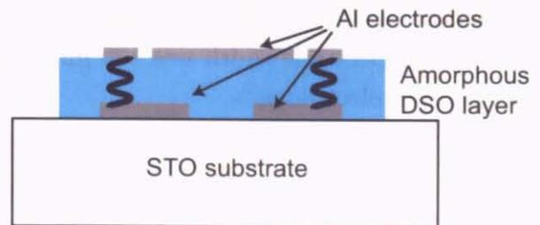
Figure 51: (a) Photograph, (b) Schematic view of an amorphous DSO/STO FET.
