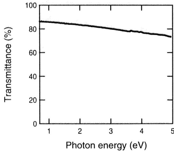
Figure 42: Transmittance of amorphous DSO film on sapphire.
