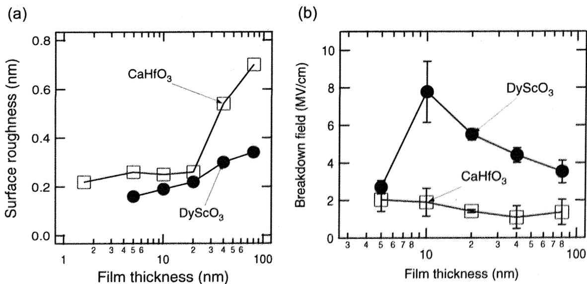
Figure 48: (a) RMS of surface roughness and (b) Average breakdown field of epitaxial DSO and CHO film on Nb:STO.
