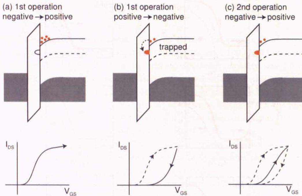
Figure 66: (a) A normal switching behavior is seen during the first scan. (b) At low temperatures, carriers are trapped by trapping sites in the insulator layer, sharply decreasing  $I_{DS}$ . (c) At 50~60 K, some of the trapped carriers can be released. In the higher temperature case, all carriers are released from the trap sites while at low temperatures all carriers remain trapped. Therefore, obvious hysteresis loop could only be observed at 50~60 K.
