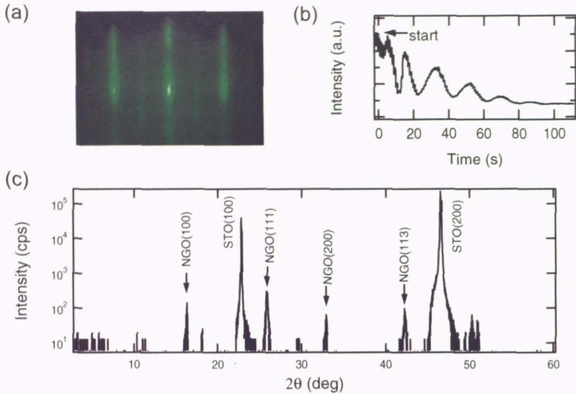
Figure 20: (a) Typical RHEED pattern of NGO film on STO substrate. (b) RHEED oscillation observed during NGO film growth at 700 °C, 1 mTorr. (c) XRD  $2\theta$ - $\theta$  scan of NGO film grown at 700 °C, 1 mTorr.
