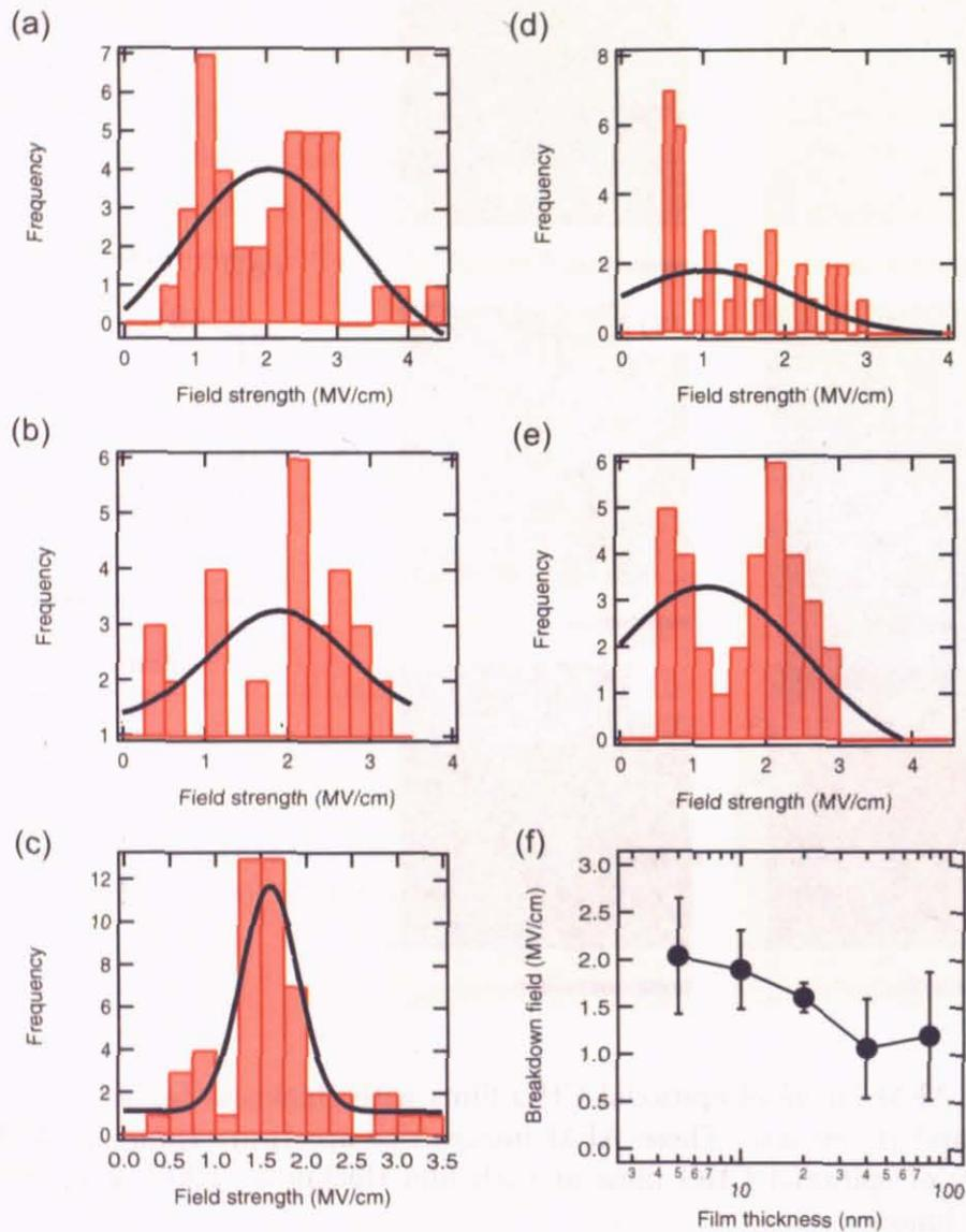
Figure 46: The histogram of breakdown fields of (a) 5, (b) 10, (c) 20, (d)40, and (e) 80 nm thickness epitaxial CHO films on Nb:STO substrates. (f) Average breakdown field of epitaxial CHO films at each film thickness.
