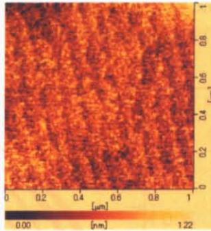
Figure 52: Typical surface morphology of the device surface. The image size is  $1 \times 1 \mu\text{m}^2$ .
