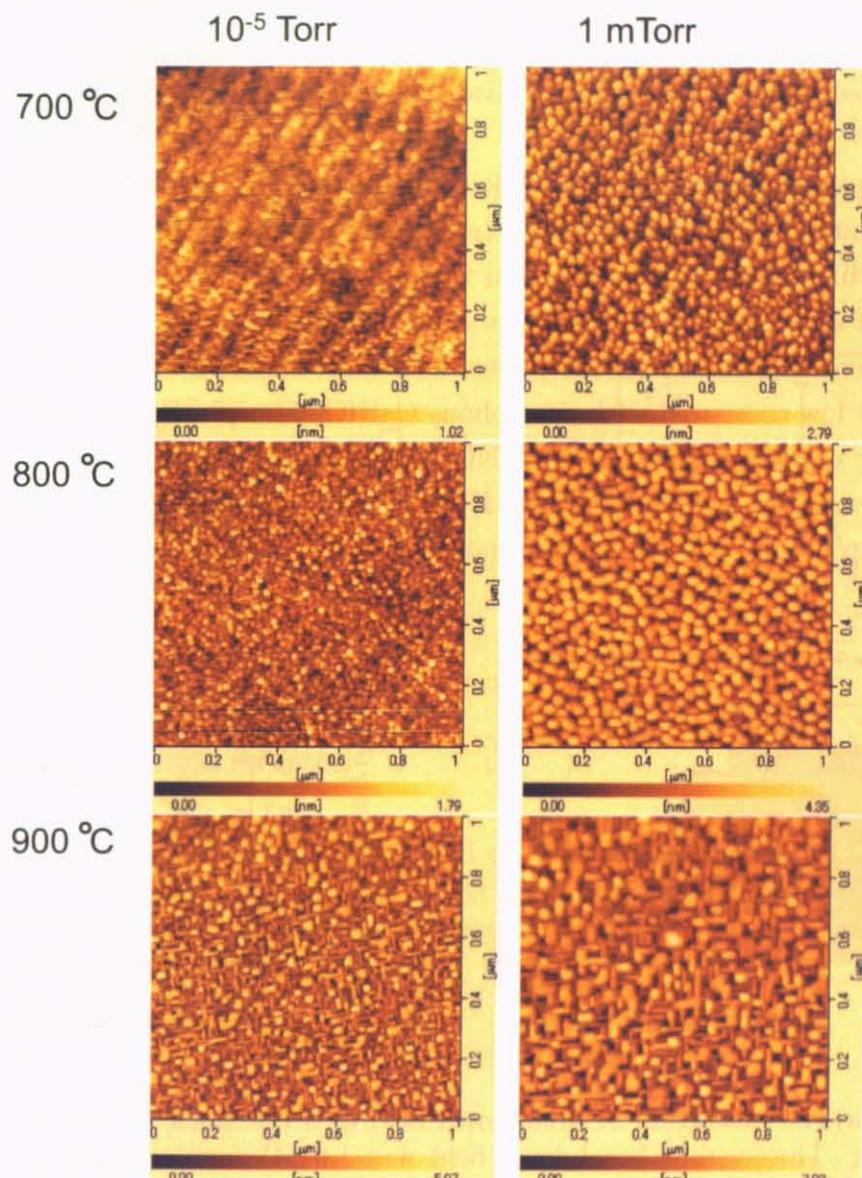
Figure 23: AFM image of 5 nm thick NGO film grown under various conditions. Step and terrace structure can be seen in 700 °C growth film. These AFM images size are 1  $\mu\text{m} \times 1 \mu\text{m}$ .
