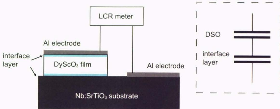
Figure 36: Schematic view of capacitance measurement system, and interfacial layer between film and substrate, Al pad.
