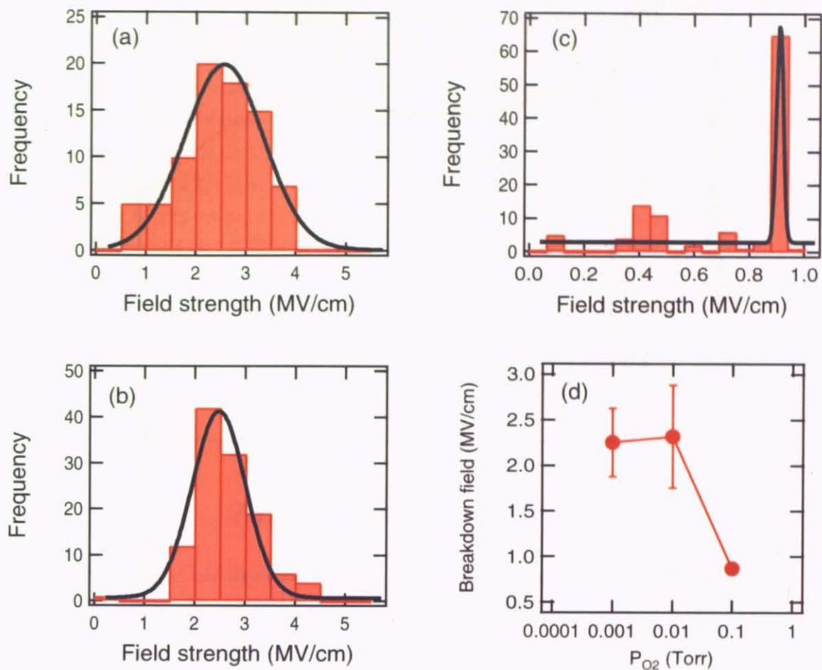
Figure 25: The histogram of breakdown field of amorphous NGO film, (a) grown at 1 mTorr, (b) 10 mTorr, and (c) 100 mTorr oxygen partial pressure. The values of average breakdown field at each oxygen pressure are shown in (d).
