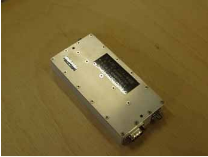
Figure 4.4 Digital phase-shifter
