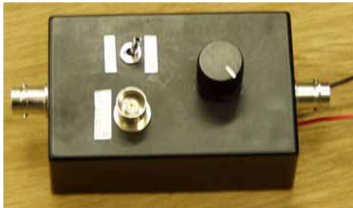
Figure 4.13 Picture of Open/Load Switching Unit
