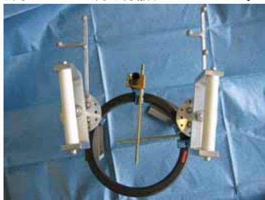
Fig.3 Measurement Instrument for Fracture Reduction Force
