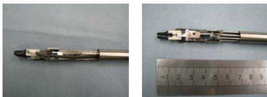
Fig.7: 2-DOF bending forceps
