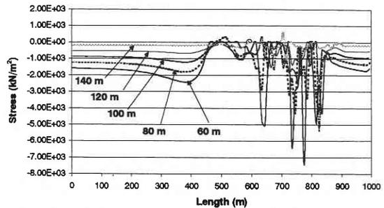
Fig. 11 Stresses in soil deposit (Case 3)
