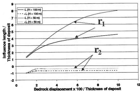
Fig. 13 Influence length (dip angle =  $90^\circ$ )
