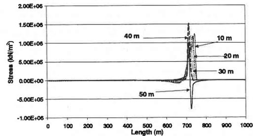
Fig. 5 Stresses in vertical direction in bedrock at regular intervals (Case 1)
