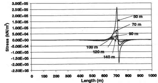
Fig. 6 Stresses in vertical direction in soil deposit at regular intervals (Case 1)
