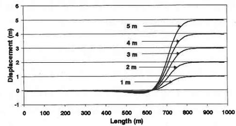
Fig. 4 Surface displacement at each 1-m displacement of hanging wall (Case 1: elastic analysis, dip angle =  $45^{\circ}$ )
