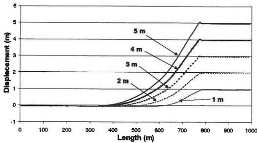
Fig. 7 Surface displacement (Case 2: non-linear analysis, dip angle = 90°)
