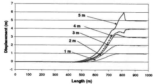
Fig. 10 Surface displacement (Case 3: non-linear analysis, dip angle = 45°)
