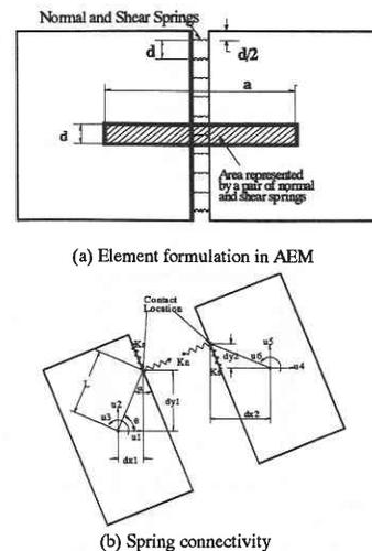
Fig. 1 Element modelling in AEM
