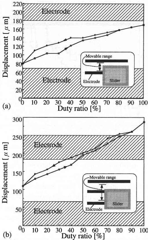
Figure 8 Displacement in the micro-step actuation
