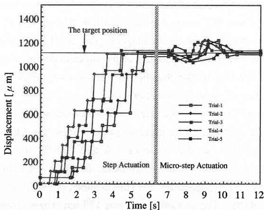
Figure 9 Positioning of the slider in the step and the micro-step actuation
