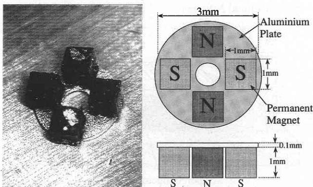
Figure 2 External view and the size of the slider
