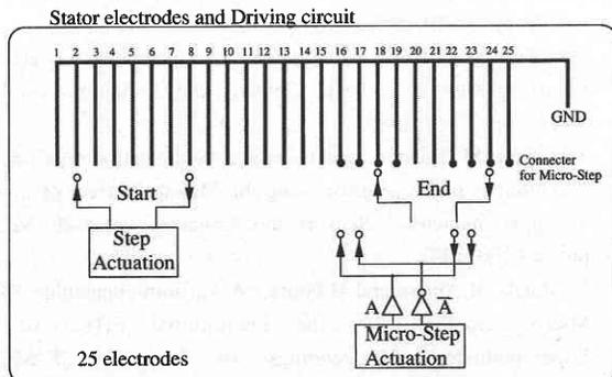
Figure 6 Stator electrodes and the driving circuit connection
