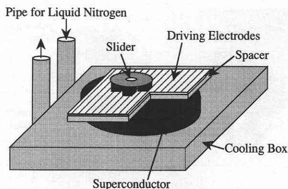
Figure 1 Main part of the actuator
