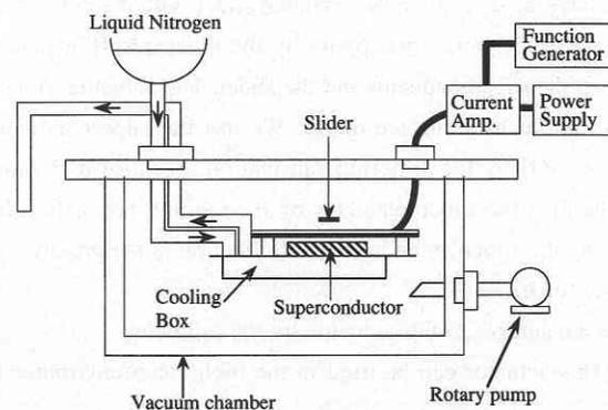
Figure 4 Experimental set up
