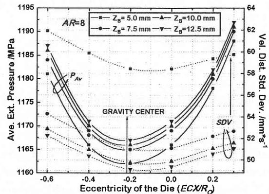
Fig. 3 Variation of  $P_{Av}$  and  $SDV$  at the die entrance with  $EC$  and  $Z_B$  for a "L" section,  $AR = 8$ .
