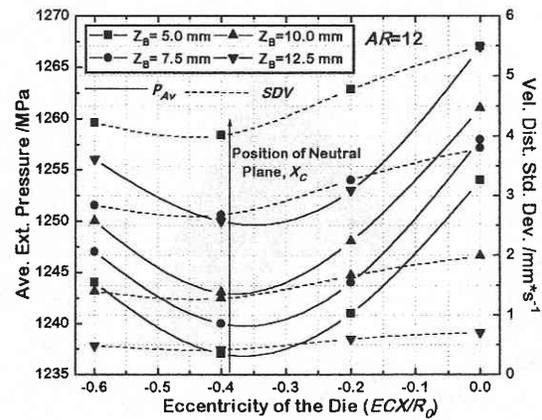
Fig. 10 Effect of  $Z_B$  and  $ECX$  on  $P_{Av}$  and  $SDV$  at the die-exit for a "T" section,  $AR = 12$ .
