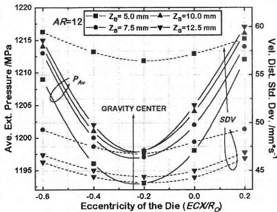
Fig. 2 Variation of  $P_{Av}$  and  $SDV$  at the die entrance with  $EC$  and  $Z_B$  for a "L" section,  $AR = 12$ .
