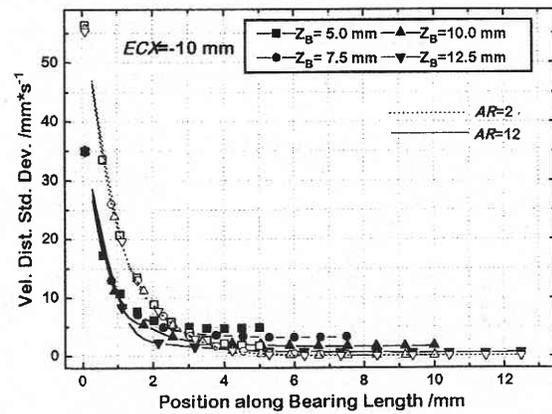
Fig. 7 Variation of  $SDV$  along bearing length for “T” sections,  $ECX = -10$  mm.
