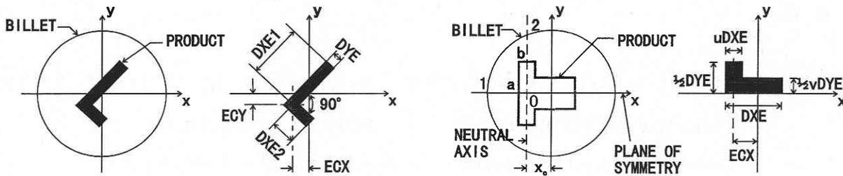
Fig. 1 Computational models of "L" sections and "T" sections.
