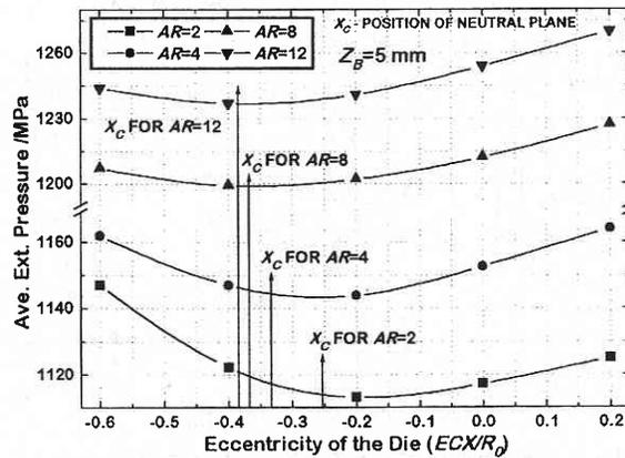
Fig. 8 Effect of  $ECX$  and  $AR$  on  $P_{Av}$  for “T” sections,  $Z_B = 5$  mm.
