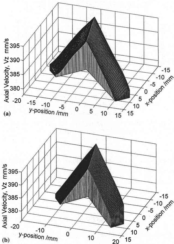
Fig. 6  $V_z$  profiles for a “L” section,  $AR = 8$ ,  $ECX = -10$  mm,  $Z_B = 7.5$  mm (a)  $ECY = 26.67$  mm (b)  $ECY = -3.33$  mm.
