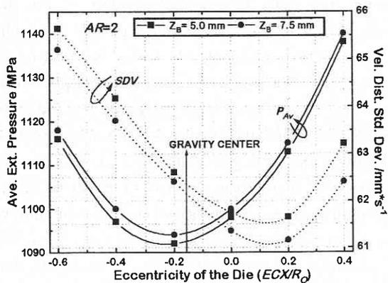
Fig. 4 Variation of  $P_{Av}$  and  $SDV$  at the die entrance with  $ECX$  and  $Z_B$  for a "L" section,  $AR = 2$ .
