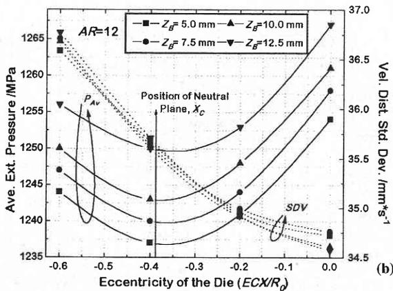
Fig. 9 Variation of  $P_{Av}$  and  $SDV$  at the die entrance with  $EC$  and  $Z_B$  for "T" sections (a)  $AR = 12$ , (b)  $AR = 2$ .
