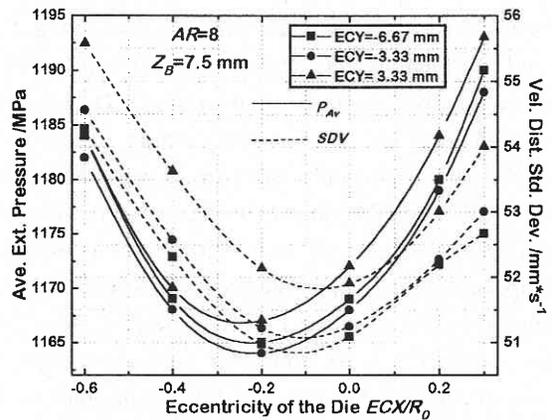
Fig. 5 Variation of  $P_{Av}$  and  $SDV$  at the die entrance with  $ECX$  and  $ECY$  for a "L" section,  $AR = 8$ ,  $Z_B = 7.5$  mm.
