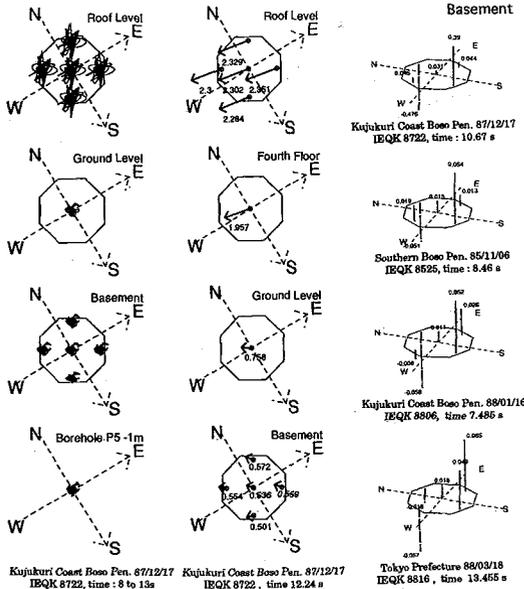
Fig. 4 Displacement orbit graphs      Fig. 5 Diagrams of displacements (cm)      Fig. 6 Vertical Displacements (cm)
