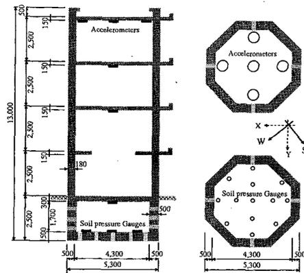
Fig. 1(a) Plan and cross-section of the tower [4]
