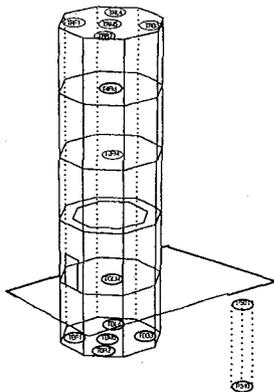
Fig. 1(b) Locations of the Accelerometers
