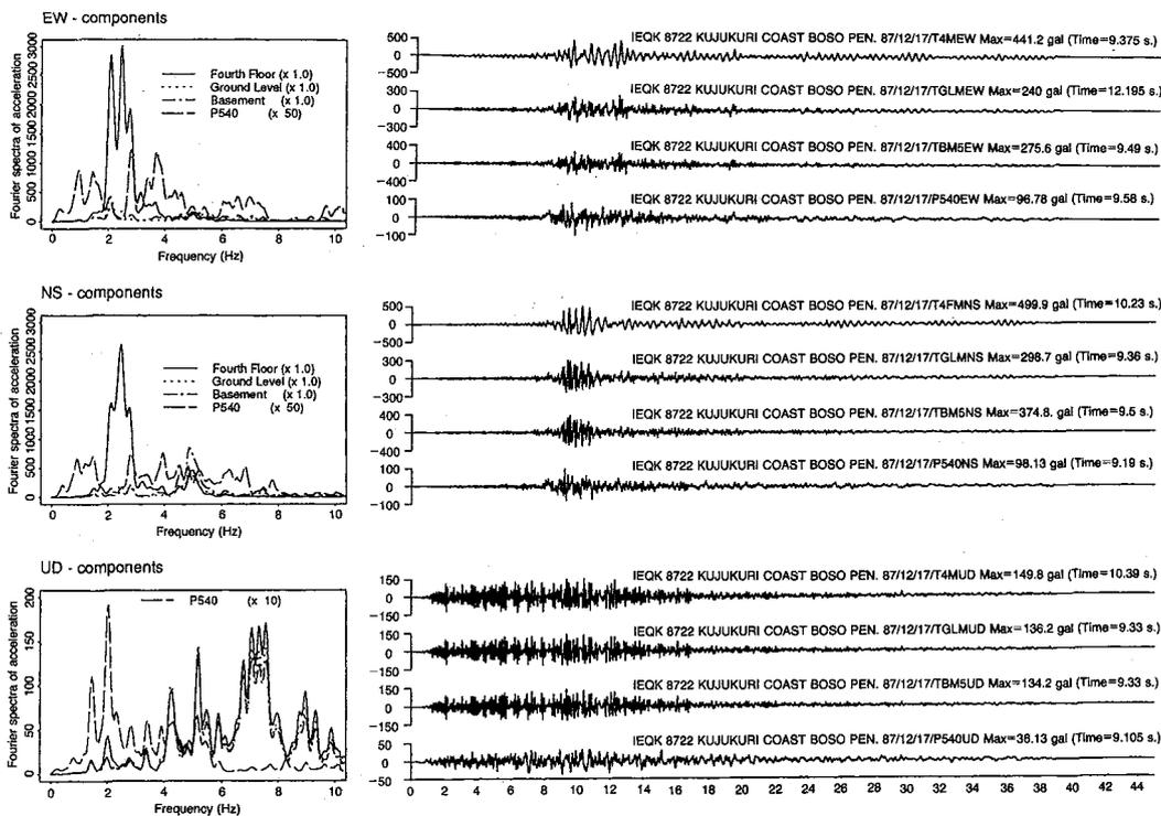
Fig. 3 Fourier spectra and wave forms (IEQK 8722)
