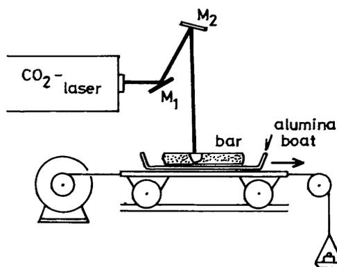
Fig. 1 Schematic illustration of the HTMZ system for Bi-2212 crystal growth with  $\text{CO}_2$ -laser heating.
