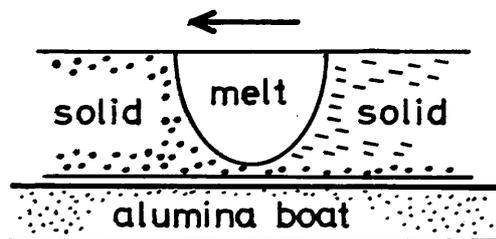
Fig. 2 Schematic cross section of Bi-2212 bar set on alumina boat under laser heating.
