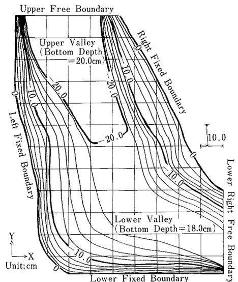
Fig.1 A Plan of Alluvial Layer of a Experimental Ground Model
