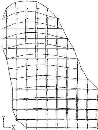
Fig.2 Fundamental Natural Mode of the Analysis
