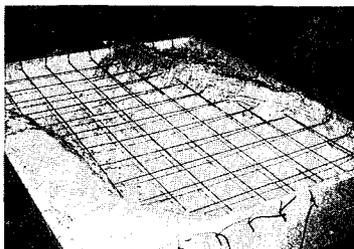
Photo.1 A Photograph of the Test Ground Model (The valley shape is formed by plaster)
