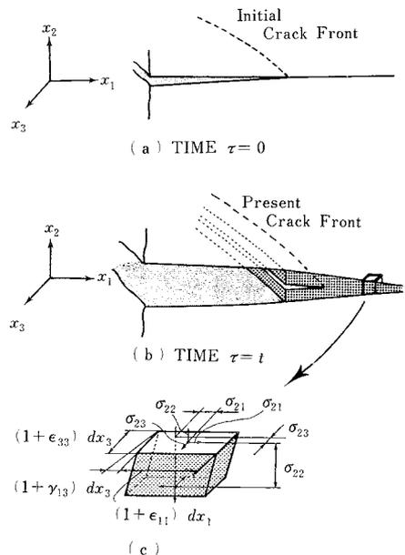
Fig.1 Discontinuous crack model
