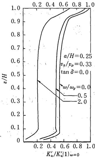
Fig. 8 Vertical Distribution of Local Dynamic Stiffness for Horizontal Vibration (Eq. (42))
