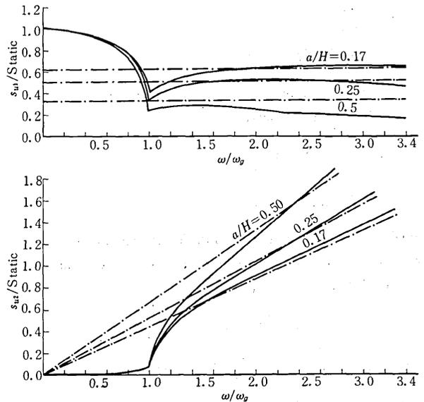
Fig. 9 Variations of Horizontal Dimensionless Dynamic Stiffness with Frequency and the  $a/H$  Ratio (Eq. (43) or (44)). Full Line for the Proposed Solution and Dashed Line for the Approximate Solution by Novak
