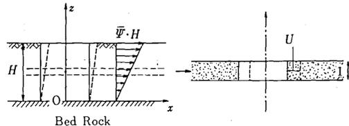
Fig. 7 Notation and Horizontal Displacement of Cylinder
