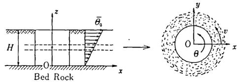
Fig. 4 Notation and Torsional Displacement of Cylinder
