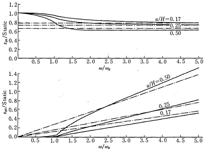
Fig. 6 Variations of Torsional Dimensionless Dynamic Stiffness with Frequency and the  $a/H$  Ratio (Eq. (28) or (29). Full Line for the Proposed Solution and Dashed Line for the Approximate Solution by Novak
