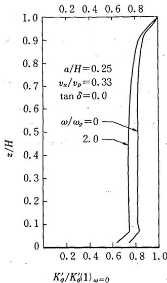
Fig. 5 Vertical Distribution of Local Dynamic Stiffness for Torsion (Eq. (27))
