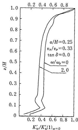
Fig. 2 Vertical Distribution of Local Dynamic Stiffness for Vertical Vibration (Eq. 13)
