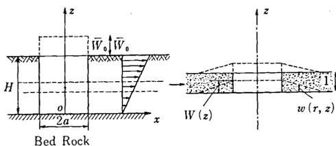
Fig. 1 Notation and Vertical Displacement of Cylinder in which  $\lambda$  and  $G$  are lame's constants,  $G'$  is the viscosity modulus associated with  $G$ , and  $\rho$  is a mass density of the surface soil stratum. The viscosity is introduced only in the shear modulus  $G$ .
