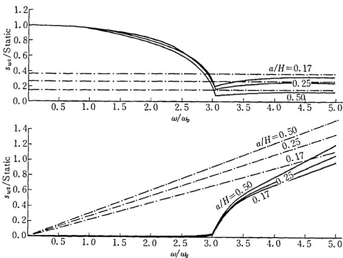
Fig. 3 Variations of Vertical Dimensionless Dynamic Stiffness with Frequency and the  $a/H$  Ratio (Eq. (14) or (15)). Full line for the Proposed Solution and Dashed line for the Approximate Solution by Novak
