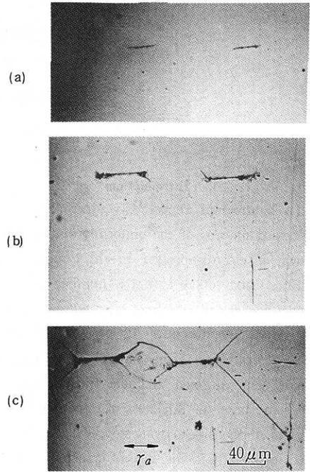
Fig. 4 Process from initiation of cracks to branching (a)  $n=1.4 \times 10^5$ , (b)  $n=1.8 \times 10^5$ , (c)  $n=2.4 \times 10^5$ ,  $\gamma_a=1.09 \times 10^{-3}$ ,  $N=3.4 \times 10^5$
