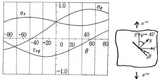
Fig. 13. Stress components in plane bending
