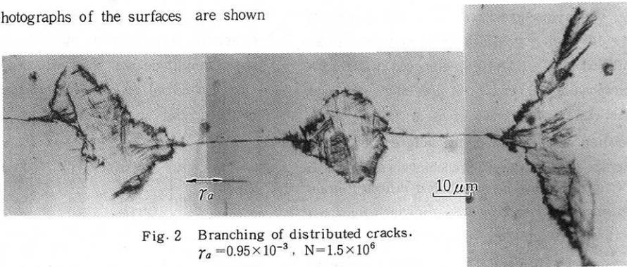
Fig. 2 Branching of distributed cracks.
