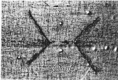
Fig. 10. Branching in specimen B which had a little larger grain size. It is shown that the branching angle is  $45^\circ$ .  $\gamma_a = 1.2 \times 10^{-3}$ ,  $N = 1.15 \times 10^5$
