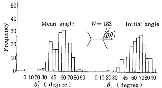
Fig. 9 Distribution of branching angles, specimen A and minute grain size.
