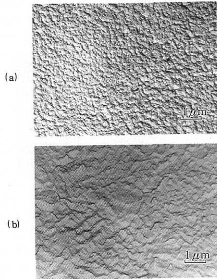
Fig. 1 Crystal structure of electrodeposited copper (a) Specimen A, grain size: 0.2 to 0.3  $\mu\text{m}$ . (b) Specimen B, grain size: about 1  $\mu\text{m}$
