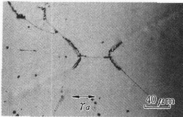
Fig. 3 Transition from distributed cracks to stage II cracks
