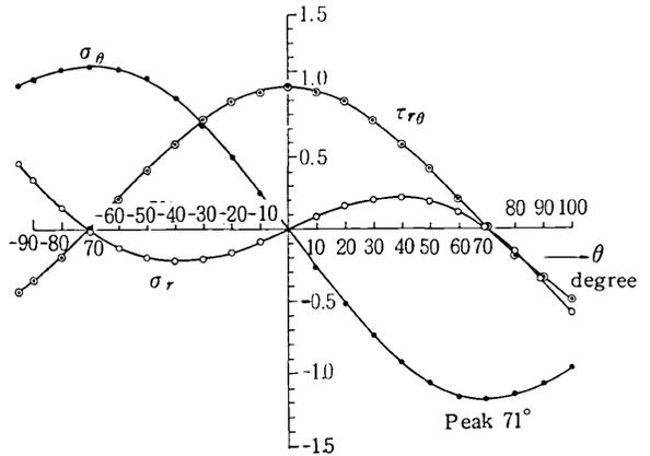
Fig. 8 Variation of stress components near a crack tip in the case of torsion test
