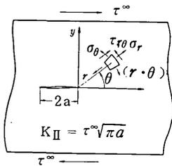
Fig. 7 Stress components at advancing edge of a crack in the case of torsion test
