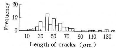
Fig. 5 Distribution of the maximum crack length between branching. (Specimen A, number of measurements  $n=70$ , mean value  $\bar{x}=53.8 \mu\text{m}$ , standard deviation  $s=26.6 \mu\text{m}$ )
