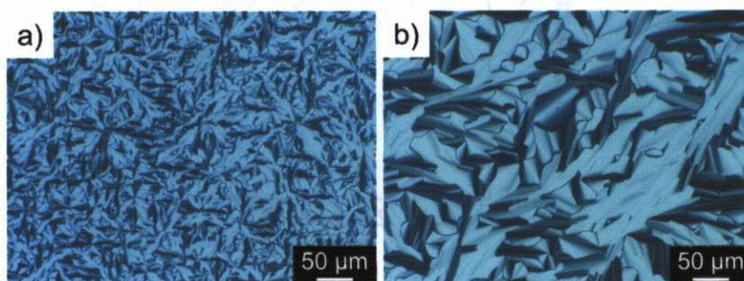
**Figure 3–12.** Polarized optical micrographs of (a)  $\text{IL}(\text{CF}_3\text{SO}_3^-)$  and (b)  $\text{IL}(\text{PF}_6^-)$  in the hexagonal columnar phases at 50 °C.
