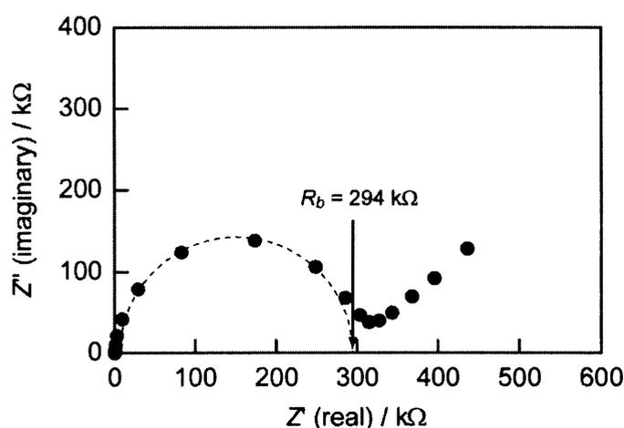
**Figure 3–6.** Impedance spectrum for **1c** aligned perpendicular to the comb-shaped gold electrode in the columnar state at 100 °C. The cell constant is 47.6 cm<sup>-1</sup>. The bulk resistance  $R_b$  was obtained from the intercept of the left semi-circle on the  $Z'$  axis.
