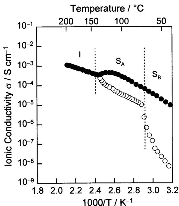
**Figure 2–8.** Anisotropic ionic conductivities of the homeotropically aligned smectic liquid crystalline complexes composed of equimolar amounts of **2** and **3**: (●) parallel and (○) perpendicular to the smectic layer plane.
