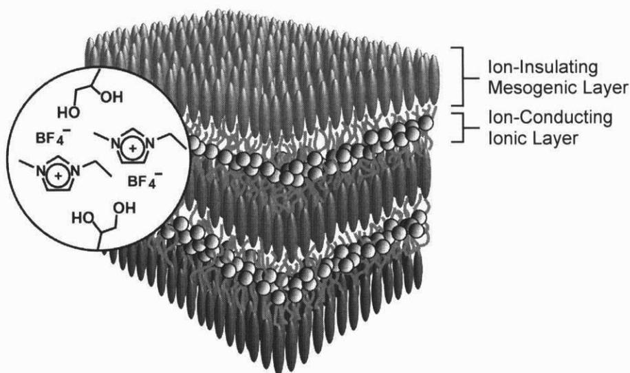
**Figure 2–6.** Illustration of nanophase-segregated layered structures composed of **1a** and **2**.
