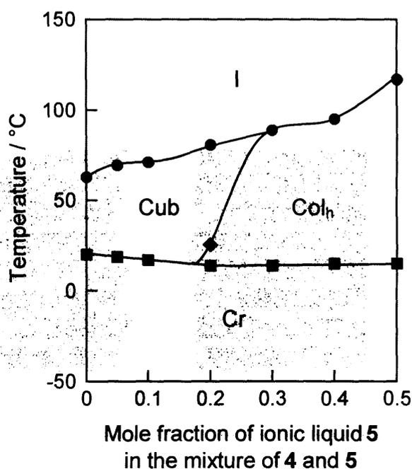
**Figure 2–12.** Phase transition behavior for the mixtures of mesogenic molecule **4** and ionic liquid **5** on cooling. Col<sub>h</sub>: hexagonal columnar, Cr: crystalline, Cub: cubic, I: isotropic.
