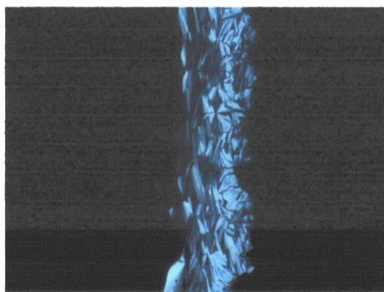
**Figure 2–11.** Polarized optical micrograph of the  $\text{Col}_h$  phase induced in the contact region between the isotropic liquid phase of ionic liquid **5** (optically isotropic region at the left-hand side) and the micellar cubic phase of compound **4** (right-hand side) at room temperature.
