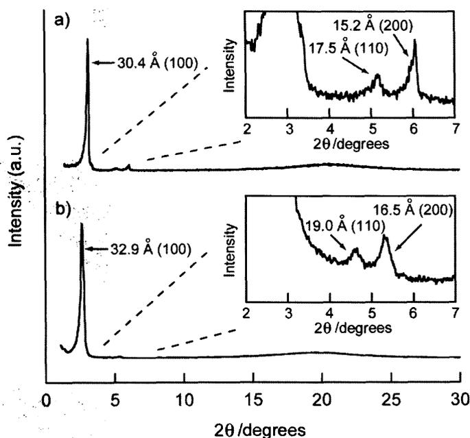
**Figure 3–3.** WAXD patterns of the  $\text{Col}_h$  phases of a) **1c** and b) **1e** at 25 °C. Insets indicate the enlarged views of the small-angle region.
