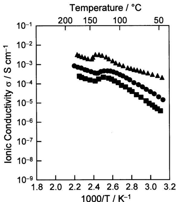
**Figure 2–9.** Ionic conductivities parallel to the smectic layer of the homeotropically aligned mixtures of **2** and **3** in the molar ratio of 7:3 (▲), 8:2 (●), and 9:1 (■).
