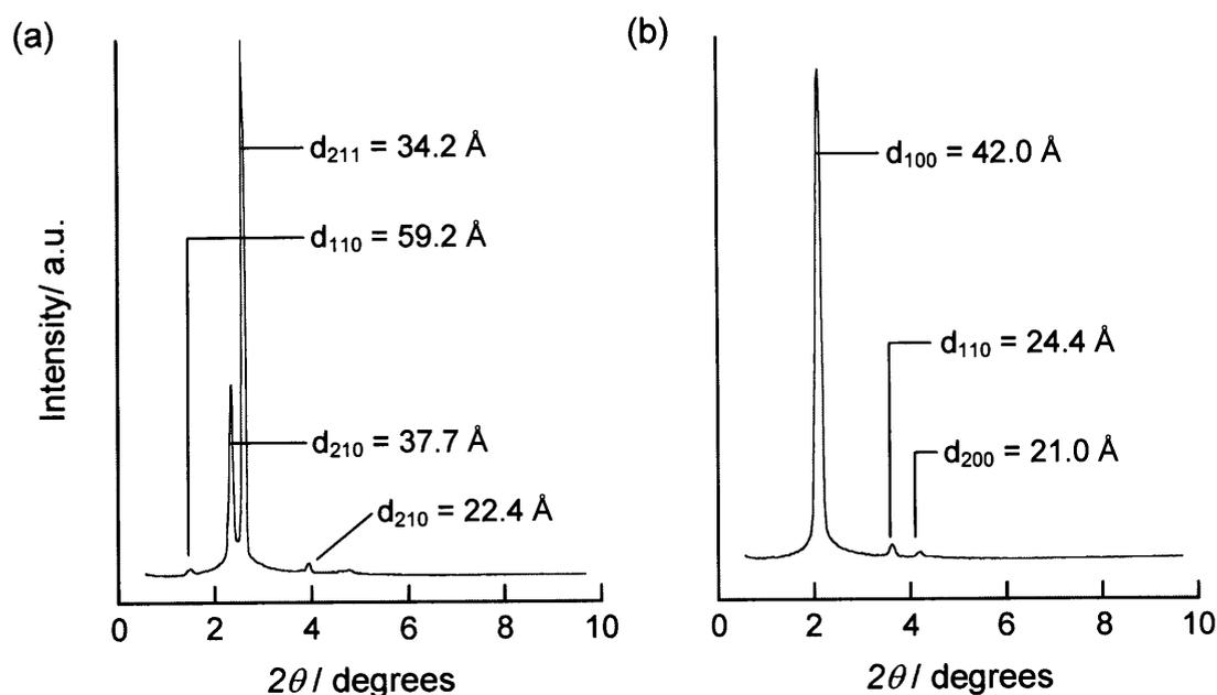
**Figure 2–13.** X-ray diffraction patterns of (a) the mixture of **4** and **5** (8:2 molar ratio) at 50 °C and (b) the equimolar mixture of **4** and **5** at 50 °C.
