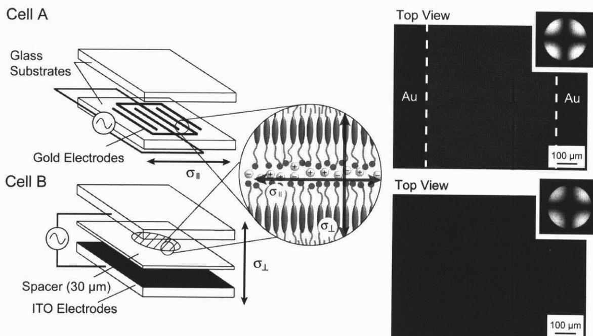
**Figure 2–4.** Schematic illustrations of the Cell A and B for the anisotropic ion-conductive measurements (left). The samples forming the smectic liquid crystalline phases are filled between electrodes. The samples composed of equimolar amounts of an ionic liquid and mesogenic compounds form homeotropically aligned monodomains in the cells (center). The orthoscopic and conoscopic images at 120 °C for the mixture of **1b** and **2** filled in these cells are also shown (right).
