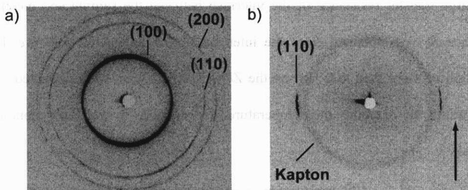
**Figure 3–5.** 2D SAXS patterns of **1c** in the Col<sub>h</sub> state at 25 °C: a) unoriented **1c** and b) oriented **1c** by shearing. An arrow indicates the shearing direction. A halo shown in the figure b) originates from the X-ray scattering from a Kapton film. (100) and (200) diffraction arcs are not observed.
