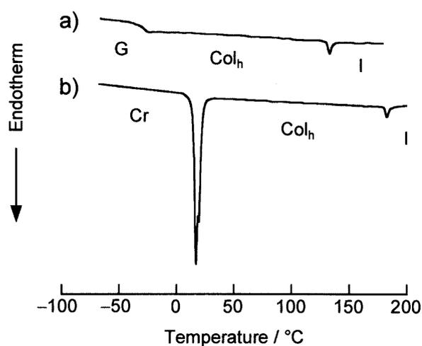
**Figure 3–2.** DSC thermograms of a) **1c** and b) **1e** on the second heating at a scanning rate of 10 °C min<sup>-1</sup>. Col<sub>h</sub>: hexagonal columnar; Cr: crystalline; G: glassy; I: isotropic.
