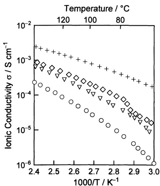
**Figure 3–13.** Ionic conductivities of  $\text{IL}(\text{X}^-)$  as a function of temperature: (+) for  $\text{IL}((\text{CF}_3\text{SO}_2)_2\text{N}^-)$ , ( $\diamond$ ) for  $\text{IL}(\text{CF}_3\text{SO}_3^-)$ , ( $\nabla$ ) for  $\text{IL}(\text{PF}_6^-)$ , ( $\circ$ ) for  $\text{IL}(\text{BF}_4^-)$ .
