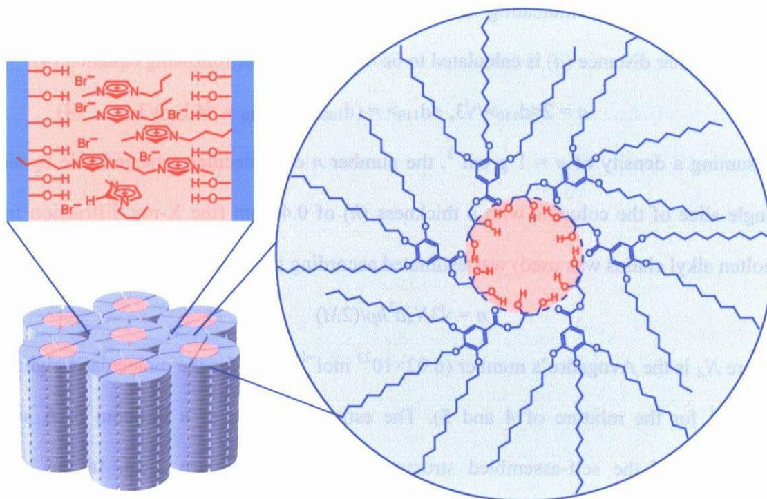
**Figure 2–14.** Illustration of the formation of self-assembled columnar structure.
