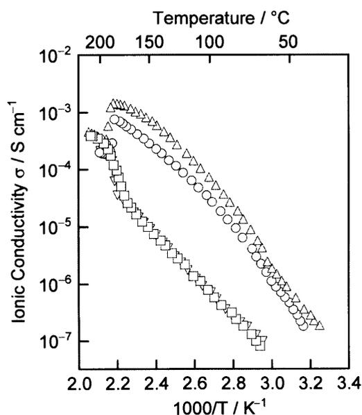
**Figure 3–9.** Anisotropic ionic conductivities of **1e** alone and complex of **1e** and  $\text{LiBF}_4$  (molar ratio of  $\text{LiBF}_4$  to **1e**: 0.25): ( $\Delta$ ) parallel and ( $\nabla$ ) perpendicular to the columnar axis for the oriented complex.
