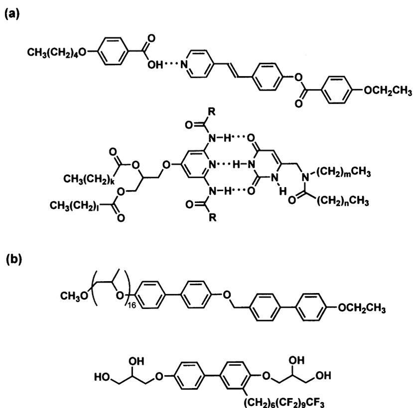
**Figure 1–7.** Specific liquid crystals: (a) supramolecular hydrogen-bonded liquid crystals; (b) microphase-segregated liquid crystals.
