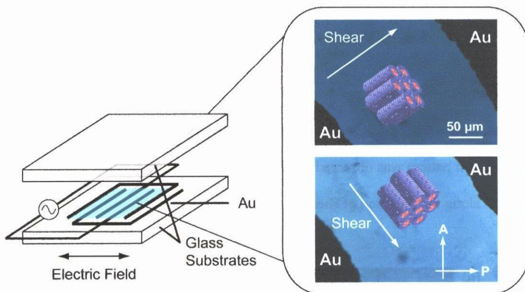
**Figure 2–21.** Schematic illustration of a glassy cell with comb-shaped gold electrodes with thickness of 0.8 μm for the anisotropic ion-conduction measurements (left). The columnar liquid crystal is filled between electrodes and aligned in two directions by shearing perpendicular and parallel to the electrodes. Polarized optical micrographs and illustrations of the oriented sample in the Col<sub>h</sub> state at 50 °C. Directions of A: analyzer and P: polarizer.
