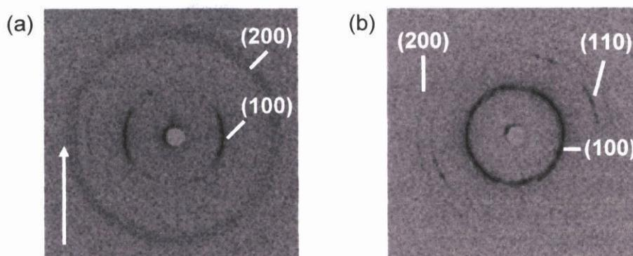
**Figure 2–20.** Two-dimensional X-ray scattering images of the mixture of **4** and **5** in the hexagonal columnar phase: (a) oriented sample of the mixture by shearing and (b) non-oriented sample of the mixture. The arrow shows the direction of shearing.
