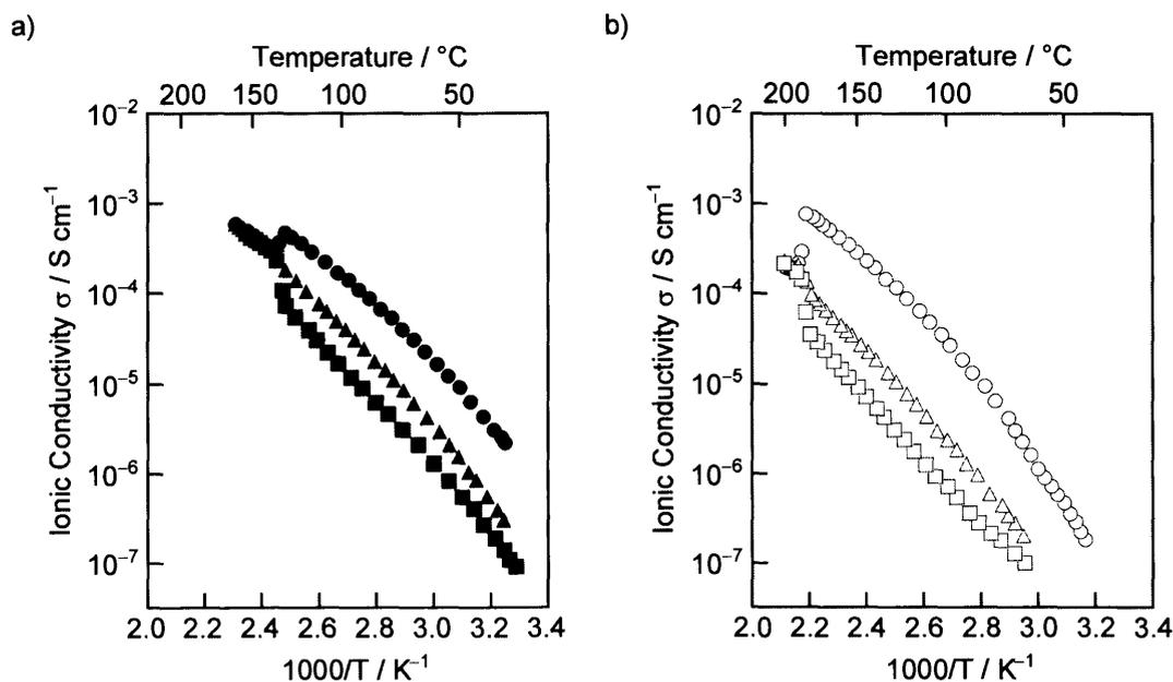
**Figure 3-8.** Anisotropic ionic conductivities of a) **1c** and b) **1e** as a function of temperature: (●) parallel and (■) perpendicular to the columnar axis for oriented **1c**; (▲) for unoriented sample of **1c**; (○) parallel and (□) perpendicular to the columnar axis for oriented **1e**; (Δ) for unoriented sample of **1e**.
