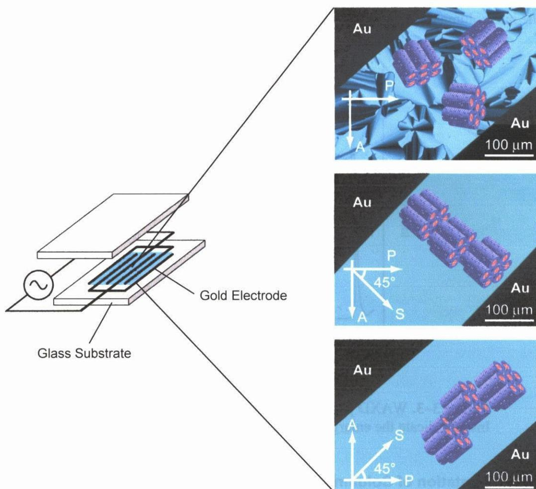
**Figure 3-4.** Schematic illustration of a glassy cell with comb-shaped gold electrodes with thickness of  $0.8 \mu\text{m}$  for the anisotropic ion-conduction measurements (left). The samples forming the  $\text{Col}_h$  phases are filled between electrodes. Polarizing optical microscopic images and illustrations of the oriented and self-assembled structures of **1e** in the  $\text{Col}_h$  state at  $25^\circ\text{C}$  (right). Directions of A: analyzer; P: polarizer; S: shearing.
