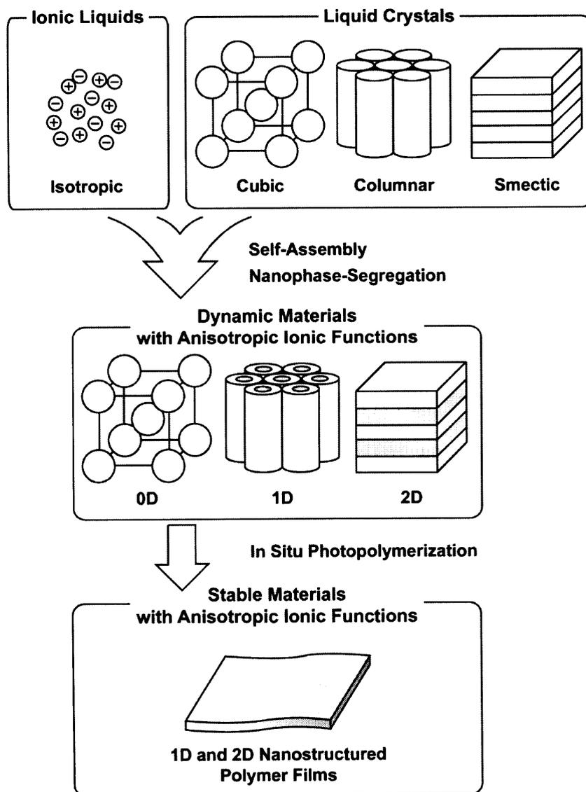
**Figure 1–10.** Schematic illustration of the design strategies for the development of anisotropic ion-conductive materials based on ionic liquids.
