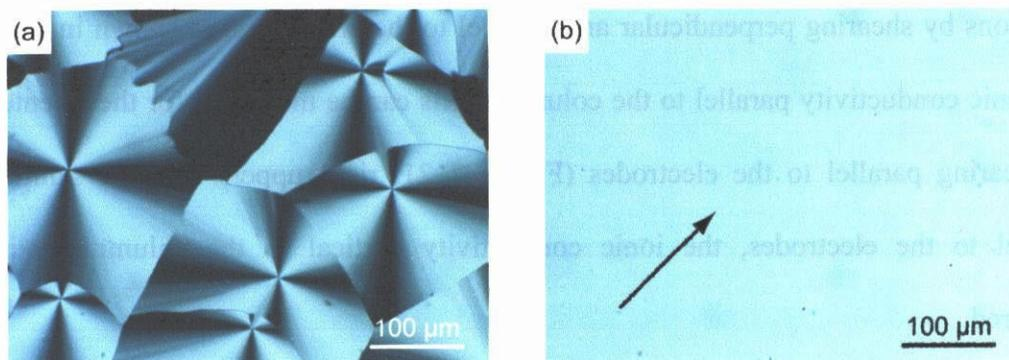
**Figure 2–19.** Polarized optical micrographs of the equimolar mixture of **4** and **5** in the  $Col_h$  phase at room temperature: (a) before shearing; (b) after shearing the materials. The arrow shows the direction of shearing.
