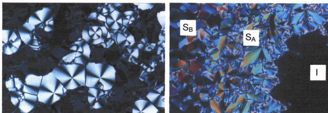
**Figure 2-3.** Polarized light optical photomicrographs of the texture of **1a** in the Col phase at 100 °C (left) and the contact region of **1a** with **2** (right-hand side) at 100 °C (right).
