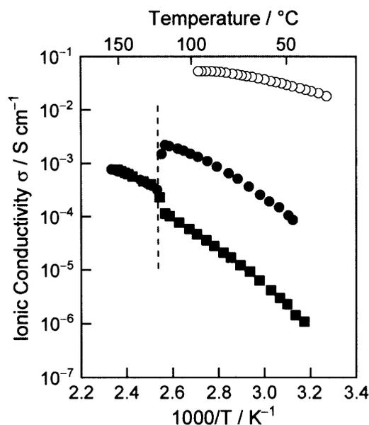
**Figure 2–22.** Temperature dependence of ionic conductivities for ionic liquid **5** alone (○) and the columnar liquid crystal composed of equimolar amount of **4** and **5** (■) parallel and (●) perpendicular to the columnar axis).
