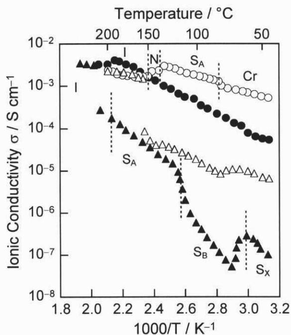
**Figure 2–5.** Anisotropic ionic conductivities of the homeotropically aligned smectic liquid crystalline complexes composed of equimolar amounts of **1** and **2**: (●) parallel and (▲) perpendicular to the smectic layer plane for **1a** and **2**; (○) parallel and (△) perpendicular to the smectic layer plane for **1b** and **2**.
