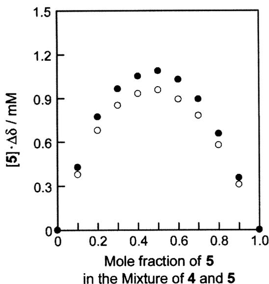
**Figure 2–17.** Job's plot determined by <sup>1</sup>H NMR spectroscopy indicating the 1:1 stoichiometry of the complex formed between **4** and **5**. (●):  $\Delta\delta$  for the H<sup>a</sup> resonance of **4** induced by the addition of **5** and (○):  $\Delta\delta$  for the H<sup>b</sup> resonance of **4** induced by the addition of **5**. Total concentration of **4** and **5** is maintained at 10 mM.
