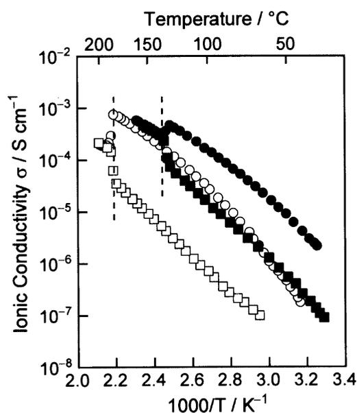
**Figure 3–7.** Anisotropic ionic conductivities of **1c** and **1e** as a function of temperature: (●) parallel and (■) perpendicular to the columnar axis for **1c**; (○) parallel and (□) perpendicular to the columnar axis for **1e**. The broken lines denote the Col<sub>h</sub>-I phase transition temperatures
