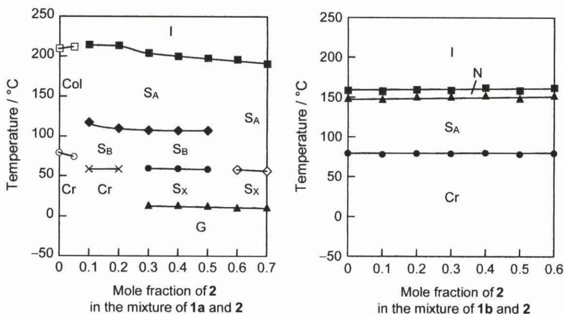
**Figure 2-2.** Phase transition behavior for a mixture of **1a** and **2** (left) and a mixture of **1b** and **2** (right) determined by DSC on the second heating. Cr: crystalline,  $S_A$ : smectic A,  $S_B$ : smectic B,  $S_X$ : unidentified smectic, Col: columnar, G: glassy, N: nematic.
