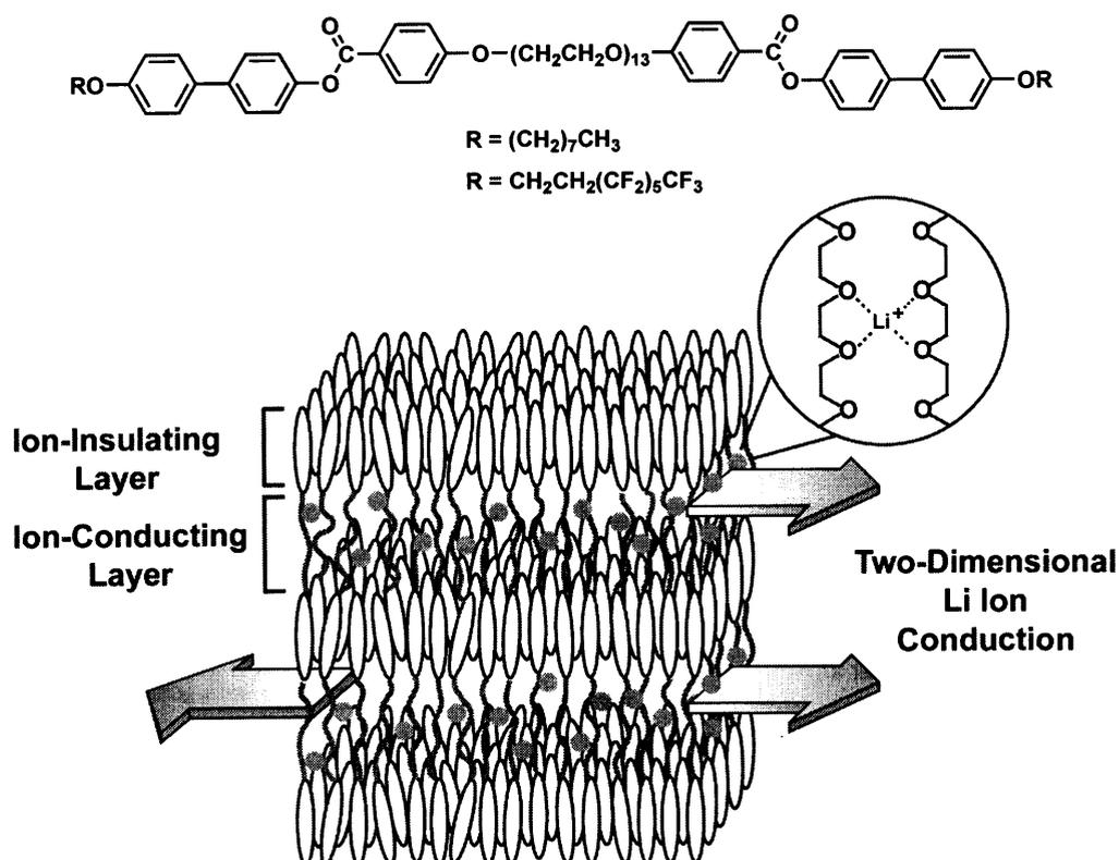
**Figure 1–9.** Two-dimensionally anisotropic ion-conductive liquid crystals.
