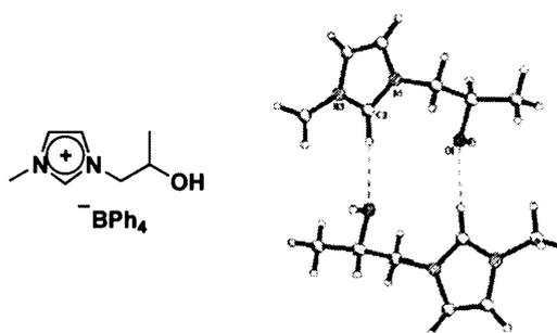
**Figure 2–18.** Molecular structures and crystal structure of imidazolium salt reported by Rogers.<sup>39</sup> The hydrogen-bonded dimer formed by R/S-pairs of the 1-(2-hydroxypropyl)-3-methylimidazolium cations.
