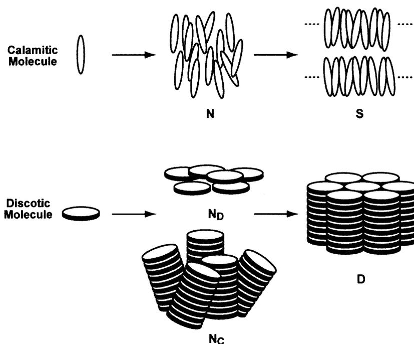
**Figure 1–5.** Representation of the molecular shape and orientation of the major thermotropic liquid crystalline phases. N: nematic phase; S: smectic phase; N<sub>D</sub>: discotic nematic phase; N<sub>C</sub>: columnar nematic phase; D: discotic phase.
