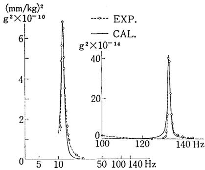
Fig. 4 Response curve of a steel with spring (II)
