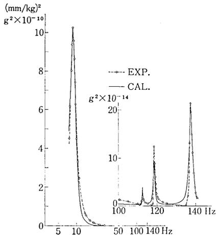
Fig. 3 Response curve of a steel with spring (I)
