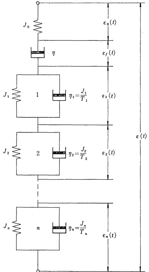
Fig. 1 The generalized Voigt (or Kelvin) model for uniaxial stress field. For deviatoric or bulk deformation,  $J_0, J_1, T_1, \dots$  are replaced by  $D_0, D_1, T_{D,1}, \dots$  and  $B_0, B_1, T_{B,1}, \dots$ .
