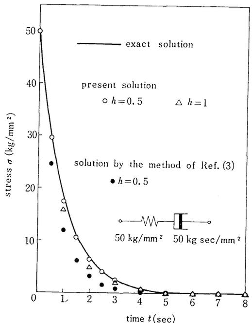
Fig. 2 Stress relaxation test of a Maxwell model.
