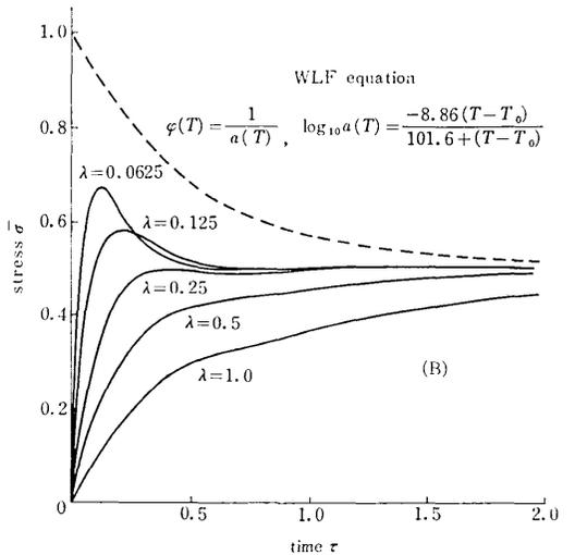
Fig. 3 Stress relaxation of a viscoelastic bar. Material property is temperature-independent in (A), and temperature-dependent in (B) according to the WLF postulate.
