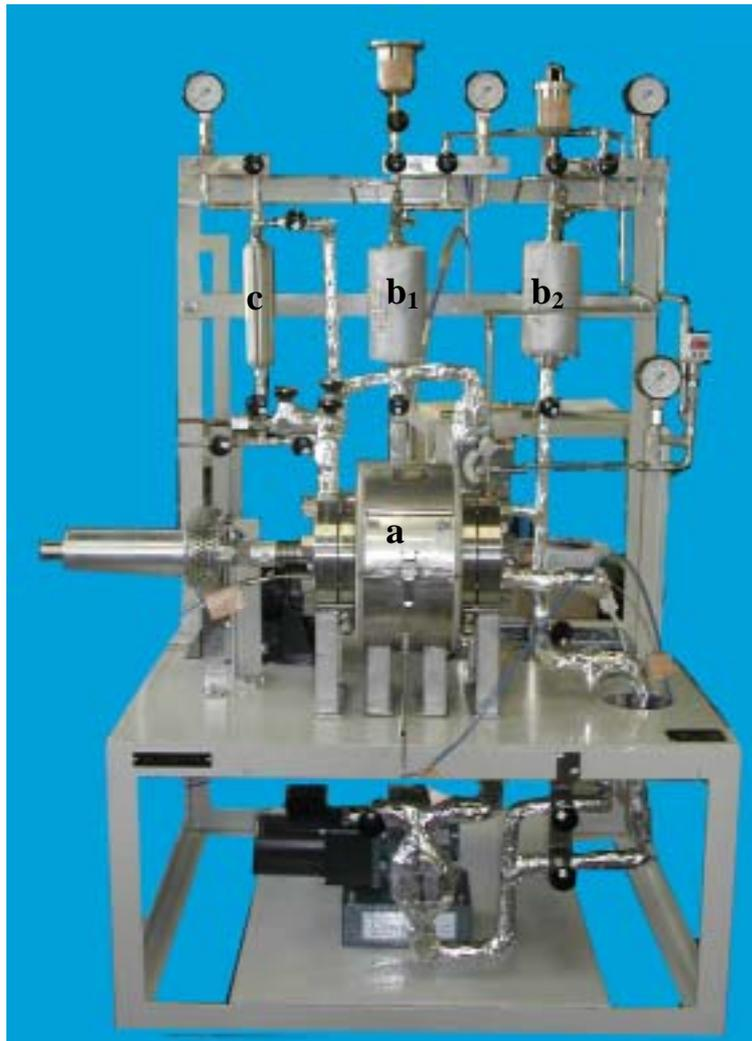
Fig.2.1 The laboratory wood-cooking equipment for optimization of modified cooking
