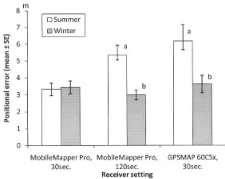
Fig. 2. GPS positioning accuracy by receiver setting in summer and winter. Means followed by different letters differ significantly according to Welch's t-test ( $p < 0.05$ ).
