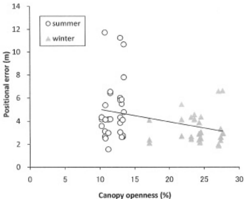
Fig. 5. Relationship between canopy openness and GPS positional errors. Each dot indicates the mean error of three repetitions by the same receiver setting with different satellite visibility conditions.
