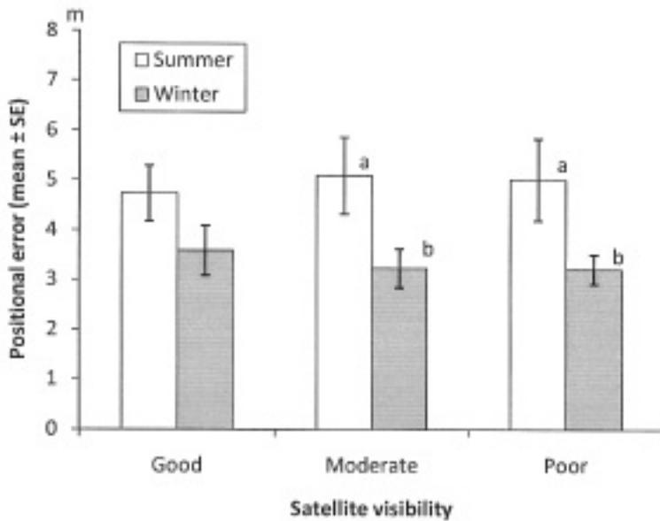
Fig. 3. GPS positioning accuracy by satellite visibility in summer and winter. Means followed by different letters differ significantly according to Welch's t-test ( $p < 0.05$ ).
