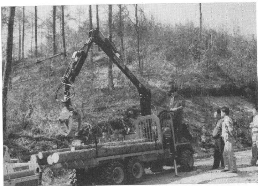
図-5 日本製の林内作業車の実演状況. Fig. 5. Small-size forwarder made in Japan.
