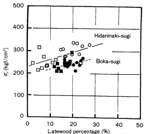
Fig. 22. Relationship between compressive strength parallel to the grain ( $\sigma_c$ ) and latewood percentage. squares: juvenile wood, circles: mature wood
