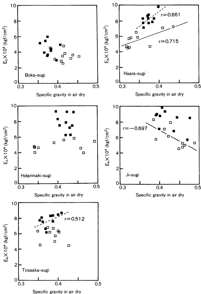
Fig. 7. Relationship between Young's modulus in bending ( $E_b$ ) and specific gravity in air dry.
