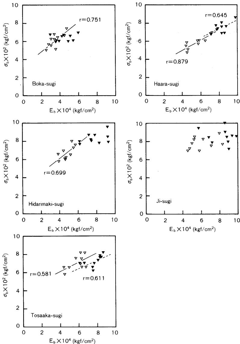
Fig. 15. Relationship between bending strength ( $\sigma_b$ ) and Young's modulus in bending ( $E_b$ ).
