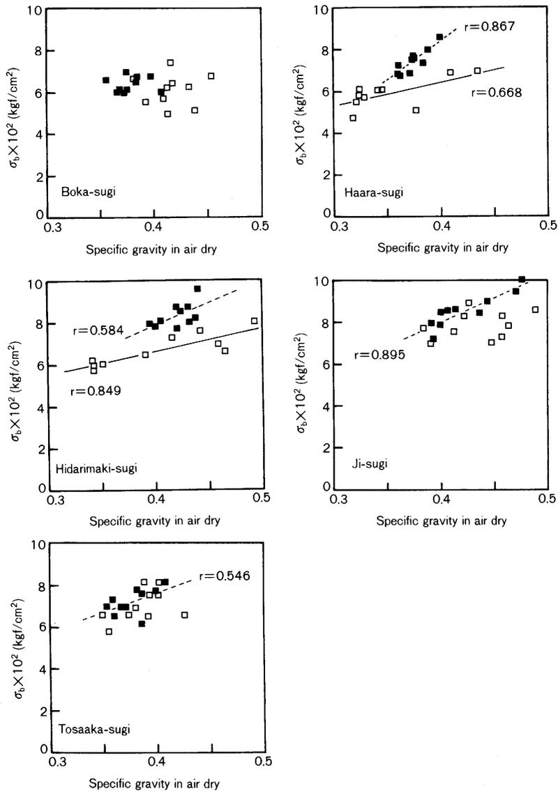
Fig. 8. Relationship between bending strength ( $\sigma_b$ ) and specific gravity in air dry.
