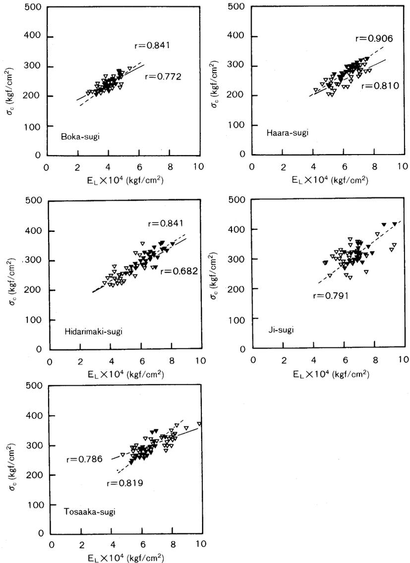
Fig. 16. Relationship between compressive strength parallel to the grain ( $\sigma_c$ ) and Young's modulus in compression parallel to the grain ( $E_L$ ).
