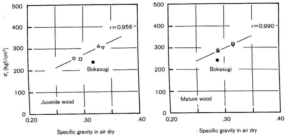
Fig. 14. Relationship between compressive strength parallel to the grain ( $\sigma_c$ ) and specific gravity in air dry of 5 sugi cultivars.
