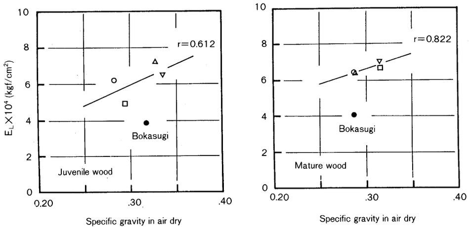
Fig. 13. Relationship between Young's modulus in compression parallel to the grain ( $E_L$ ) and specific gravity in air dry of 5 sugi-cultivars. Boka-sugi is not included in the calculation of regression line.
