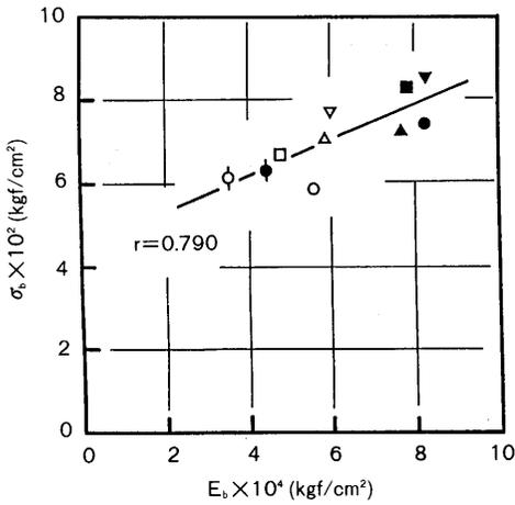
Fig. 17. Relationship between bending strength ( $\sigma_b$ ) and Young's modulus in bending ( $E_b$ ) of 5 sugi cultivars. closed: juvenile wood, open: mature wood
