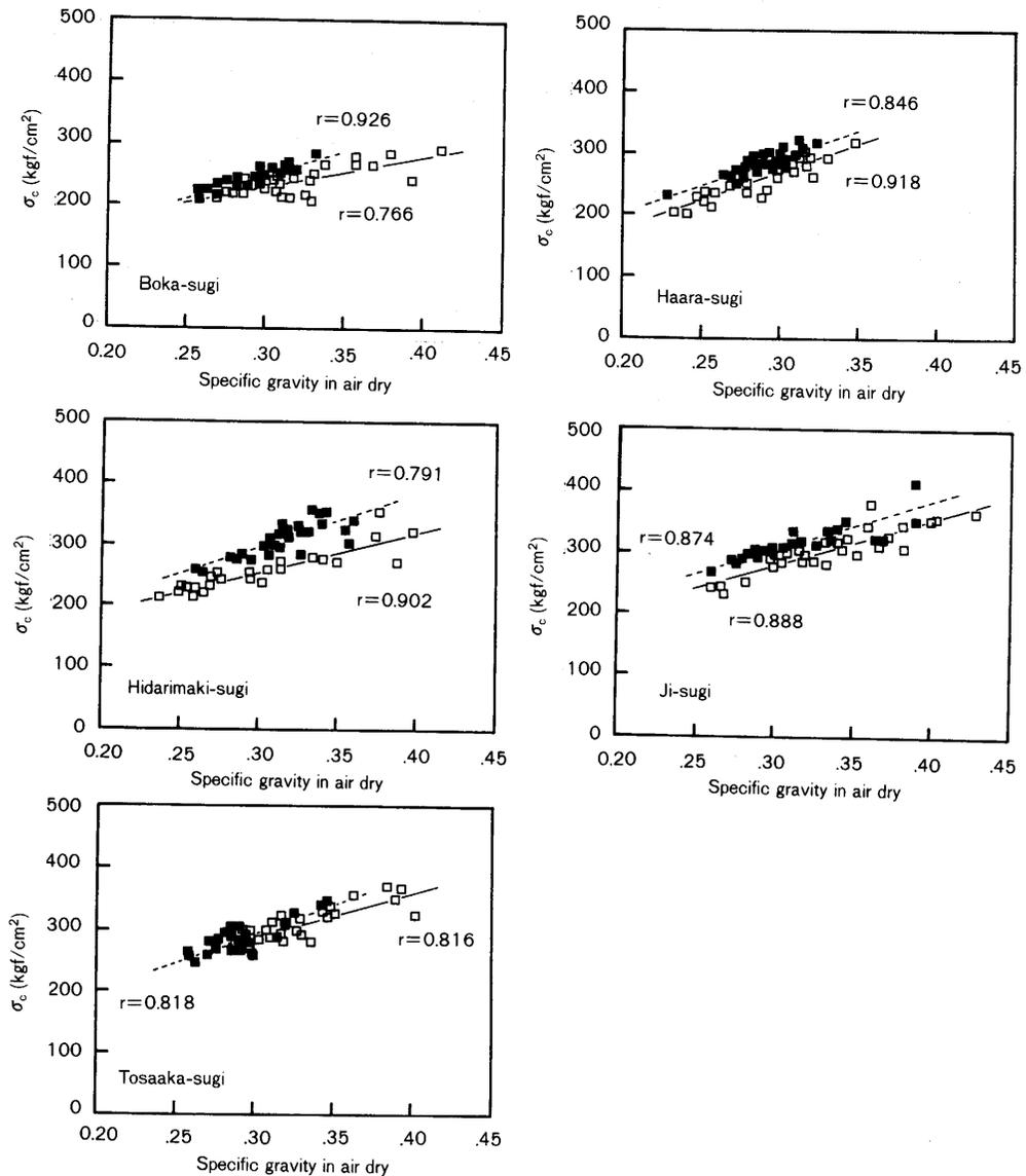
Fig. 12. Relationship between compressive strength parallel to the grain ( $\sigma_c$ ) and specific gravity in air dry.
