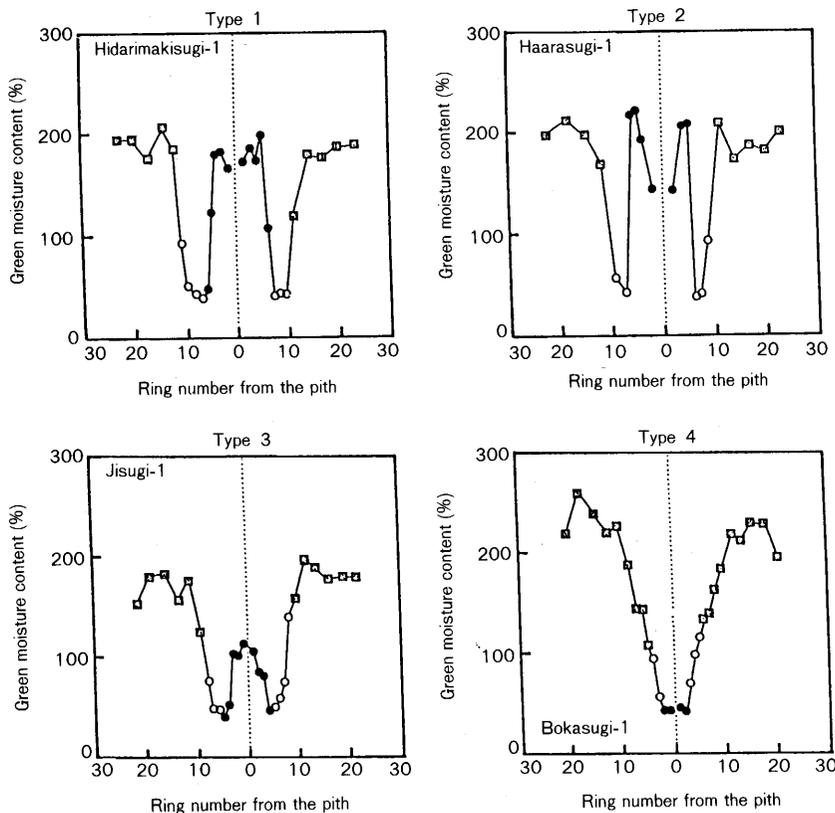
Fig. 5. Examples of radial distribution of green moisture content at the breast height. ●: heartwood, ○: white zone, □: sapwood
