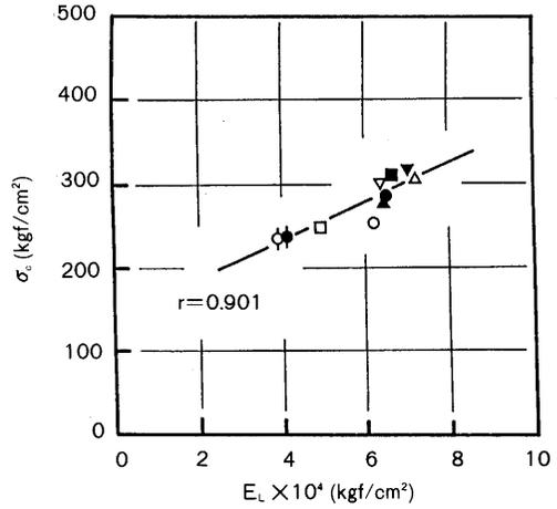
Fig. 18. Relationship between compressive strength parallel to the grain ( $\sigma_c$ ) and Young's modulus in compression parallel to the grain ( $E_L$ ) of 5 sugi-cultivars. closed: juvenile wood, open: mature wood
