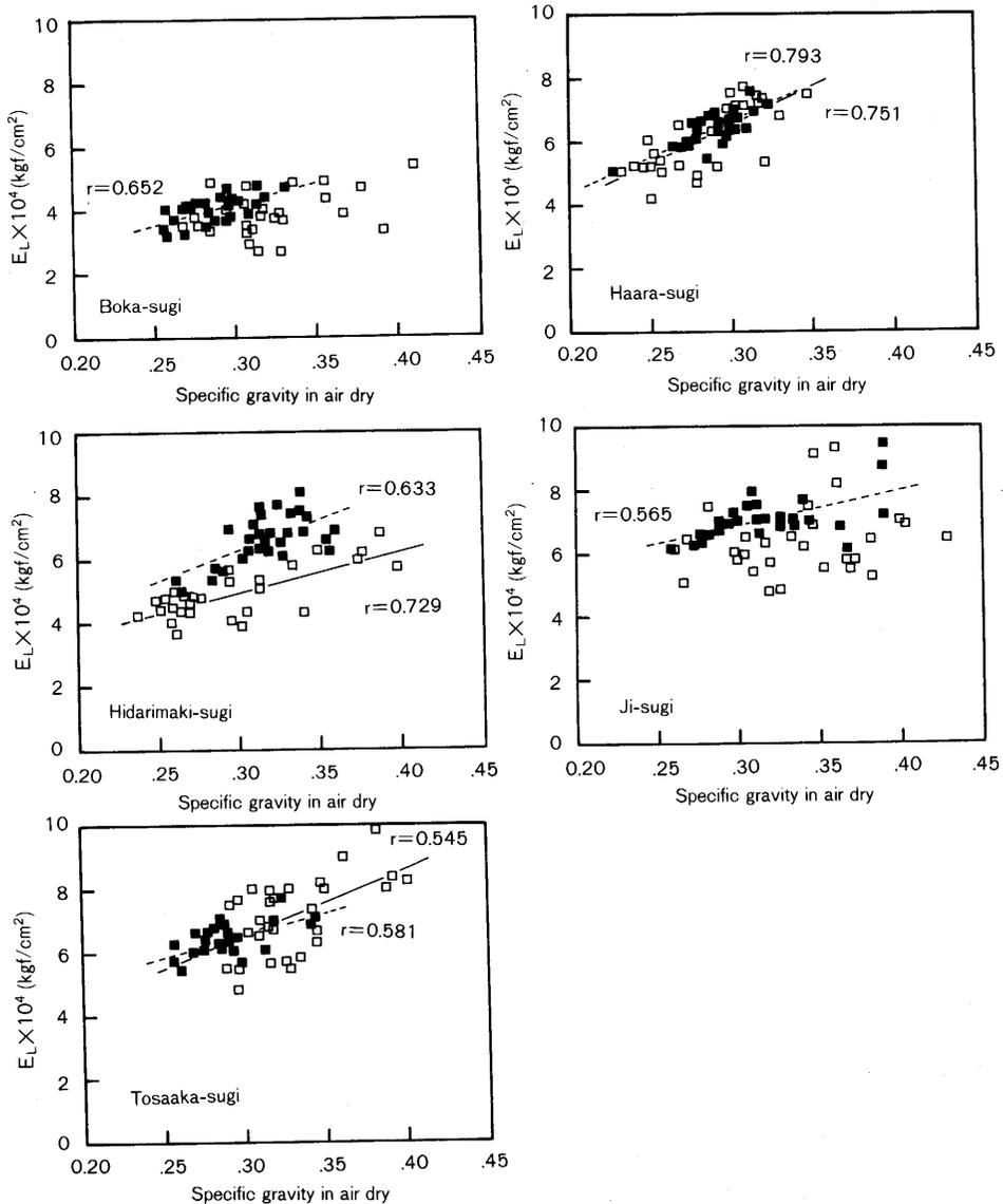
Fig. 11. Relationship between Young's modulus in compression parallel to the grain ( $E_L$ ) and specific gravity in air dry.
