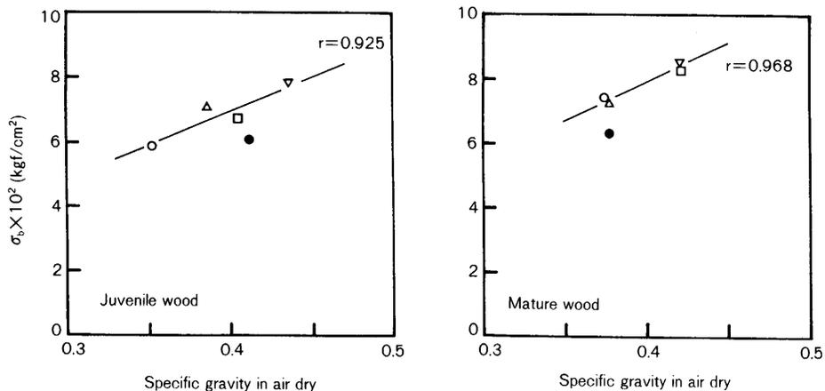
Fig. 10. Relationship between bending strength ( $\sigma_b$ ) and specific gravity in air dry of 5 sugi-cultivars. Boka-sugi is not included in the calculation of regression line.
