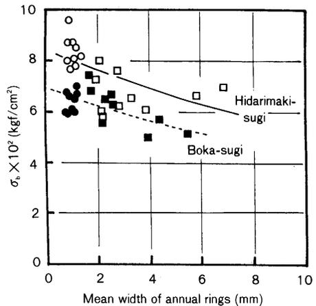
Fig. 20. Relationship between bending strength ( $\sigma_b$ ) and mean width of annual rings. squares: juvenile wood, circles: mature wood
