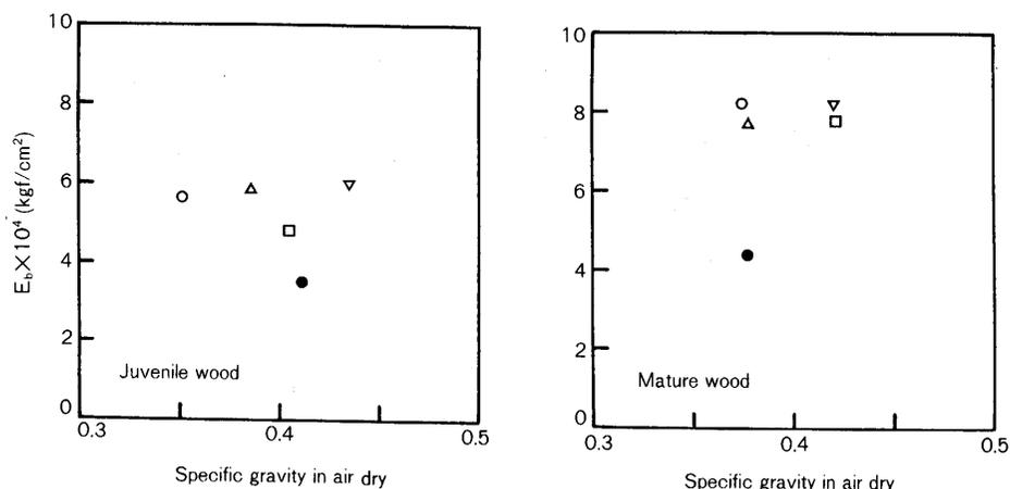
Fig. 9. Relationship between Young's modulus in bending ( $E_b$ ) and specific gravity in air dry of 5 sugi-cultivars.
