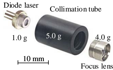
Figure 3.4: Picture of the diode laser optical system: diode laser, collimation tube, and focusing lens.
