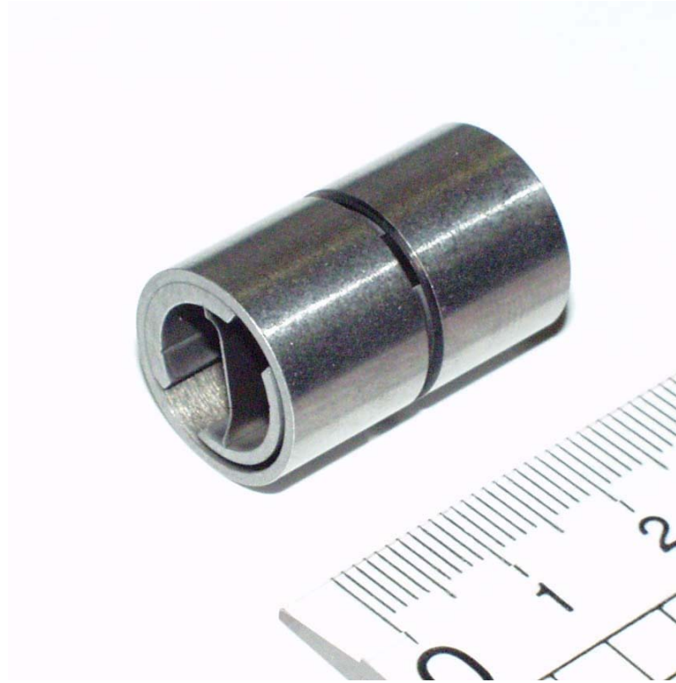
Figure 2.2: Photograph of a flexural pivot with the rotational spring constant of 0.191 \text{ Nm/rad} .
