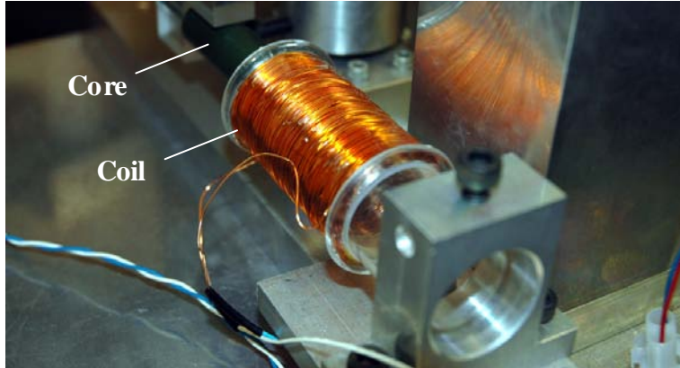
Figure 2.5: Picture of the magnetic damper.
