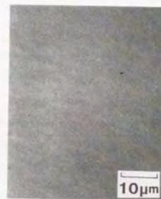
FIG. 2.7. Nomarski microphotograph of surface of a Cl-doped ZnSe layer with  $n_{300\text{K}} = 5.2 \times 10^{17} \text{ cm}^{-3}$ .
