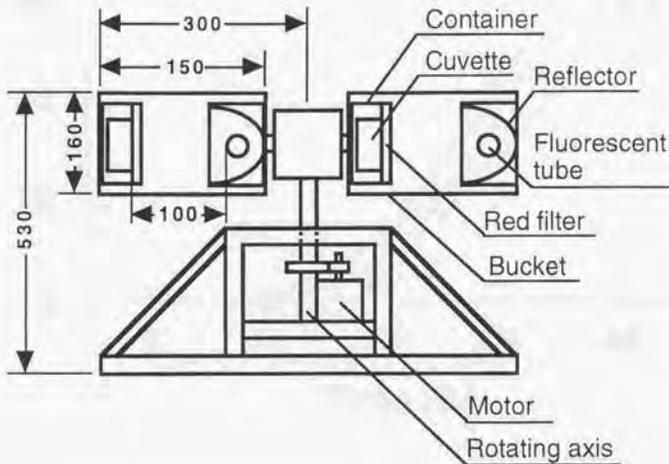
**Fig. 2** The centrifugation equipment. The electric power for the light source for each bucket was supplied via the rotating axis. At maximum rotation (260 rpm), the protonemata were exposed to basipetal hypergravity at  $20 \times g$  (Basi- $20 \times g$ ) or acropetal hypergravity at  $13 \times g$  (Acro- $13 \times g$ ). Numbers refer to distances in mm.
