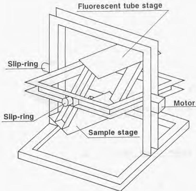
**Fig. 2** The three-dimensional clinostat. The centrifugal force ( $F$ ) which is generated by rotation of samples on the clinostat is calculated by the formula indicated below:
