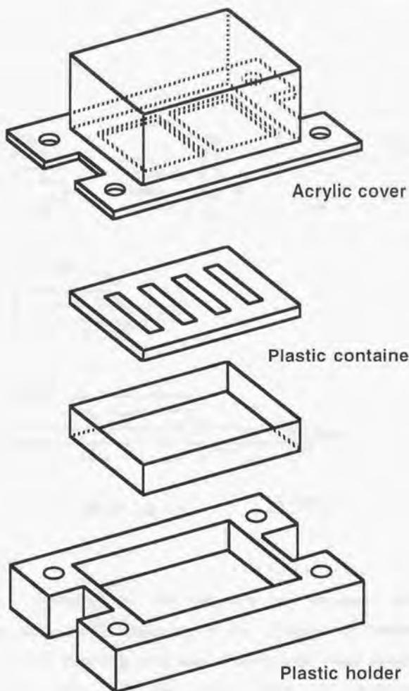
**Fig. 1** The attachment for the centrifugation system. A plastic container was stuffed with rock wool and filled with agar medium. Assembled attachment was bolted to the bucket and centrifuged. White light was irradiated from above in this figure.
