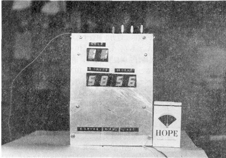
Fig. 6. Digital crystal clock with liquid crystal display.
