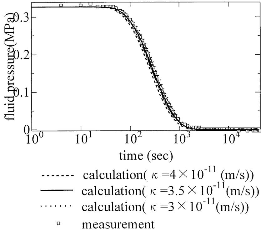
Fig. 6. Comparison of calculated and measured fluid pressures at the bottom of the sample.
