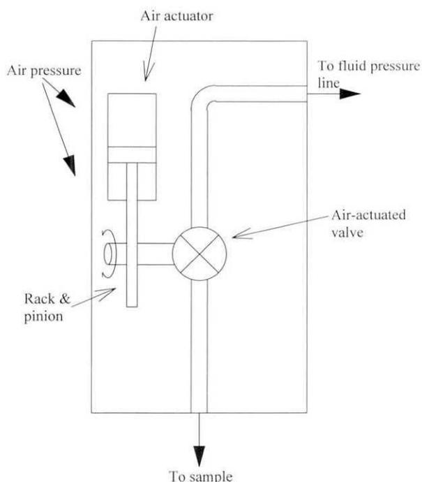
Fig. 1. Schematic figure of the newly developed endplug with built-in valve.
