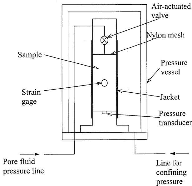
Fig. 3. Schematic figure of the experimental system.
