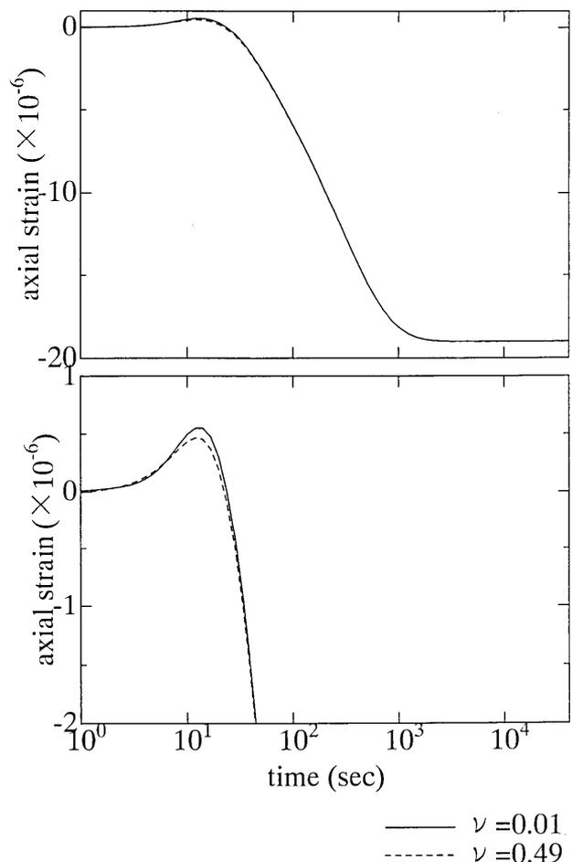
Fig. 5. Calculated axial strains during the pore pressure diffusion process. Note that the drained Poisson's ratio is not sensitive to strains.
