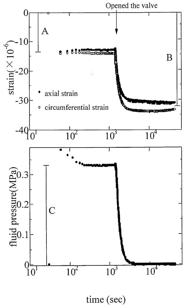
Fig. 4. Strains and fluid pressure data obtained. Note that extension is positive for strains.
