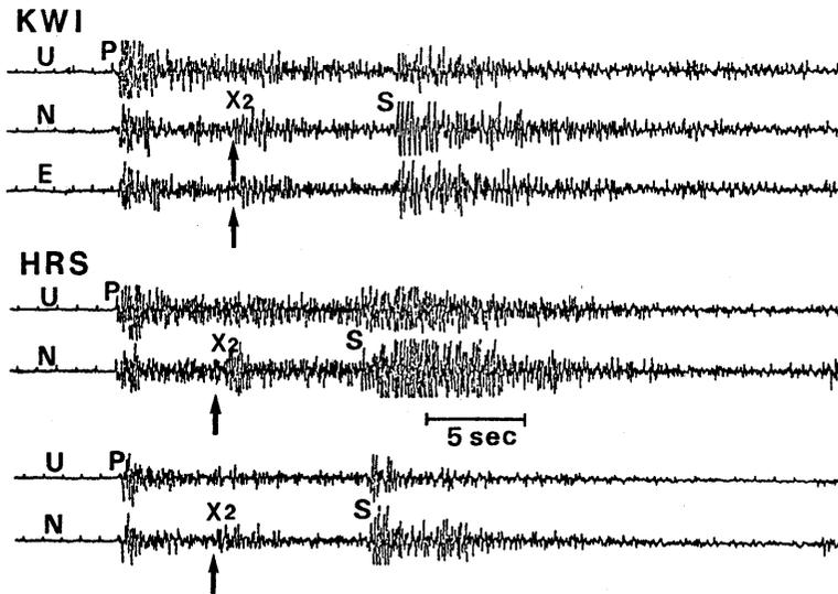
Fig. 6. Examples of the later phase  $X_2$ . This phase is prominent on the horizontal components. N and E are horizontal components in the north-south and east-west directions, respectively, and U is the vertical component.
