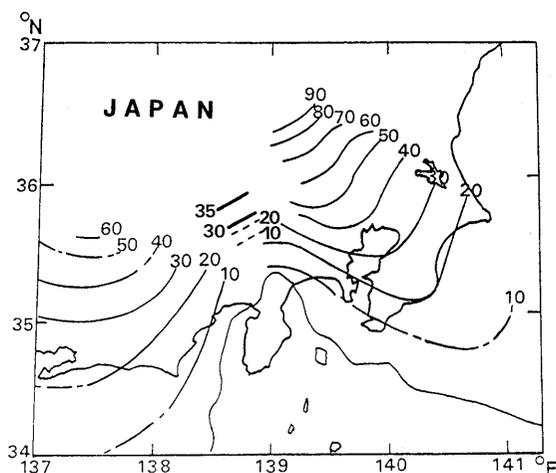
Fig. 12. Iso-depth lines of the upper boundary of the subducting Philippine Sea plate obtained using P-S converted wave data are denoted by two thick lines. The iso-depth lines obtained using S-P converted wave data (IIDA *et al.*, 1990) are shown by broken lines. Thin contour lines show results obtained by ISHIDA (1991).
