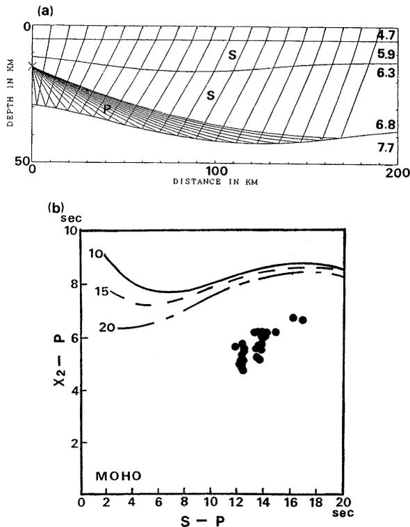
Fig. 9. (a), Ray paths of P to S converted waves at the Moho boundary are shown. Numbers indicate P-wave velocity in each layer; (b), The X-P time graph. The observed  $X_2$ -P data are denoted by solid circles. Theoretical X-P time data for a P-S converted wave at the Moho boundary are shown by lines. Three theoretical lines of the focal depths of 10, 15, and 20 km are shown by solid, broken, and dash-dotted lines, respectively.
