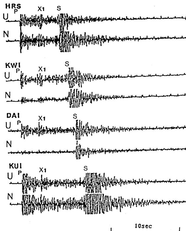
Fig. 4. Examples of the later phase  $X_1$ . This phase is prominent on the vertical component. The  $X_1$ -phase was investigated in detail by IIDAKA *et al.* (1990). U is the vertical component and N is the horizontal component in the north-south direction.
