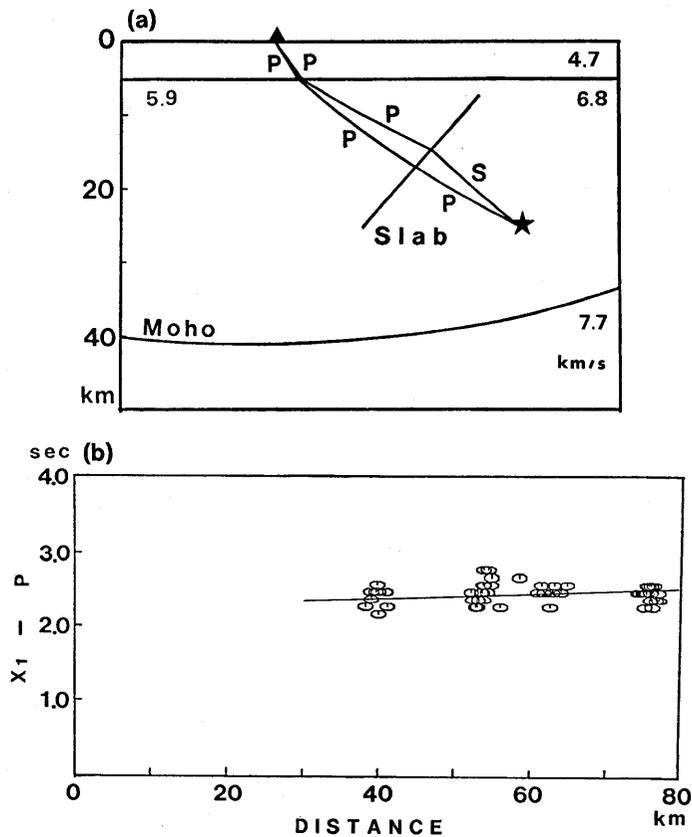
Fig. 5. (a), Schematic representation for the ray paths of direct P- and S-converted P waves. The star and triangle denote the hypocenter and station, respectively; (b), Calculated times (solid line) for an S-converted P wave at the upper boundary of the subducting Philippine Sea plate versus epicentral distance when the depth of the hypocenter is 25 km. Observed  $X_1$ -P times are shown by open circles.
