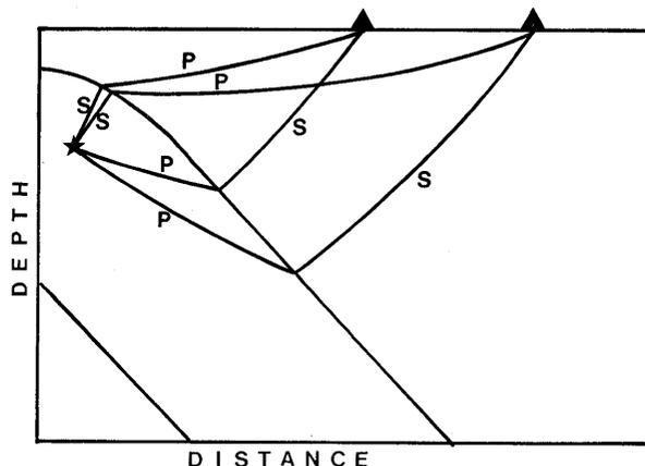
Fig. 1. Differences in the ray paths of S to P and P to S converted waves are shown schematically.
