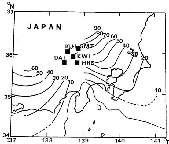
Fig. 2. Map of five seismic stations (squares) located in the western Kanto region. Iso-depth lines of the upper boundary of the Philippine Sea plate inferred from the seismicity after ISHIDA (1991) are shown in km.
