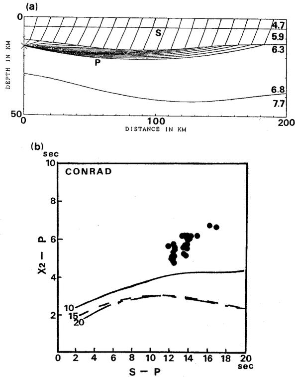
Fig. 8. (a), Ray paths of P to S converted waves at the Conrad boundary. P-wave velocity in each layer is given in km/s; (b), The X-P time graph. The observed  $X_2$ -P data are denoted by solid circles. Theoretical X-P time data for a P-S converted wave at the Conrad boundary are shown by lines. Three theoretical lines of the focal depths of 10, 15, and 20 km are shown by solid, broken, and dash-dotted lines, respectively.
