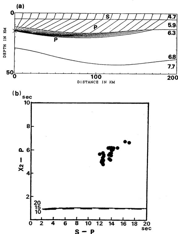
Fig. 10. (a), Ray paths of P to S converted waves at the sedimentary layers are shown. Numbers indicate P-wave velocity in each layer; (b), The X<sub>2</sub>-P time graph. The observed X<sub>2</sub>-P data are denoted by solid circles. Theoretical X-P time data for a P-S converted wave at the sedimentary layer boundary are shown by lines. Three theoretical lines of the focal depths of 10, 15, and 20 km are shown by solid, broken, and dash-dotted lines, respectively.
