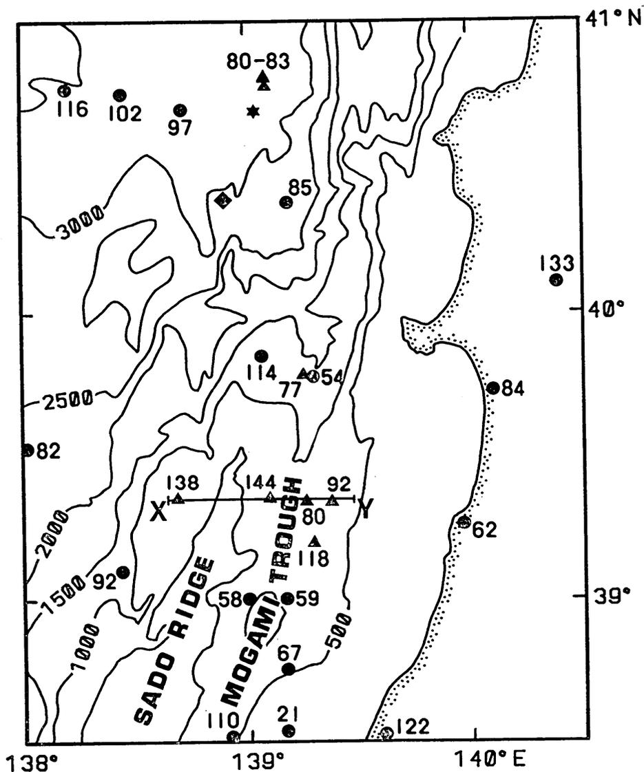
Fig. V-5. Heat flow data in the eastern margin area of the Japan Sea (in  $\text{mW/m}^2$ ). Contour interval is 500 m. Circles represent previous measurements (YOSHII, 1979; unpublished data by Honda and Lamont-Doherty Geological Observatory) and triangles are results of this study. Star is the location of an anomalous reflector (Fig. V-7). Rhombus is the epicenter of the 1983 Nihonkai-Chubu Earthquake.
