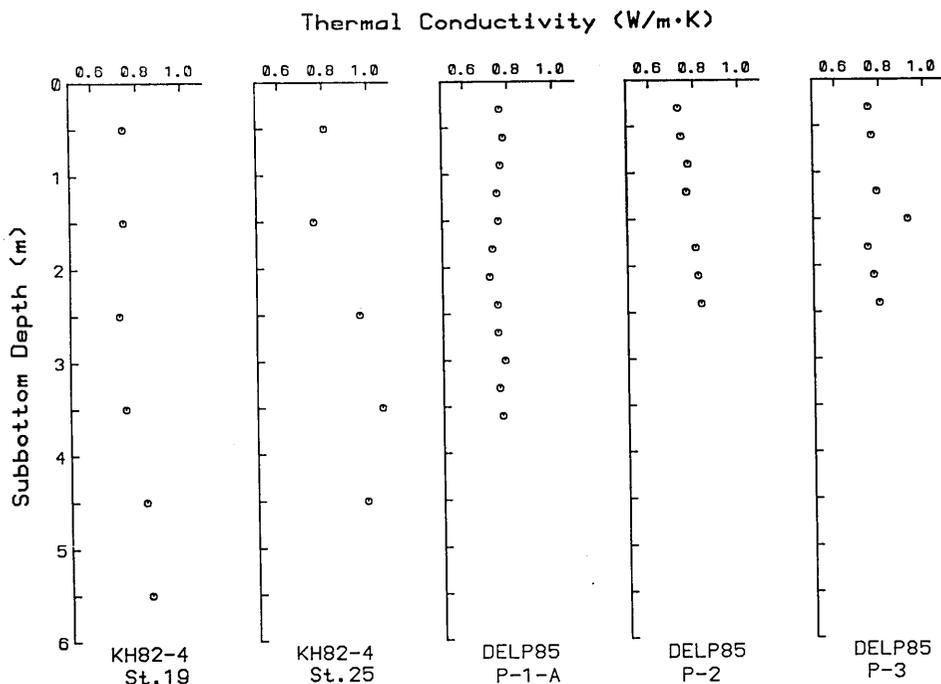
Fig. V-3. Thermal conductivity versus depth measured on piston core samples.
