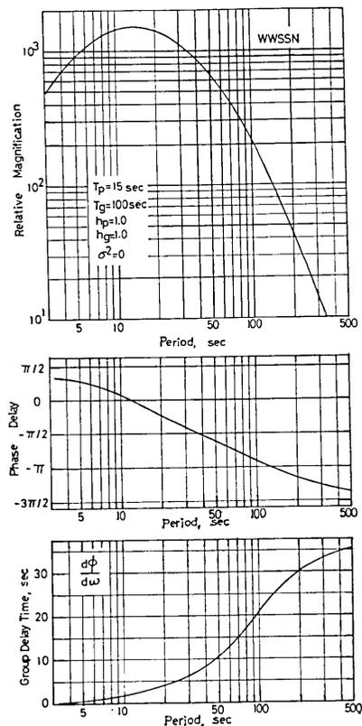
Fig. 10. Instrumental response of the WWSSN long-period seismograph: relative magnification, phase delay, and group delay time.  $T_p$  and  $h_p$  are the natural period and damping constant of the pendulum, respectively.  $T_g$  and  $h_g$  are those of the galvanometer.  $\sigma$  is the coupling factor between the seismometer and the galvanometer.
