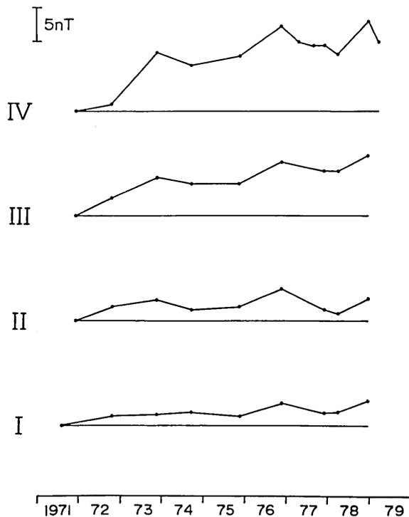
Fig. 7. Secular changes of total intensity averaged within each survey area.
