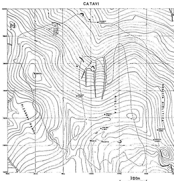
Fig. 10. Locations of temperature measurements in the Catavi mine. (local coordinates).
