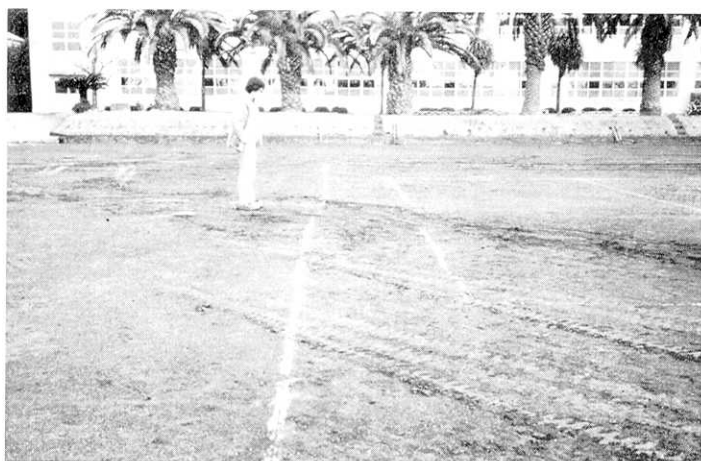
Fig. 3. En-échelon ground cracks and offset white lines on the playground of Inatori Junior High School (Loc. C-2).
