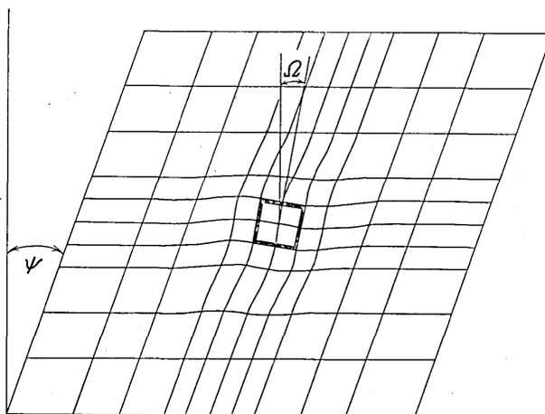
Fig. 8. Deformation in vicinity of rigid instrument base. Lines represent X-Y grid prior to deformation. Angle of shear  $\Psi = (\partial u / \partial y + \partial v / \partial x)$ . Instrument base rotates an amount  $\Omega = 1/2(\partial u / \partial y - \partial v / \partial x)$ .
