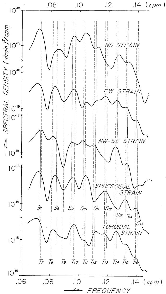
Fig. 3. Spectrum of Alaskan earthquake recorded at Nokogiriyama. Upper traces are for individual strain components and lower traces are separated spheroidal and toroidal spectra.
