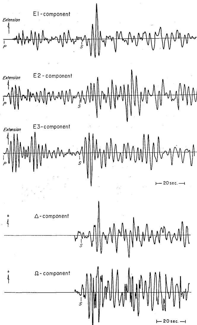
Fig. 6. Seismograms of deep earthquake in Japan Sea recorded at Yahiko. Upper traces are original strain seismograms and lower traces are separated SV and SH seismograms.
