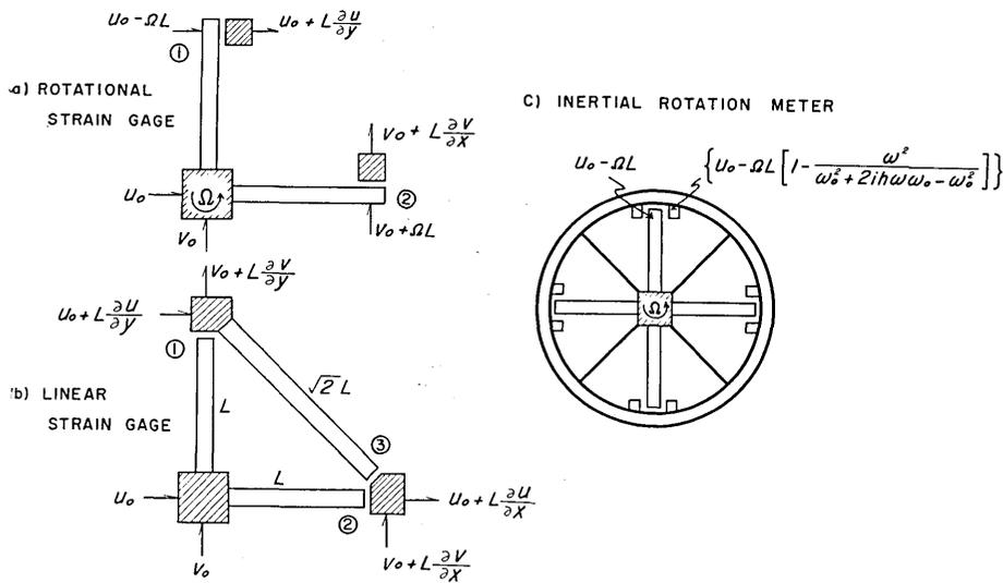
Fig. 7. a) Rotational strain gage. Sum of outputs at transducers (1) and (2) is proportional to rotation  $\Omega$  at all frequencies.
