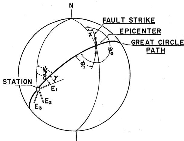
Fig. 1. Geometry and definition of source coordinates. Note that epicentral distance and direction of a nodal line of the source must be known to define source coordinates.
