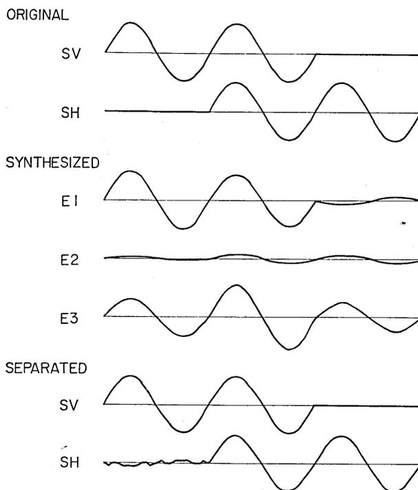
Fig. 5. Synthetic data for test of plane wave separation process. Direction parameters are assumed the same as for actual data shown in Fig. 6.
