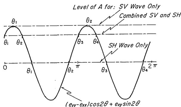
Fig. 4. Solutions to Equation 12 showing possible angles of approach  $\theta_i$ . Note that in case of a pure SV wave the ambiguity in direction of approach  $\theta_2 - \theta_1$  is  $180^\circ$ , and in the case of an SH wave the ambiguity is  $90^\circ$ . Intermediate values are also possible for a combined wave.
