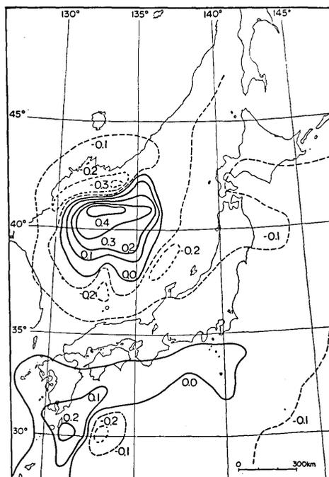
Fig. 5. The  $\Delta Z/\Delta H$  value distribution as caused by the induced currents which are distorted by Japan Islands.
