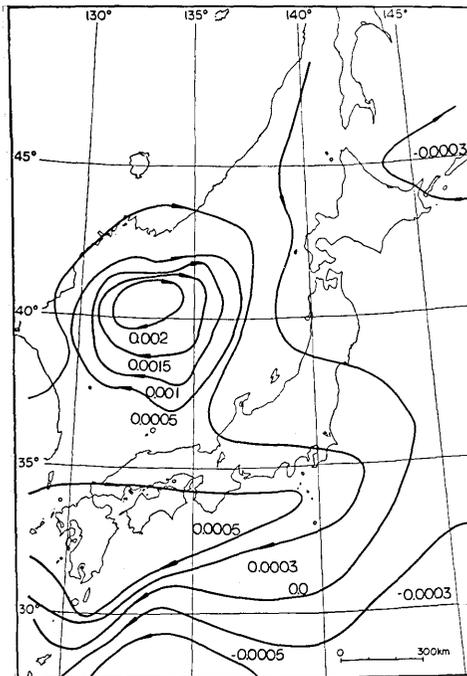
Fig. 3a. The additional current function distribution as caused by the conductivity irregularity representing Japan Islands. The unit is chosen so as to make the uniform inducing field unity.
