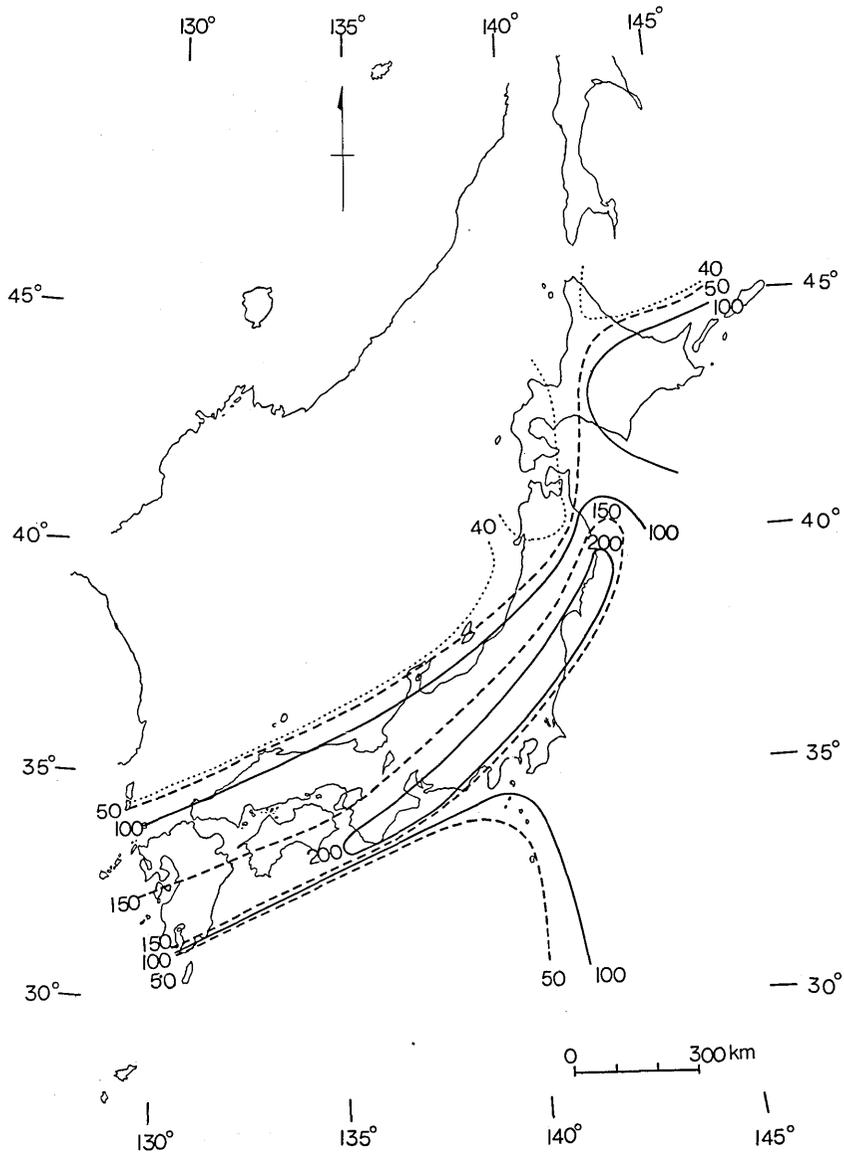
Fig. 6. Depths of mantle conducting layer in units of km underneath Japan Islands.
