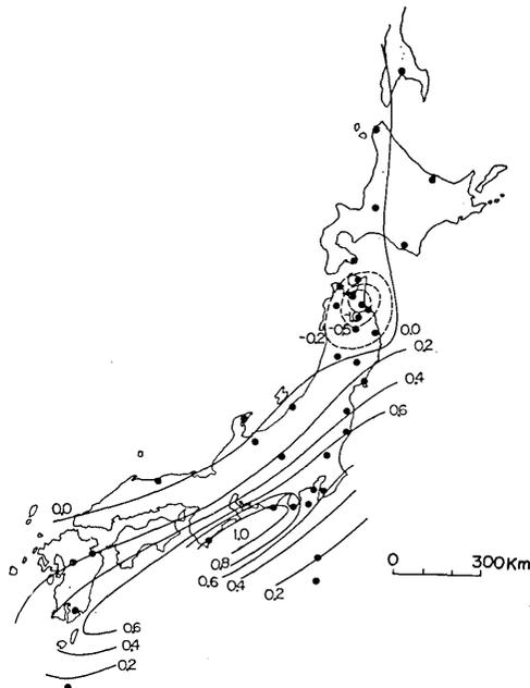
Fig. 1. The  $\Delta Z/\Delta H$  value distribution for geomagnetic bays and similar changes.
