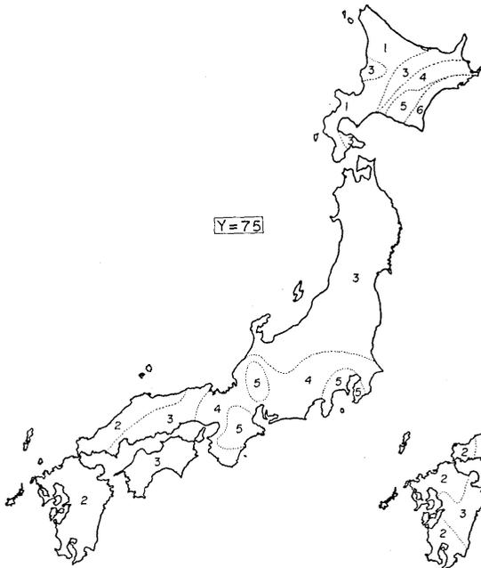
Fig. 2. Expectancy of the maximum velocity amplitude of earthquake motions at bed rock in 75 years.
