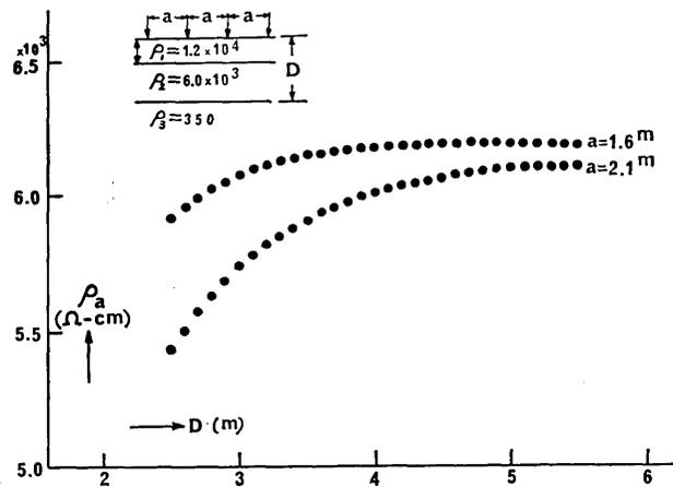
Fig. 10. Expected changes in the  $\rho_a$  (apparent resistivity) when the depth of the third layer changes as calculated for the two values of electrode distance  $a$ .
