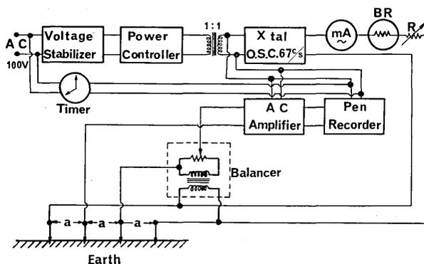
Fig. 2. Schematic diagram of the apparent resistivity observation by the four electrode method.
