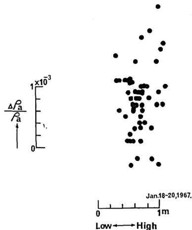
Fig. 8.  $\Delta\rho_a/\rho_a$  versus sea level relation as plotted using the hourly readings.
