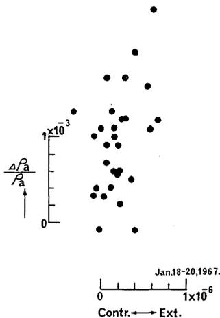
Fig. 7.  $\Delta\rho_a/\rho_a$  versus earth strain relation as plotted using the data read every two hours.
