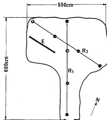
Fig. 5. Electrode arrangements in the cave. An electronic extensometer E is set parallel to the  $R_3$  arrangement.
