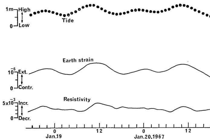
Fig. 6. Simultaneous records of the apparent resistivity, the earth strain and the sea level.
