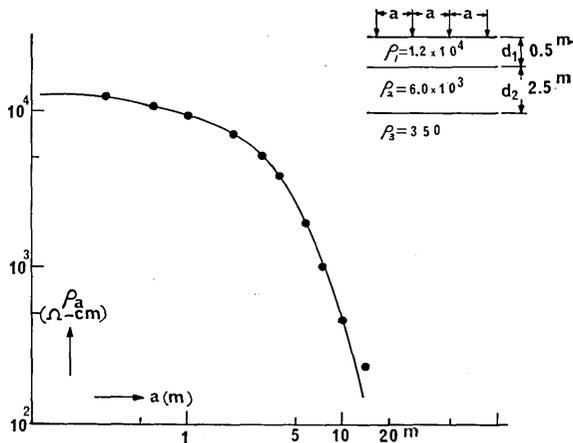
Fig. 9. Changes in  $\rho_a$  (apparent resistivity) with  $a$  (electrode distance) as revealed by the electric prospecting in the N 60°E direction.
