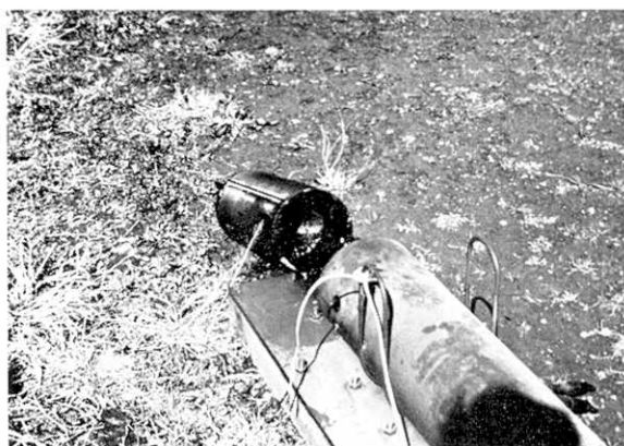
Fig. 2b. Close-up view of the powder chamber of the generator.
