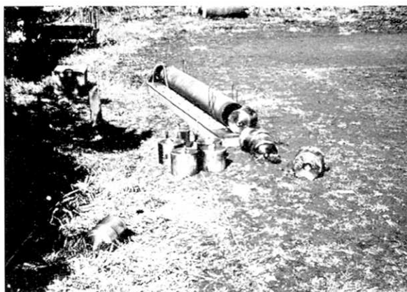
Fig. 2a. General view of Mark I SH-wave generator. Iron weights are seen outside the pipe.
