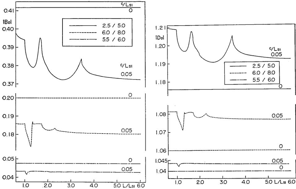
Fig. 2. Reflection ( $B_0$ ) and refraction ( $D_0$ ) coefficients of regular waves for three models in the case of normal incidence of  $SV$  waves. The abscissa is the wavelength of corrugation in units of the wavelength of the incident  $SV$  wave.
