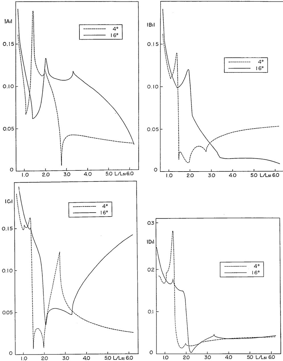
Fig. 8. Reflection and refraction coefficients of forward irregular waves in the case of the oblique incidence of *SV* waves.  $A_1$  is the reflection coefficient for forward irregular *P* waves;  $D_1$ , the refraction coefficient for forward irregular *S* waves; and so on.
