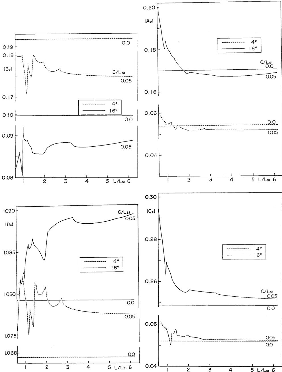
Fig. 6. Reflection and refraction coefficients of regular waves in the case of oblique incidence of  $SV$  waves.  $A_0$  is the reflection coefficient for  $P$  waves;  $D_0$  is the refraction coefficient for  $S$  waves; and so on. The abscissa is the wavelength of corrugation in units of the wavelength of the incident  $SV$  wave; the parameter is the amplitude of corrugation in units of the wavelength of the incident  $SV$  wave.
