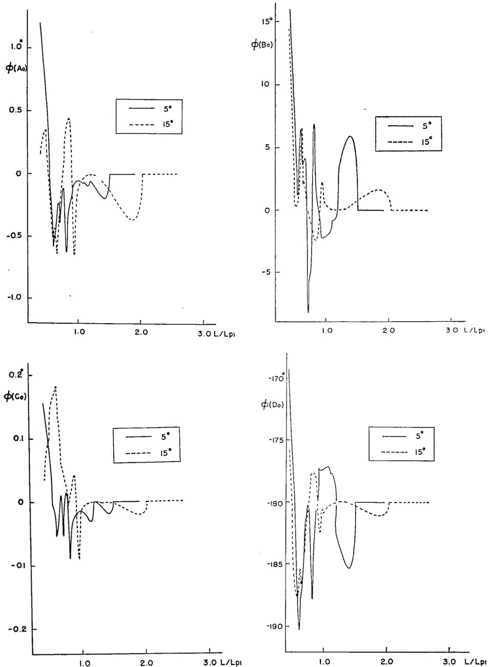
Fig. 13. Phase changes of regular waves in the case of oblique incidence of  $P$  waves. For example  $\phi(A_0)$  is the phase change of regularly reflected  $P$  waves,  $\phi(D_0)$ , that of regularly refracted  $S$  waves.  $c/L_{P1}$ , the corrugation amplitude to the wavelength of incident  $P$  wave, is put equal to 0.05.
