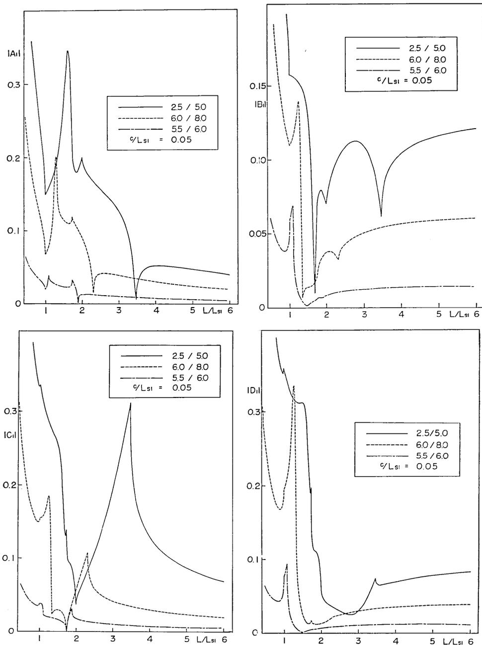
Fig. 4. Reflection and refraction coefficients of irregular waves for three models in the case of normal incidence of SV waves.
