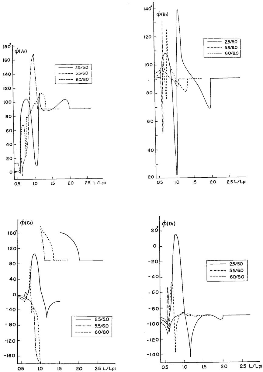
Fig. 12. Phase changes of irregular waves for three models in the case of normal incidence of  $P$  waves.  $\phi(A_1)$  is the phase change of irregularly reflected  $P$  wave;  $\phi(D_1)$ , that of irregularly refracted  $S$  wave and so on.
