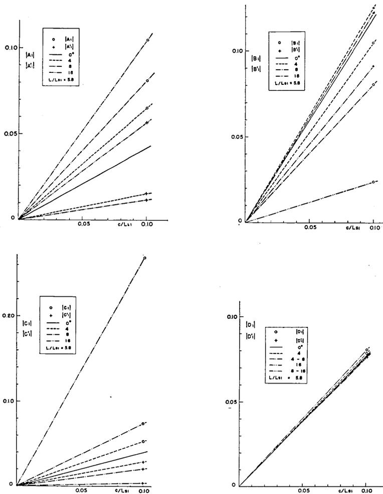
Fig. 10. Reflection and refraction coefficients of irregular waves in the case of the oblique incidence of  $SV$  waves. The abscissa is the corrugation amplitude in units of the wavelength of the incident  $SV$  wave.
