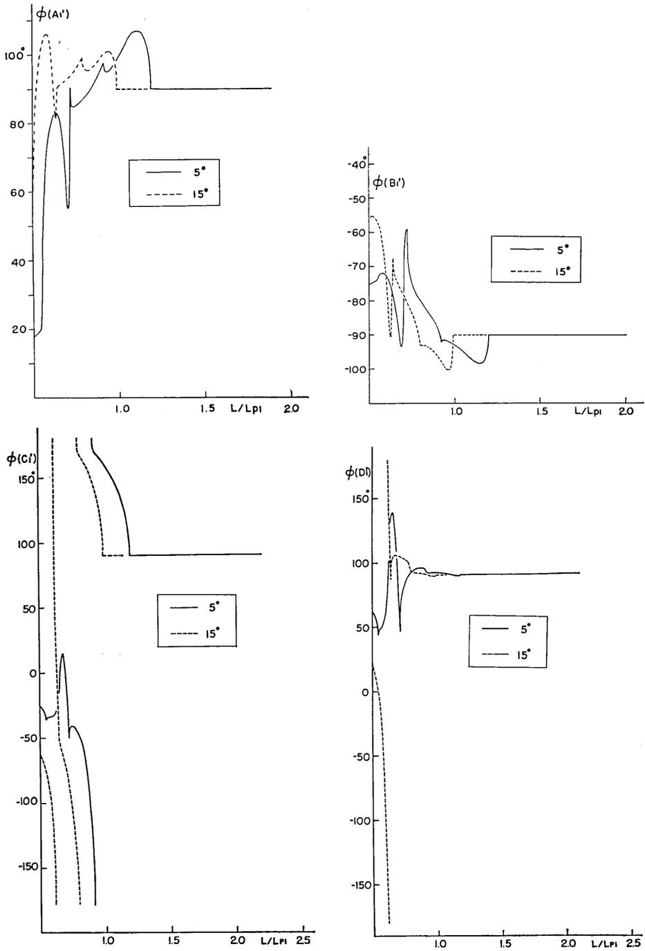
Fig. 15. Phase changes of backward irregular waves in the case of oblique incidence of  $P$  waves. For example,  $\phi(A_1')$  is the phase change of backward irregularly reflected  $P$  waves;  $\phi(D_1')$ , that of backward irregularly refracted  $S$  waves.
