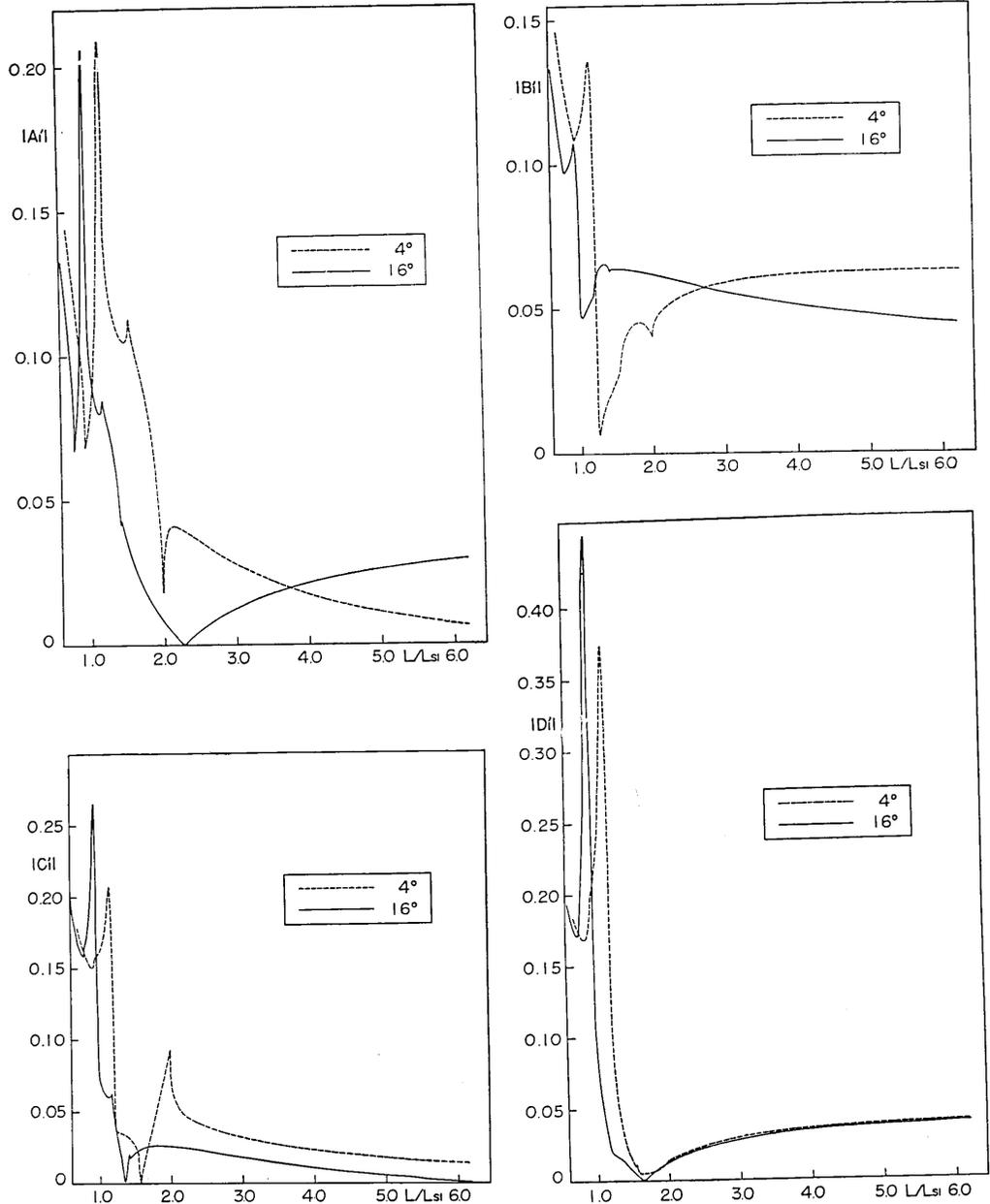
Fig. 9. Reflection and refraction coefficients of backward irregular waves in the case of the oblique incidence of  $SV$  waves.  $A_1'$  is the reflection coefficient for backward irregular  $P$  waves;  $D_1'$ , the refraction coefficient for backward irregular  $S$  waves; and so on.
