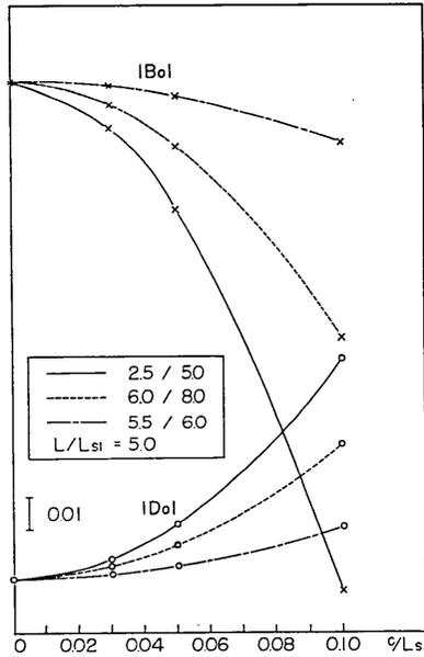
Fig. 3. Reflection and refraction coefficients of regular waves for three models in the case of normal incidence of  $SV$  waves.
