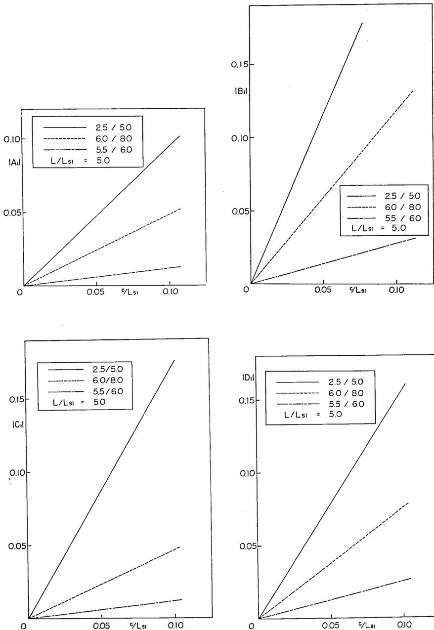
Fig. 5. Reflection and refraction coefficients of irregular waves for three models in the case of normal incidence of SV waves.
