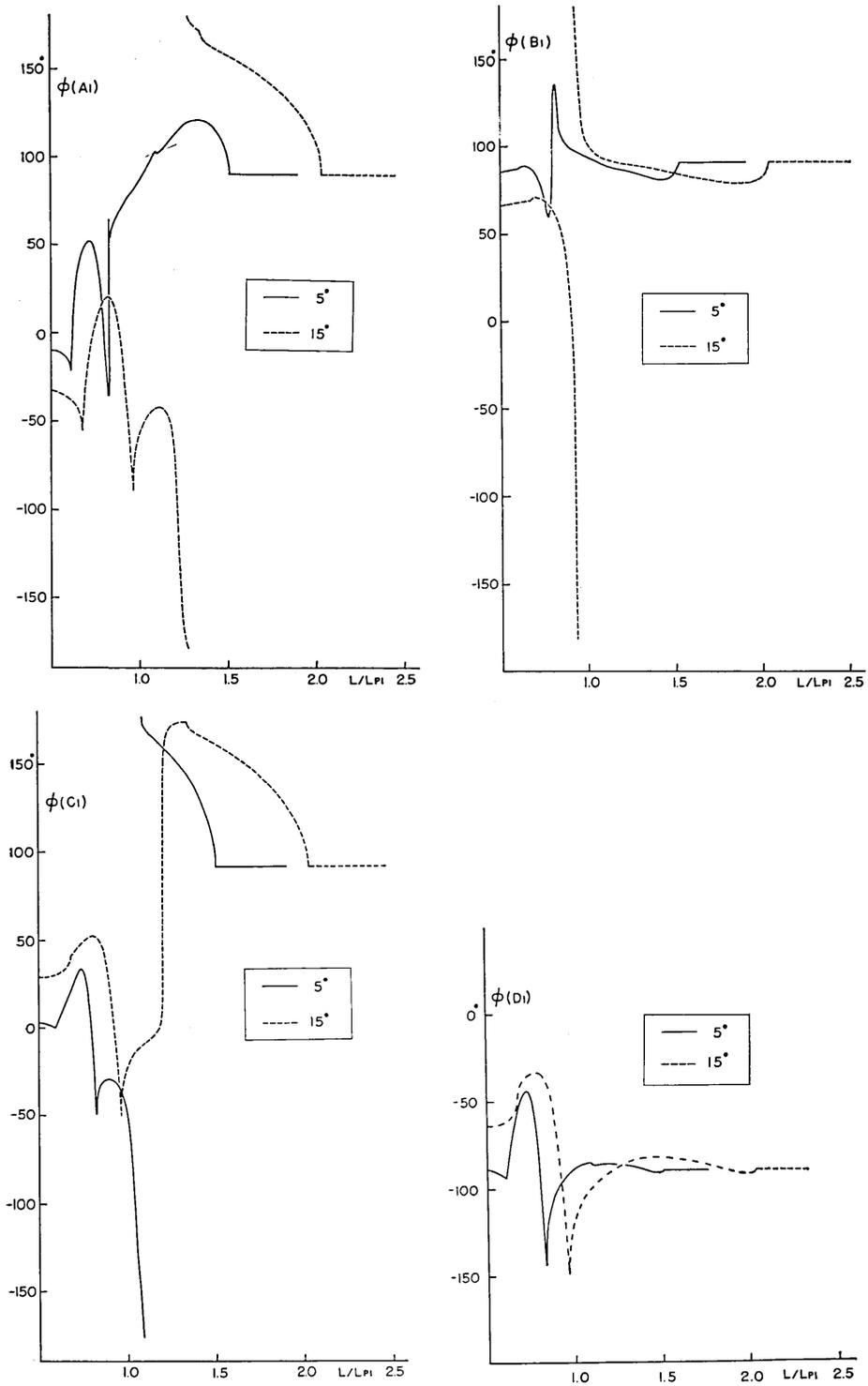
Fig. 14. Phase changes of forward irregular waves in the case of oblique incidence of  $P$  waves. For example,  $\phi(A_1)$  is the phase change of forward irregularly reflected  $P$  waves;  $\phi(D_1)$ , that of forward irregularly refracted  $S$  waves.
