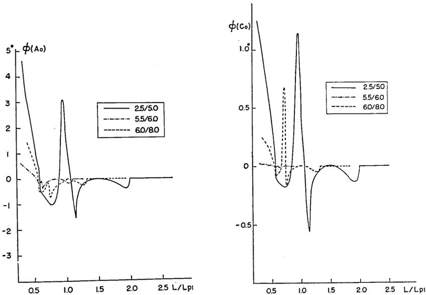
Fig. 11. Phase changes of regular waves upon reflection and refraction for three models in the case of normal incidence of  $P$  waves.  $\phi(A_0)$  stands for the phase change of regularly reflected  $P$  waves;  $\phi(C_0)$  is the phase change of regularly refracted  $P$  waves.  $c/L_{P1}$ , the corrugation amplitude to the wavelength of incident  $P$  wave, is put equal to be 0.05.
