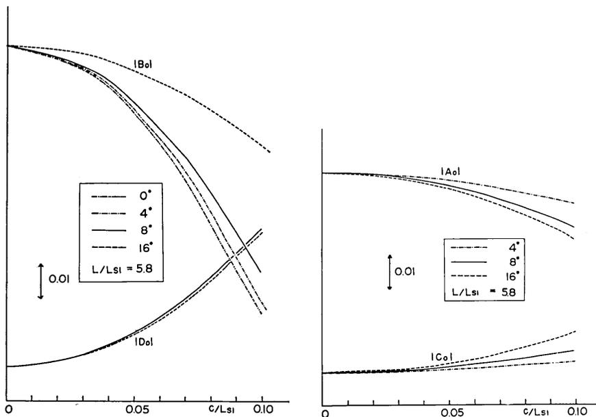
Fig. 7. Reflection and refraction coefficients of regular waves in the case of the oblique incidence of *SV* waves.  $A_0$  is the reflection coefficient for *P* waves;  $D_0$ , the refraction coefficient for *S* waves and so on. The abscissa is the amplitude of corrugation in units of the wavelength of the incident *SV* wave.
