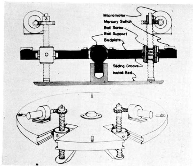
Fig. 4. Automatic levelling device.
