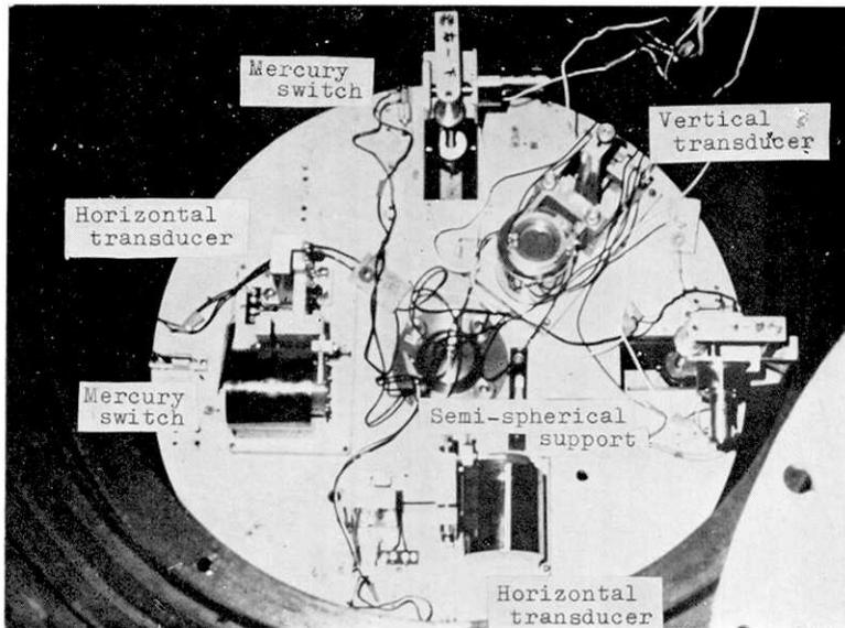
Fig. 5. Transducers on the automatic levelling plate.
