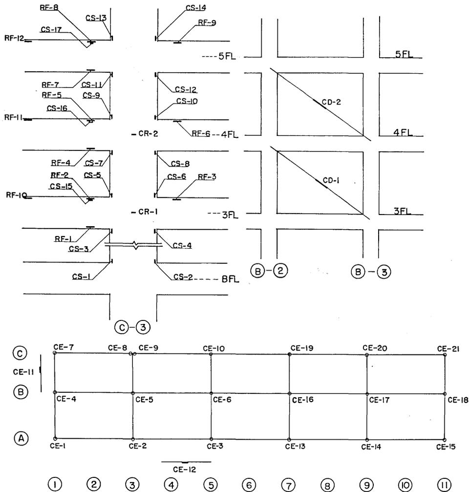
Fig. 6. Location of strain meters, etc. (2).
