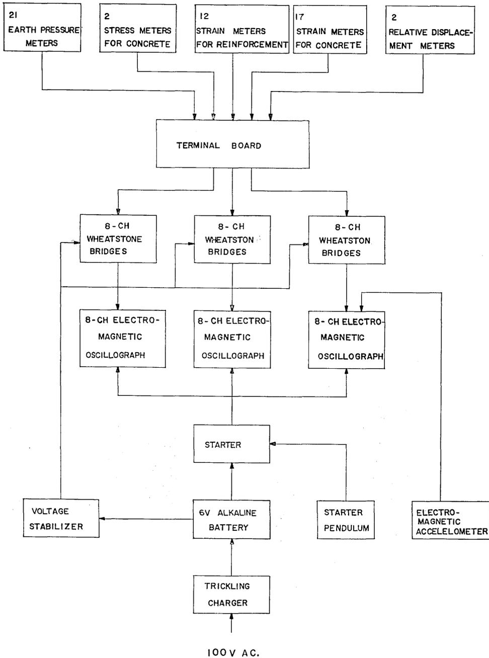
Fig. 4. Instrumentation diagram.
